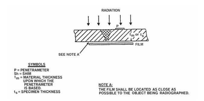
Figure 3-7. Examples of T<sub>m</sub>, T<sub>s</sub>, and Penetrameter Placement: Single Wall, No Reinforcement, No Back-Up Strip.
