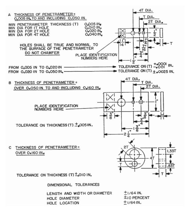
Figure 3-5. Penetrameter Designs.
