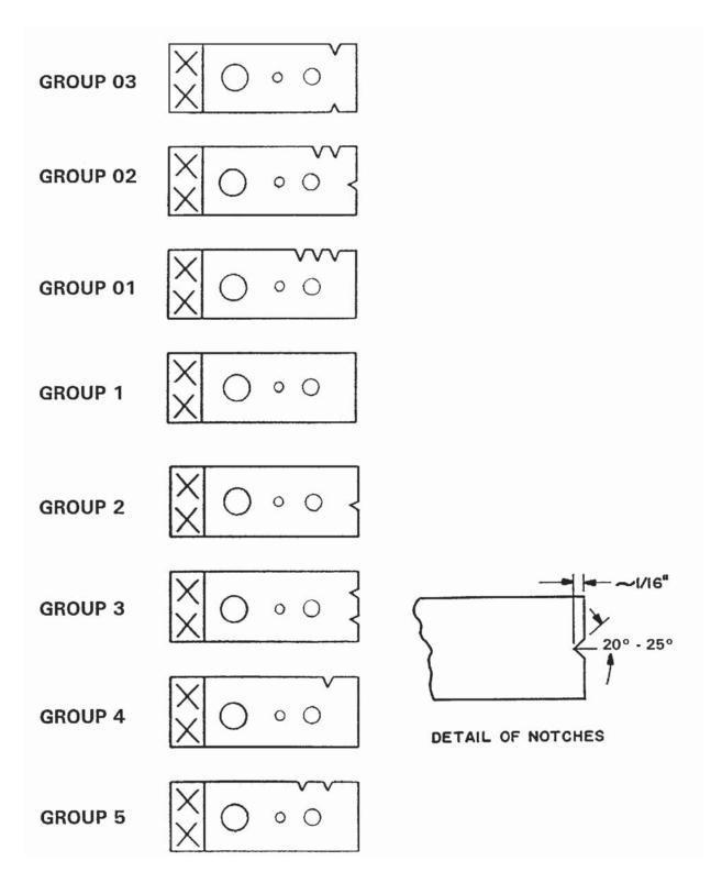
Figure 3-6. Penetrameter Identification Notching.
