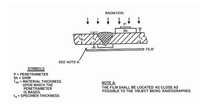
Figure 3-9. Examples of T<sub>m</sub>, T<sub>s</sub>, and Penetrameter Placement: Single Wall, Weld Reinforcement, Back-Up Strip.
