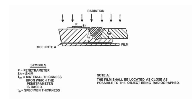
Figure 3-10. Examples of T<sub>m</sub>, T<sub>s</sub>, and Penetrameter Placement: Single Wall, Integral Backing Ring, Weld Reinforcement.
