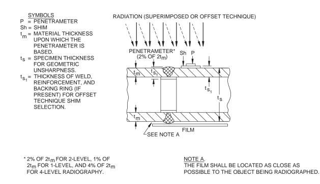
Figure 3-12. Examples of T<sub>m</sub>, T<sub>s</sub>, and Penetrameter Placement: Double Wall, Double Wall Viewing, Weld Reinforcement and Back-Up Strip.
