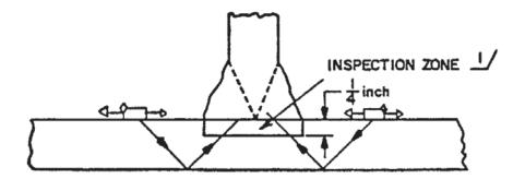
THE INSPECTION ZONE MAY BE EXPANDED AS NECESSARY WITHIN THE PLATE OR WELD. THE SAME SCANNING PROCEDURES MAY BE APPLIED TO PARTIAL PENETRATION THE WELDS.
