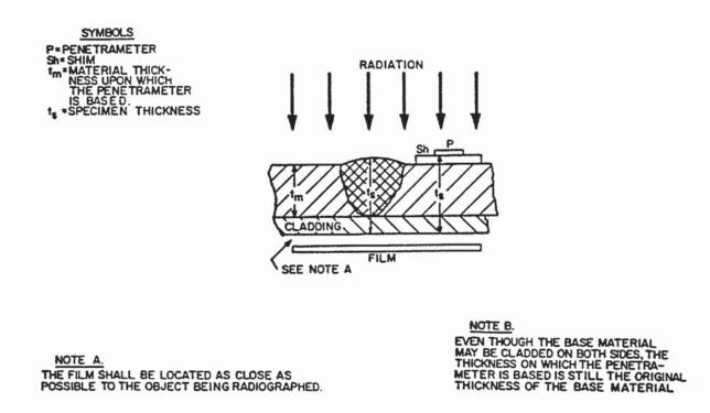
Figure 3-11. Examples of T<sub>m</sub>, T<sub>s</sub>, and Penetrameter Placement: Single Wall, Weld Reinforcement, Cladding Redeposited Over Weld in Base Metal.
