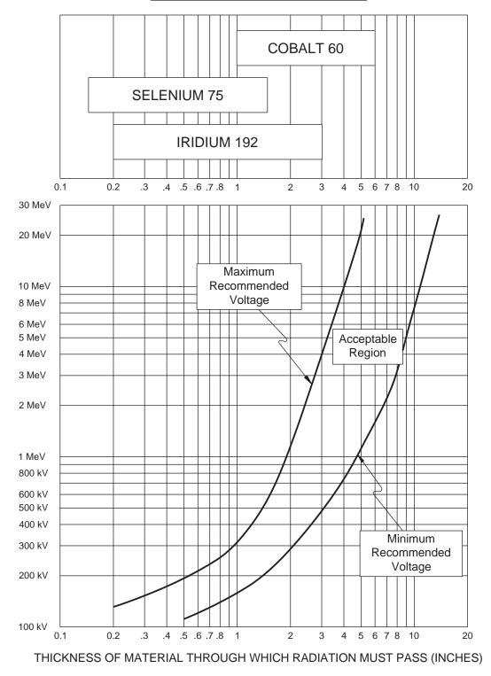
Figure 3-2. Recommended X-ray Voltage Settings and Radioisotope Sources to Be Used with Various Copper-Base and Similar Alloys.
