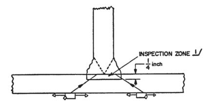
THE INSPECTION ZONE MAY BE EXPANDED AS NECESSARY WITHIN THE PLATE OR WELD. THE SAME SCANNING PROCEDURES MAY BE APPLIED TO PARTIAL PENETRATION THE WELDS.
