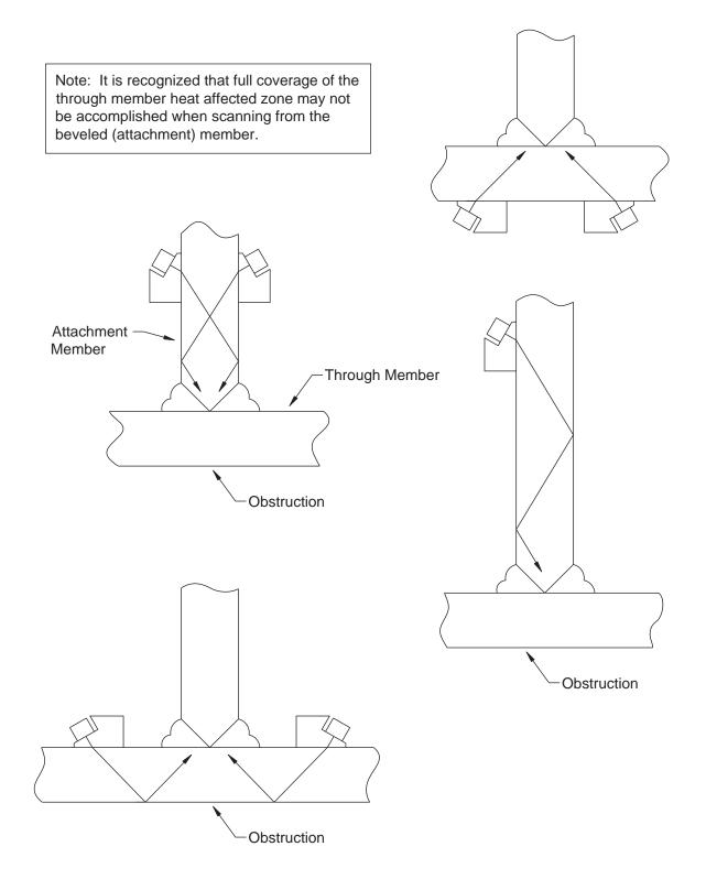
Figure 6-6. Example Scanning Techniques for Tee Welds.
