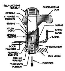
Figure 600-2.50. Quick-Acting Door Dog Assembly (Cross Section View) Modified by MACHALT 167-31004 (ECP-444)
