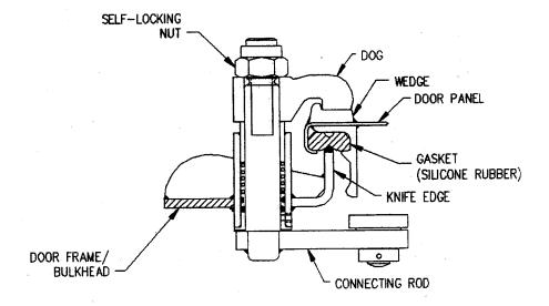
Figure 600-2.48.A. Dog With Self-locking Nut
