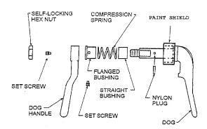
Figure 600-2.46. Steel Doors Only - Individually Dogged Door Dog Assembly (Cross Section View) Modified by MACHALT 167-31010 (ECP-526)
