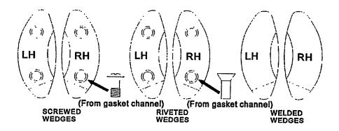
Figure 600-2.47. Watertight Door Wedges
