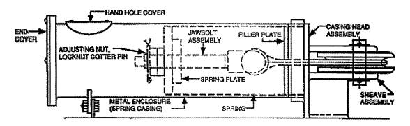
Figure 600-6.2 Spring Casing Assembly
