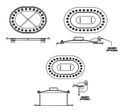
Figure 600-9.1 Watertight Manhole Cover
