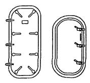
Figure 600-3.5. Armored Ballistic Closures, Tri-Hinged
