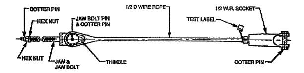
Figure 600-6.3. Cable Assembly Wire Rope
