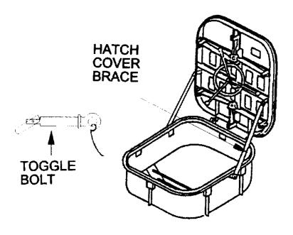
Figure 600-5.8 Hatch Cover Brace and Toggle Link
