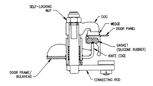
Figure 600-2.48.D Dog With Self-locking Nut
