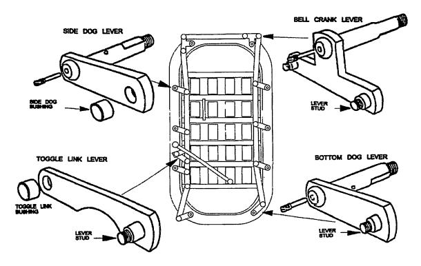
Figure 600-2.52. Quick Acting Door Levers
