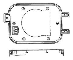
Figure 600-5.4 Flush Watertight Hatch Watertight Hatch
