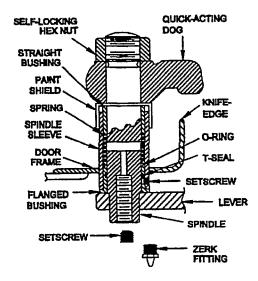
Figure 600-2.51. Quick-Acting Door Dog Assembly (Cross Section View) Modified by MACHALT 167-31010 (ECP-526)
