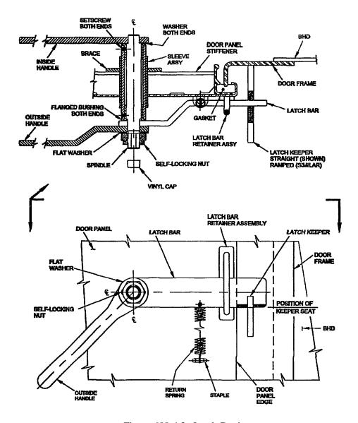
Figure 600-4.3. Latch Device
