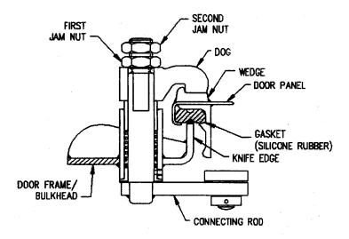
Figure 600-2.48.E Dog With Jam Nuts
