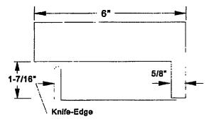
Figure 600-2.41. Gauge for Measuring Knife-edge Height
