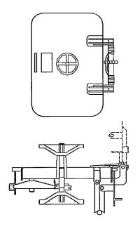
Figure 600-5.3. Raised Quick Acting Spring Balanced Hatch
