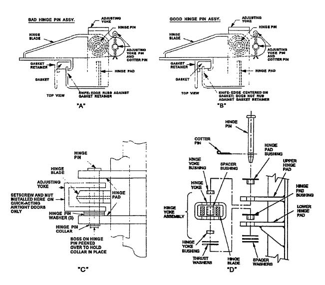
Figure 600-2.43. Hinge Pin Assemblies
