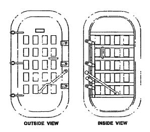
Figure 600-2.2. Quick-Acting Airtight Door
