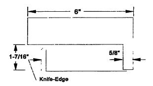
Figure 600-2.19. Gauge for Measuring Knife-edge Height
