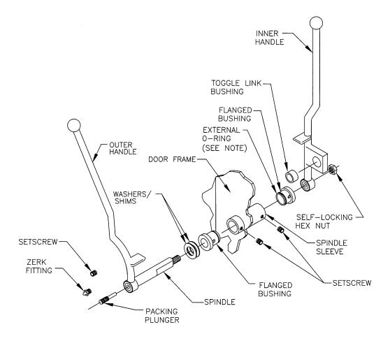
Figure 600-2.54. Quick-Acting Operating Handle Assembly (Left-Hand Shown)
