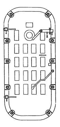
Figure 600-4.1. Door Latch Device
