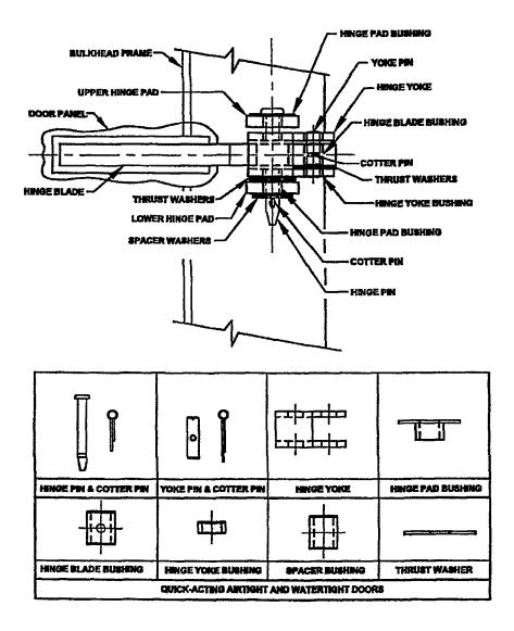
Figure 600-2.62. Watertight Door Hinge Components (For Doors With MACHALT 167-31006 (ECP-518) or MACHALT 167-31011 (ECP-538) Installed)
