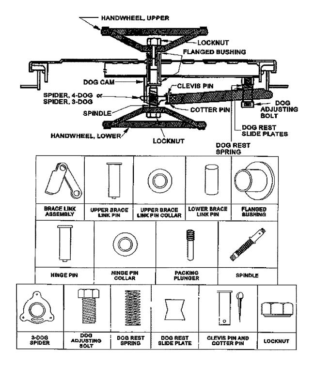
Figure 600-7.5. Raised Scuttle Components
