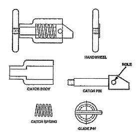
Figure 600-6.4. Automatic Catch Assembly
