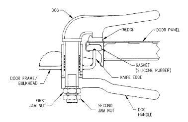
Figure 600-2.66.E. Dog With Jam Nuts
