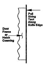
Figure 600-2.39. Knife-Edge Inspection Using String Method
