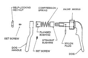
Figure 600-2.30. Individually Dogged Door Dog Assembly (Cross Section View) Modified by MACHALT 167-31010 (ECP-526)
