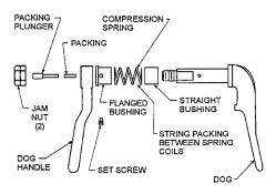
Figure 600-2.44. Individually Dogged Door Dog Assembly (Cross Sectional View)
