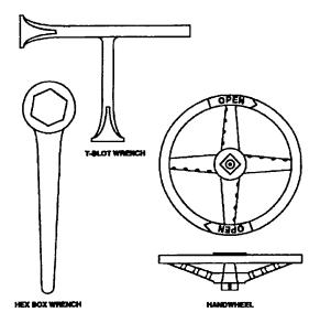
Figure 600-8.5 Handwheels and Wrenches
