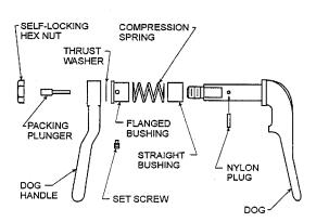
Figure 600-2.29. Individually Dogged Door Dog Lever Assembly (Cross Sectional View) Modified by MACHALT 167-31004(ECP-444)
