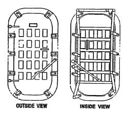
Figure 600-2.1 Quick-Acting Watertight Door
