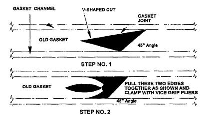
Figure 600-2.65. Gasket Removal
