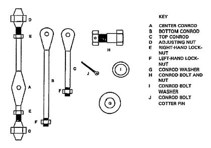
Figure 600-6.7. Turnbuckle Assembly Parts
