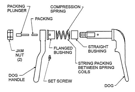
Figure 600-2.28. Individually Dogged Door Dog Assembly (Cross Sectional View)
