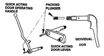
Figure 600-2.49. Packing Plunger Locations
