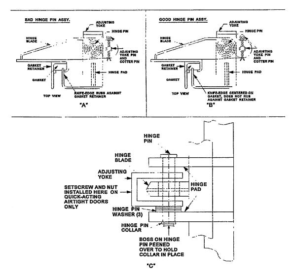
Figure 600-2.31. Hinge Pin Assemblies
