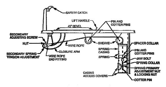
Figure 600-6.1. Typical Hatch
