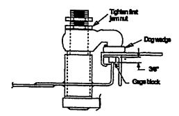
Figure 600-2.48. Dog Adjustment without Gasket Installed
