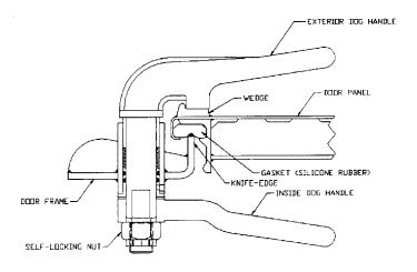
Figure 600-2.66.D. Dog With Self-locking Nut
