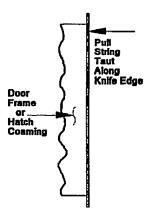
Figure 600-2.13. Knife-Edge Inspection Using String Method
