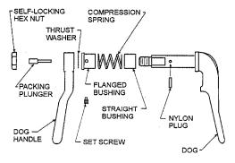
Figure 600-2.45. Individually Dogged Door Dog Lever Assembly (Cross Sectional View) Modified by MACHALT 167-31004(ECP-444)
