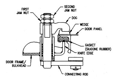
Figure 600-2.48.B Dog With Jam Nuts
