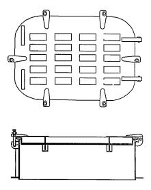
Figure 600-5.1 Raised Watertight Hatch
