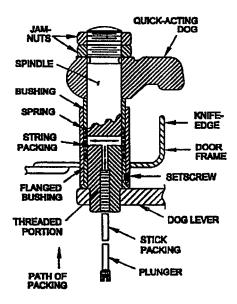
Figure 600-2.6. Quick-Acting Door Dog Assembly (Cross Sectional View)
