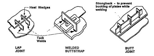
Figure 600-2.74. Methods of Securing Welded Structure
