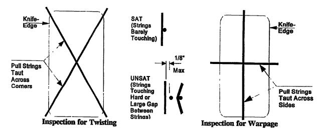
Figure 600-2.18. Knife-Edge Inspection for Warpage
