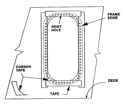
Figure 600-2.75. Dielectric Tape Installation
