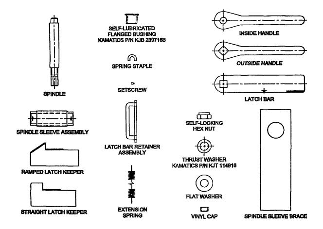
Figure 600-4.2. Latch Device Assembly Replacement Parts
