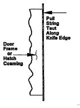
Figure 600-2.35. Knife-Edge Inspection Using String Method
