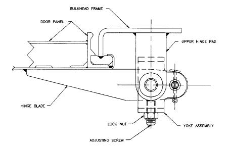
Figure 600-2.66.F. Bound Hinge Arrangement
