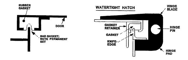
Figure 600-2.20. Gasket Inspection
