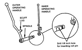
Figure 600-2.55. Quick-Acting Operating Handle Temporary Repair
