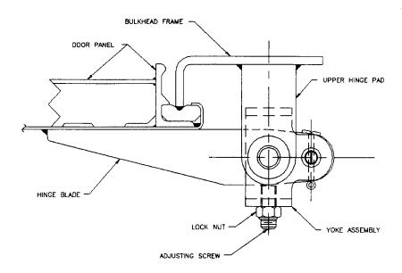
Figure 600-2.48.F Bound Hinge Arrangement
