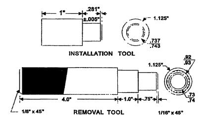
Figure 600-2.59. Conrod Removal and Installation Tool
