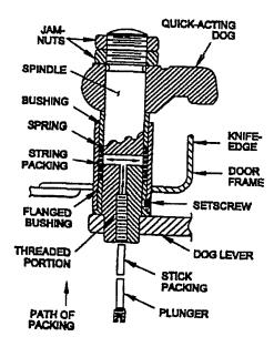
Figure 600-2.10. Quick-Acting Door Dog Assembly (Cross Sectional View)
