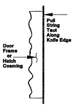
Figure 600-2.17. Knife-Edge Inspection Using String Method
