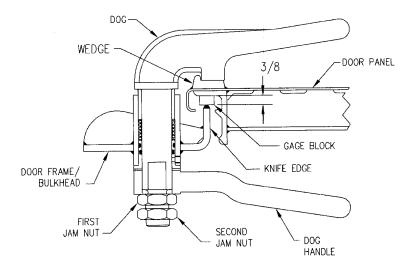
Figure 600-2.66. Dog Adjustment Without Gasket Installed
