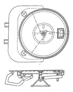
Figure 600-7.3. Flush Watertight Scuttle (2722 Kg (6000 Lb) Wheel Load
