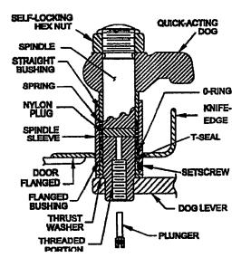
Figure 600-2.23. Quick-Acting Door Dog Lever Assembly (Cross Sectional View) Modified by MACHALT 167-31004(ECP-444)
