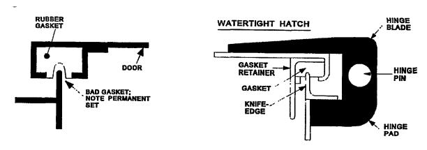
Figure 600-2.42. Gasket Inspection
