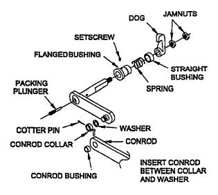
Figure 600-2.57. Quick-Acting Door Lever Assembly
