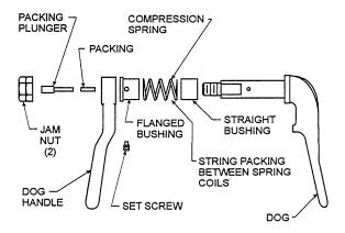
Figure 600-2.32. Individually Dogged Door Dog Assembly (Cross Sectional View)
