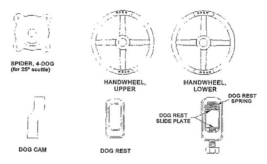
Figure 600-7.6. Scuttle Components
