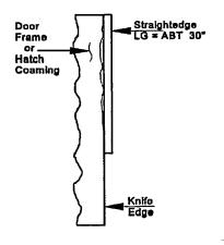
Figure 600-2.38. Knife-Edge Inspection Using Straightedge Method
