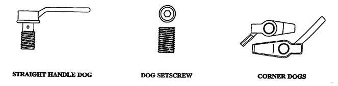
Figure 600-3.4. Straight Handle Bushing, Dog Setscrew, and Corner Dogs
