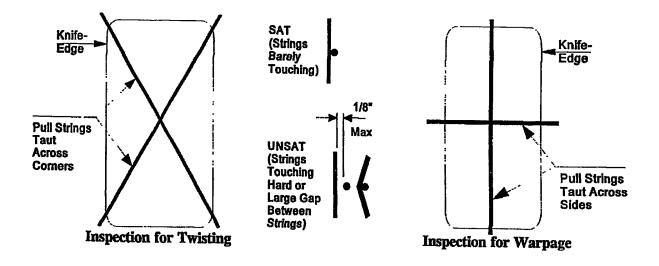
Figure 600-2.14. Knife-Edge Inspection for Warpage
