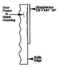
Figure 600-2.16. Knife-Edge Inspection Using Straightedge Method
