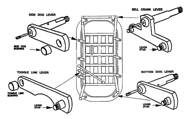
Figure 600-2.56. Quick Acting Door Levers
