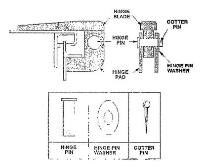
Figure 600-5.9 Watertight Hatch Hinge Assembly
