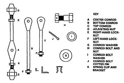
Figure 600-3.7. Linkage Assembly (Typical)
