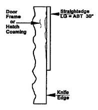
Figure 600-2.12. Knife-Edge Inspection Using Straightedge Method
