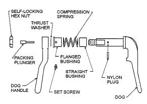
Figure 600-2.33. Individually Dogged Door Dog Lever Assembly (Cross Sectional View) Modified by MACHALT 167-31004 (ECP-444)
