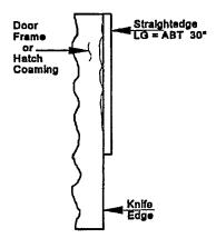
Figure 600-2.34. Knife-Edge Inspection Using Straightedge Method
