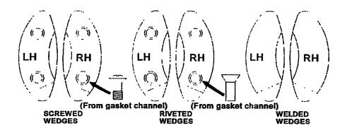
Figure 600-2.25. Watertight Door Wedges
