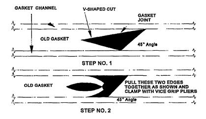
Figure 600-2.47A Gasket Removal
