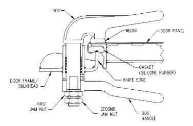
Figure 600-2.66.B. Dog With Jam Nuts
