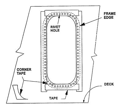
Figure 600-2.77. Dielectric Tape Installation
