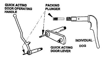
Figure 600-2.67. Packing Plunger Locations
