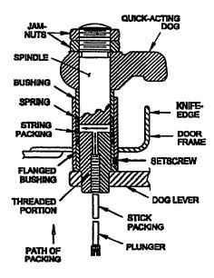
Figure 600-2.22. Quick-Acting Door Dog Assembly (Cross Sectional View)
