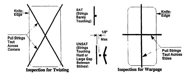
Figure 600-2.40. Knife-Edge Inspection for Warpage
