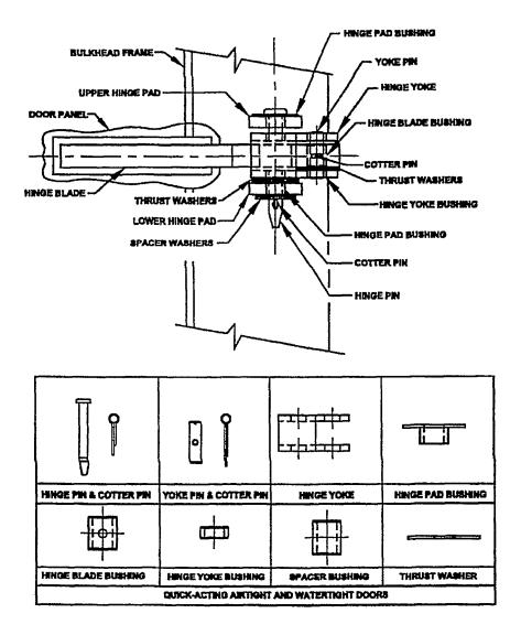
Figure 600-2.71. Watertight Door Hinge Components (For Doors With MACHALT 167-31006 (ECP-518) or MACHALT 167-31011 (ECP-538) Installed)
