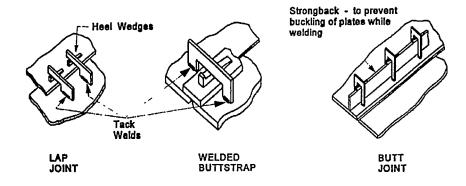
Figure 600-2.76. Methods of Securing Welded Structure
