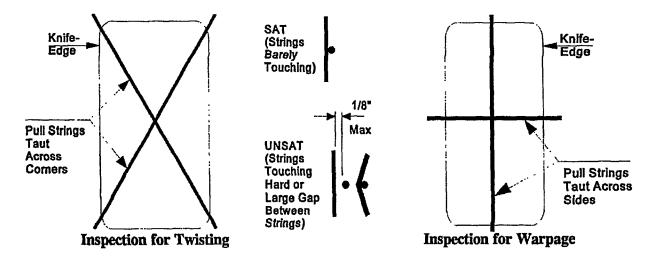
Figure 600-2.36. Knife-Edge Inspection for Warpage
