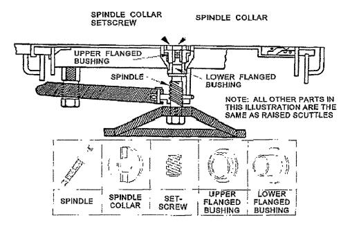
Figure 600-7.7. Flush Scuttle Components
