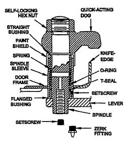
Figure 600-2.53. Quick-Acting Door Dog Assembly (Cross Section View) Modified by MACHALT 167-31010 (ECP-526)
