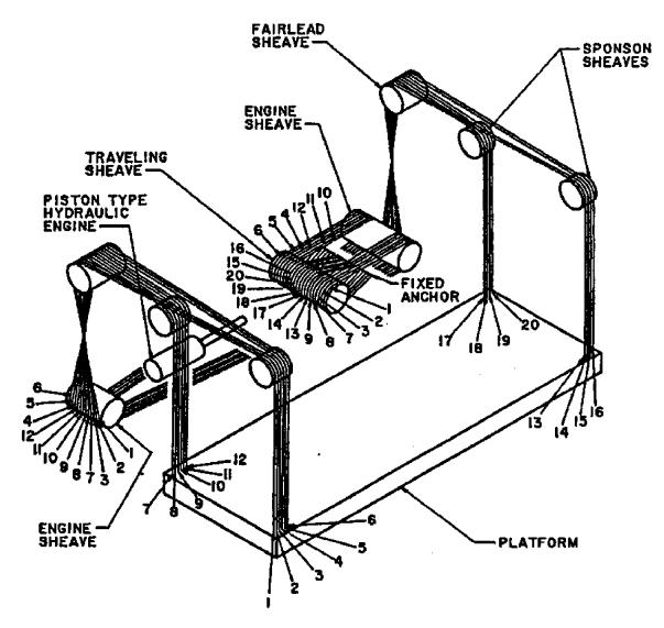
Figure 588-1-5. Typical Aircraft Elevator Reeving Arrangement
