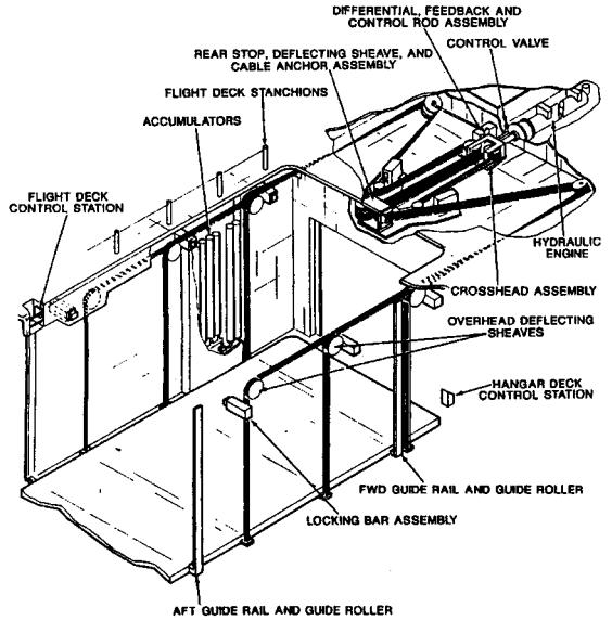
Figure 588-1-1. Typical Inboard Elevator Arrangement
