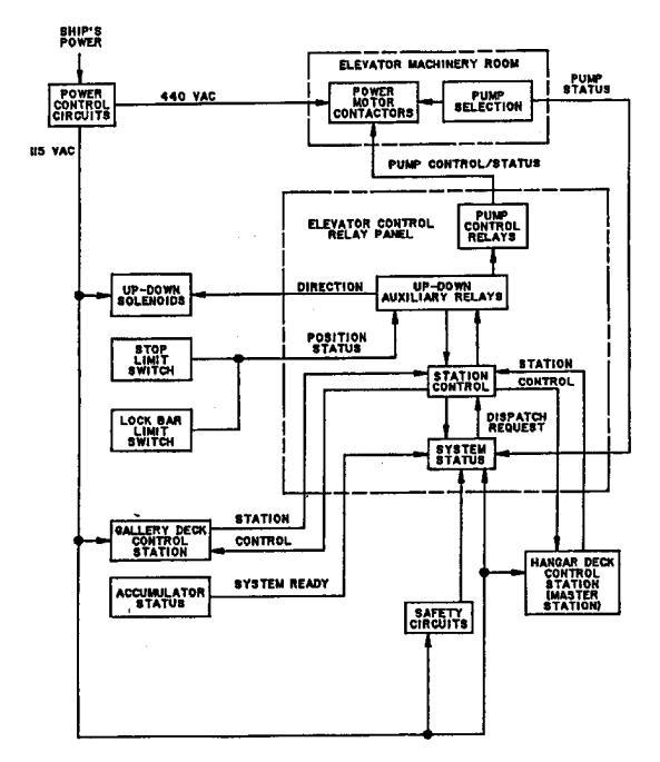
Figure 588-1-7. Control System Functional Block Diagram
