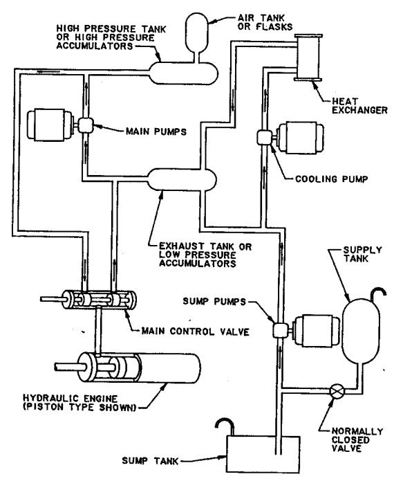
Figure 588-1-6. Simplified Hydraulic Schematic
