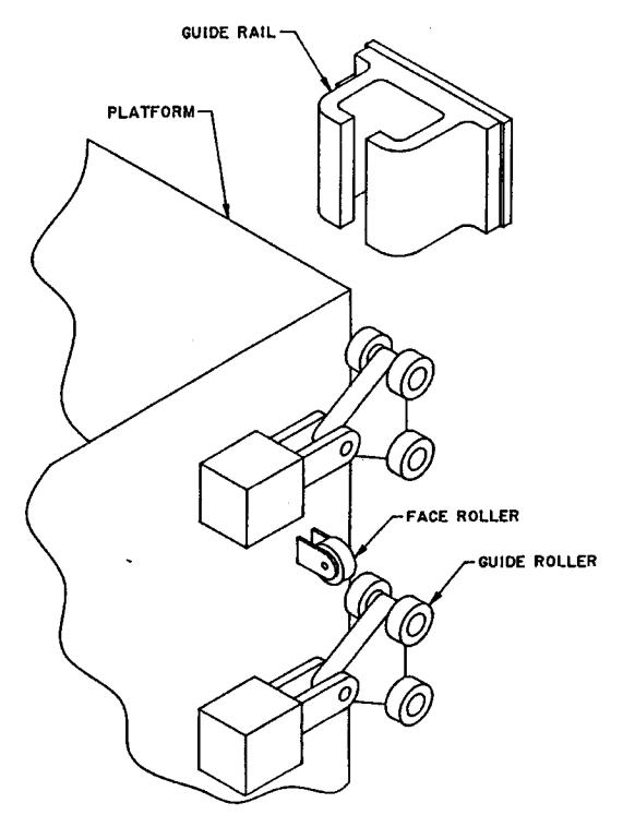
Figure 588-1-4. Typical Guide Roller Arrangement
