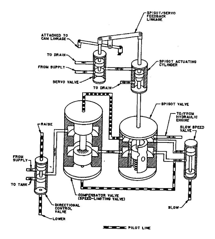
Figure 588-1-10. Pressure-compensated Main Flow Control Valve
