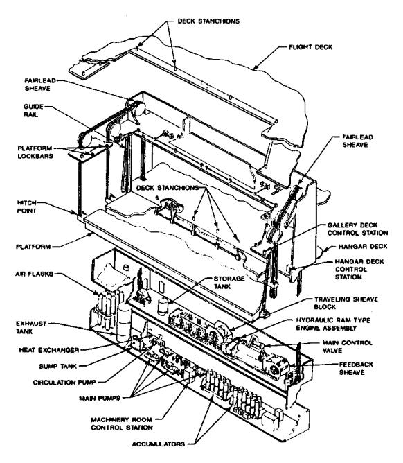
Figure 588-1-2. Typical Deck Edge Elevator Arrangement
