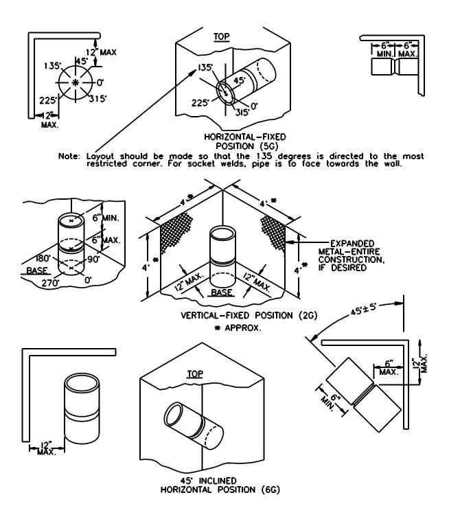
FIGURE 21. <u>Typical layout and construction for restricted accessibility</u> <u>qualification test assembly positions</u>.
