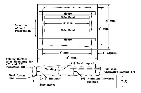
FIGURE 4a. <u>Test assembly for procedure qualification</u> of A-45 cladding for corrosion-resistance
