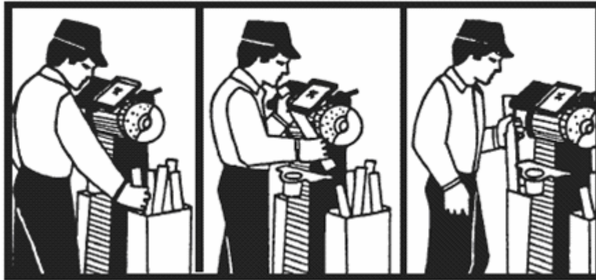
Figure 1. A worker performing the basic job steps for grinding iron castings.
