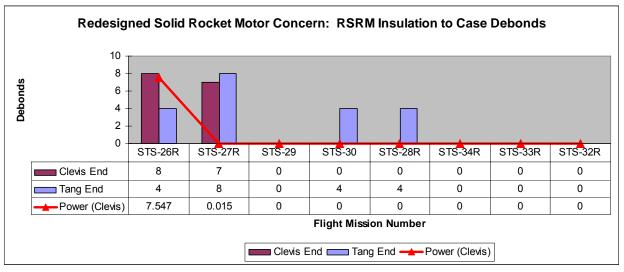
Note: Clevis end statistically significantly downward trend R-squared (power) = 0.74, Tang end statistically non-significant trend
