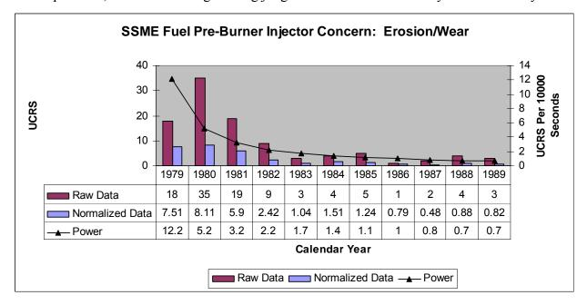
Figure E.5-2: SSME Fuel Pre-Burner Injector Concern: Erosion and Wear
