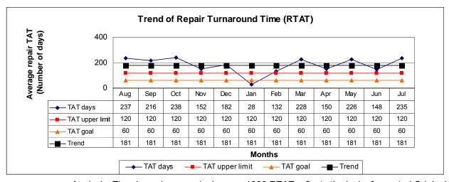
Analysis: The sharp decrease in January 1989 RTAT reflects the lack of reported Original Equipment Manufacturer (OEM) activity and not reduced repair time. Since OEM RTAT is much higher than XYZ RTAT, decreased OEM activity will cause a decrease in the program RTAT trend. Recommendations: develop new RTAT trend charts. Base trend on open and closed Preproduction Readiness Reviews (PRR's).
