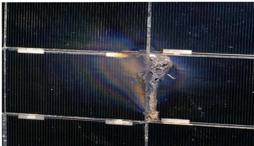
Figure 7—Arc Site of Sustained Arc on EOS-AM1 Sample Array. Cells are 2x4 cm. (Ferguson and Hillard, 2003)
