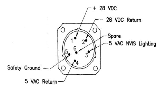
FIGURE 2. Wiring.
