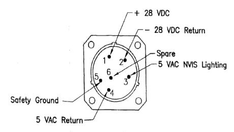
FIGURE 2: Wiring
