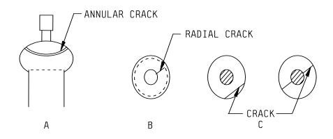
FIGURE D-2. Cracks.
