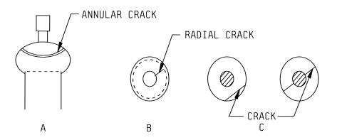
FIGURE D-2. Cracks.
