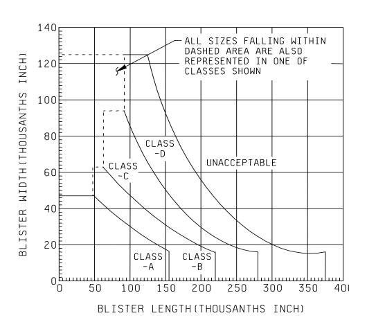
FIGURE D-1. Classification of soft glass unbroken blister sizes.
