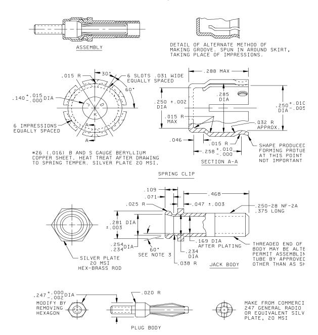
FIGURE C-2. Locking jack and plug for magnetron tubes.
