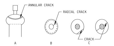
FIGURE D-2. Cracks.
