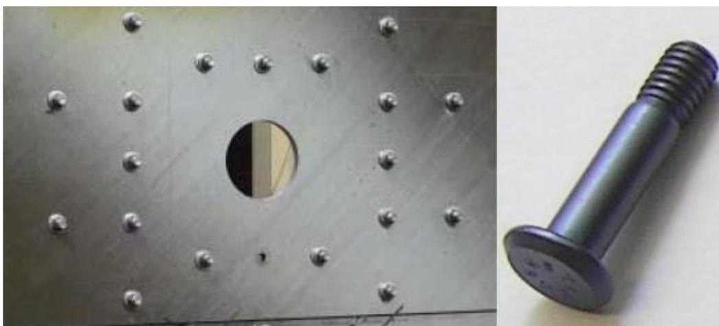
Figure 1.6: Bolted composite structure and mechanical fastener [22]
