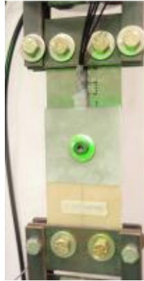
Figure 3-1: Lap joint loaded into the MTS machine.
