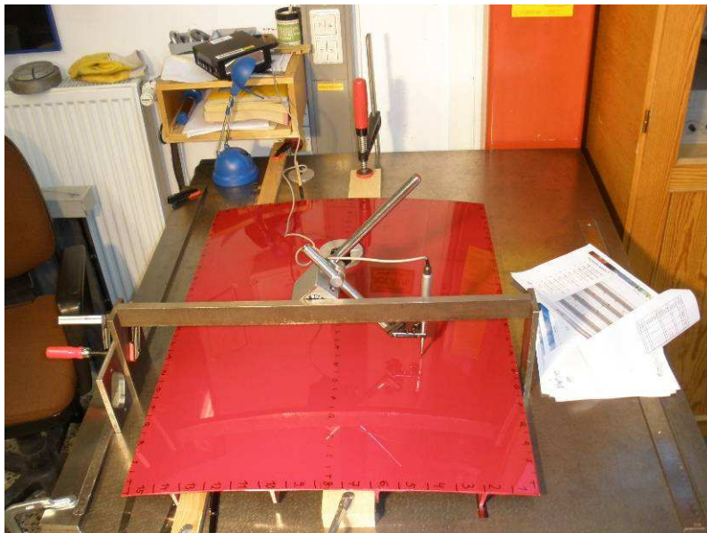
Figure 35: Set-up of dent depth measurements.
