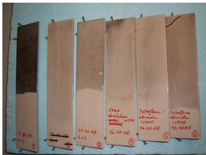
Figure 40: Trials for dirt application using acetylene soot for specimen 1 to 3, candle soot for specimen 4 and paraffin oil soot for specimens 5 and 6.
