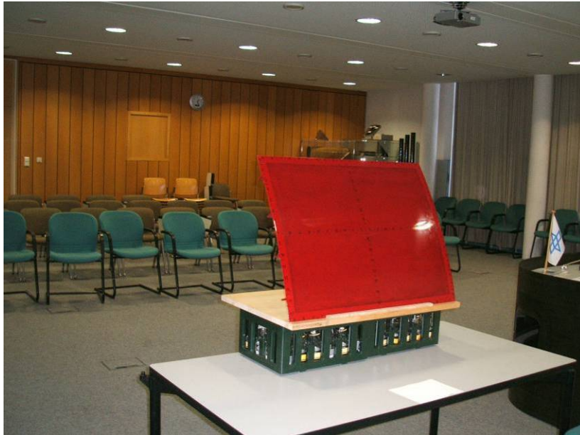
Figure 49: Lighting in meeting room 101 of Building 118 at the DLR Braunschweig site. Three light bulbs in each ceiling lamp provide around 400 lux on the table surface in the foreground.
