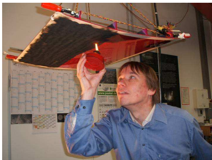
Figure 41: Application of paraffin oil soot on panel 1 with red glossy coating. The paraffin flame had no effect on the glossy coating.
