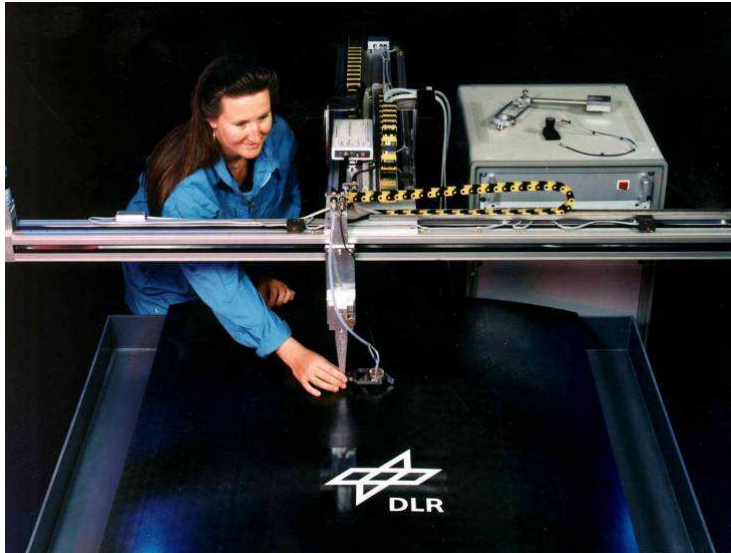
Figure 19: The ultrasonic scans were conducted with a stationary high resolution device using water coupling.
