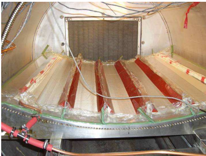
Figure 10: Stringers are supported by silicone cores (red pieces) with triangular cross sections to prevent the from collapsing during curing.
