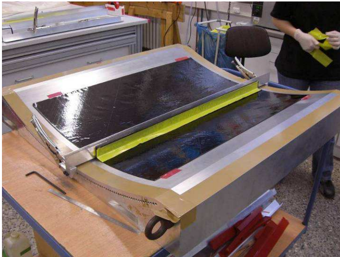
Figure 9: Placement of stringer on skin laminate. A tool with 1 m radius was used for the manufacturing test.
