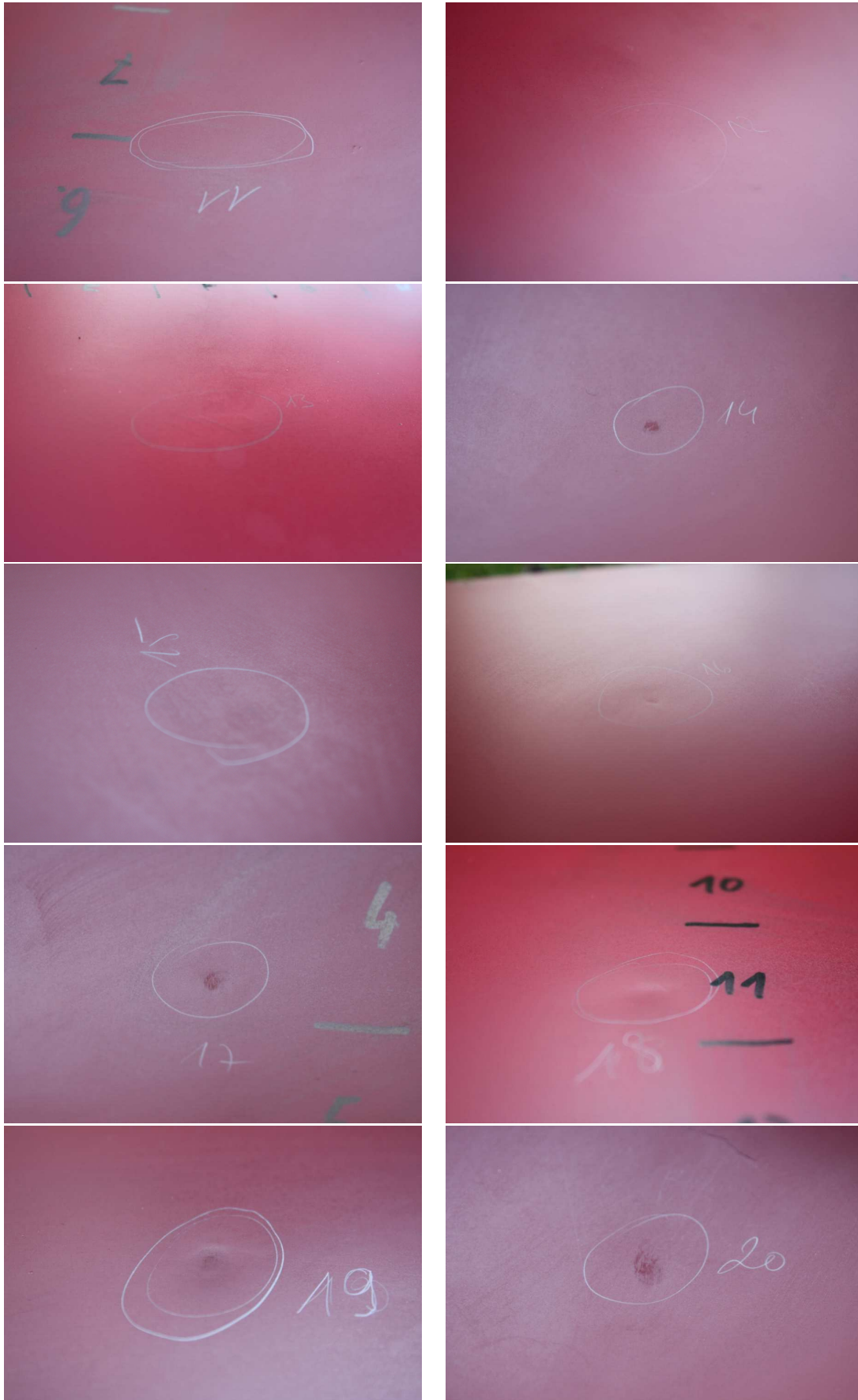
Figure 32: Impact locations 11-20 on panel 2 after impacting. The size of the markings on the panel does not correspond to size of internal damage.
