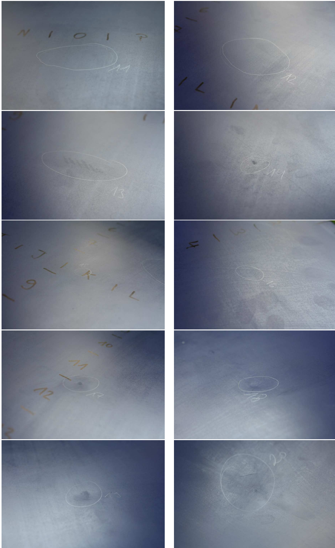
Figure 31: Impact locations 11-20 on panel 1 after impacting. The size of the markings on the panel does not correspond to size of internal damage.
