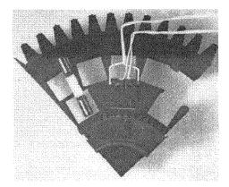
Figure 28. Tensile and compact tension specimens machined from the Nene X disc. The eletrical leads are part of the automated DC-PD technique used to monitor crack growth during testing.
