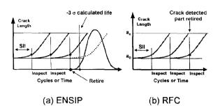
Figure 12. Schematic representations of the damage tolerance approaches based on (a) MIL-STD 1783 (ENSIP); (b) Retirement for Cause (RFC).
