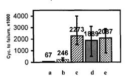
Figure 23. The fretting fatigue life of Ti-6Al-4V: a = base metal; b = CuNiln +  $MoS_2$ ; c = shot peened; d = shot peened + CuNiln +  $MoS_2$ ; e = shot peened +  $MoS_2$ .
