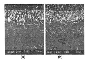
Figure 8. Service-induced precipitation of sigma phase immediately below the protective coating in a Mar-M246 turbine blade from a CF transport aircraft engine; (a) new blade; (b) service-exposed blade.
