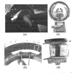
Figure 18. Hardware for thermal fatigue testing of NGVs in burner rig: (a) and (b) specimen fixture and cooling arrangement; (b) close-up of specimens mounted in fixture; (c) fine wire thermocouples spot welded on air foils for temperature calibration
