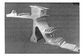
Figure 16. Example of seal teeth repair using the Dabber™ technique (Courtesy of Liburdi Engineering, Hamilton, Ontario).
