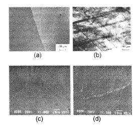
Figure 6. Effects of service exposure on microstructure (a) Virgin disc; (b) Service exposed disc showing evidence of dislocation activity (PSB) indicative of LCF damage accumulation (c) Virgin disc spacer; (d) Service exposed disc spacer showing evidence of creep voids along grain boundaries; [1,12].
