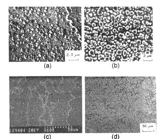
Figure 7. Internal microstructural damage in high time blades: (a) bimodal distribution of gamma prime precipitates in new blade; (b) coarsening of gamma prime precipitates and elimination of secondary gamma prime in service exposed IN738 turbine blade; (c) precipitation of carbides (arrows) along grain boundaries in IN738 turbine blade; (d) precipitation of sigma phase in IN 713C blade [13,14].
