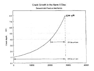
Figure 32. Damage tolerance based life cycle management curve for Nene X turbine discs using 90/95 POD value of the LPI tehnique as the detection limit of the technique [40]
