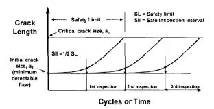
Figure 11. The Damage Tolerance approach.
