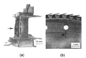
Figure 9. (a) Airfoil bowing, loss of coating and cracking of a CF T56-A15 first stage nozzle guide vane; (b) Crack initiating from bolt hole in CF j85 CAN40/15 compressor disc [15,16].
