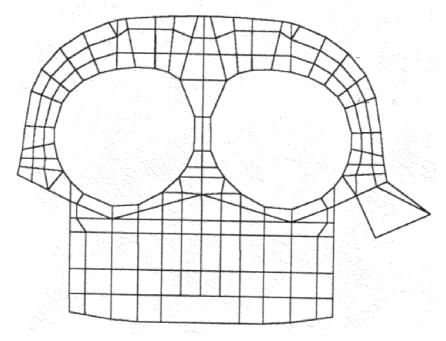
Fig. 2.2-4A Coarse Mesh FE-Model of Cemter Fuselage Frame
