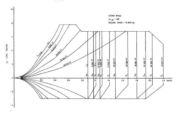
Fig. 1.2.1-1 Ma-n Diagram in Altitude
