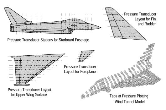
Fig. 1.4-1 Prototype Pressure Plotting for Flight Load Survey
