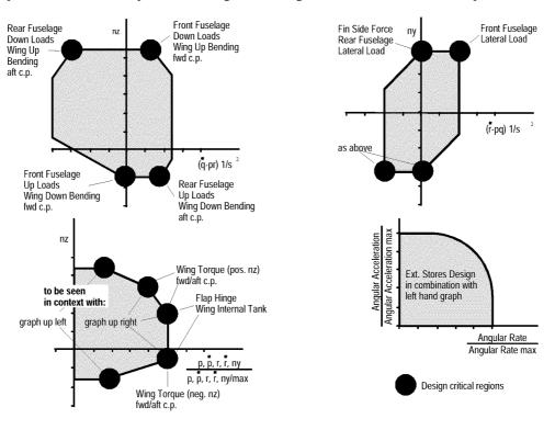
Fig. 1.2.3-2 Flight Parameter Envelopes for Structural Design
