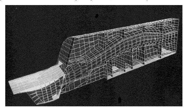
Fig. 2.2-2 FE-Half-Model of Center Fuselage Structure
