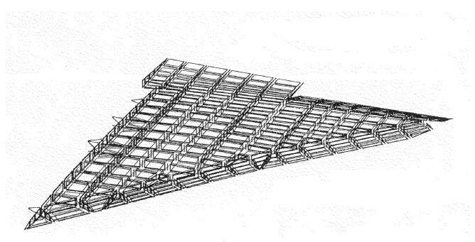
Fig. 2.2-1 Coarse Mesh FE-Model of Wing Structure
