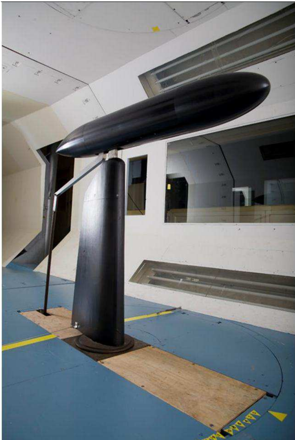
Figure 6: Submarine model mounted in LSWT, showing pylon support and pitch control arm.
