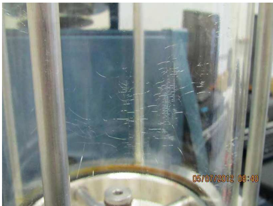
Figure 34: Wash Housing showing crazing
