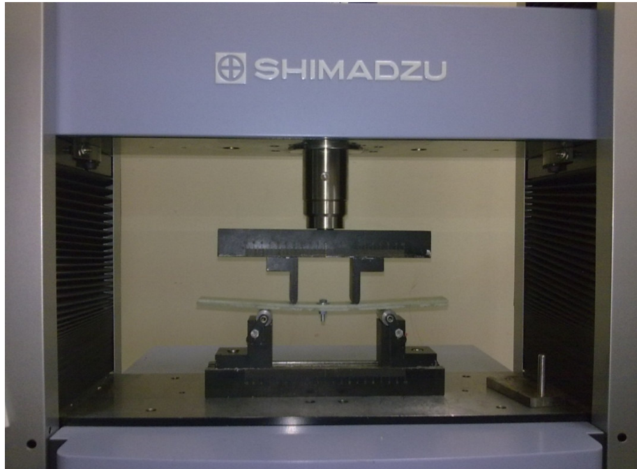
Figure 4.5 Bolt loaded glass-epoxy laminated composite four point bending test process
