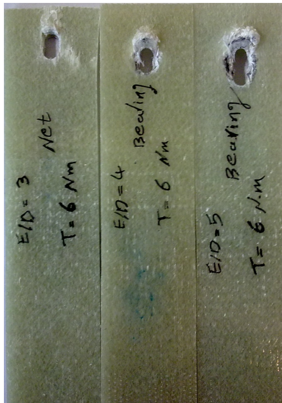
Figure 5.3 The photograph of some tested specimens at traction for T=6 Nm and variable E/D ratio with various failure modes.
