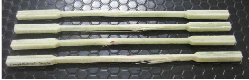
Figure 3.3 Deformed tensile test specimens to obtain longitudinal elasticity module ( E_1 ) and poisson ratio ( \nu_{12} )
