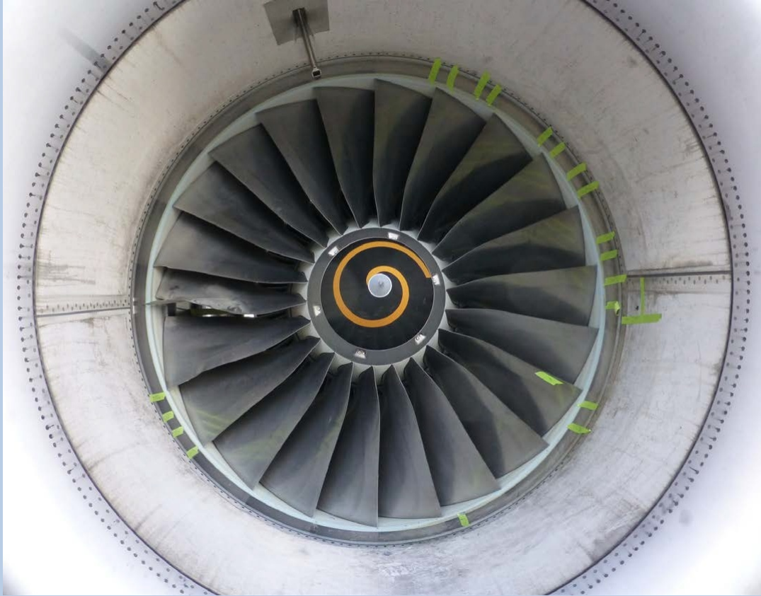
Fan blade damage caused by ingesting a duck. Source: Operator
