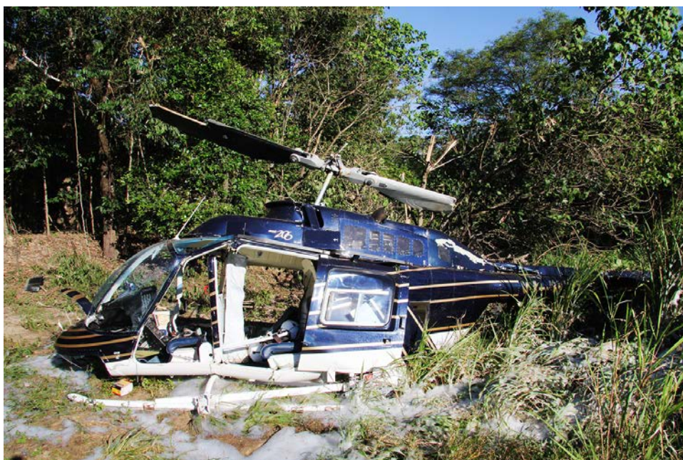
Wirestrike, Bell 206B III JetRanger helicopter (VH-BHU), near Mossman Hospital, Queensland (AO-2011-067) (image courtesy of Queensland Police)
