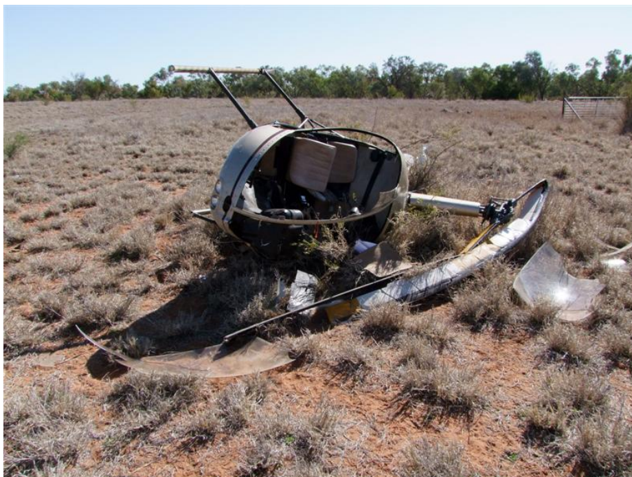
Wirestrike, Robinson R22 Beta II helicopter (VH-HSW), 90 km SW of Cunnamulla, Queensland (AO-2011-080) (image courtesy of Queensland Police)
