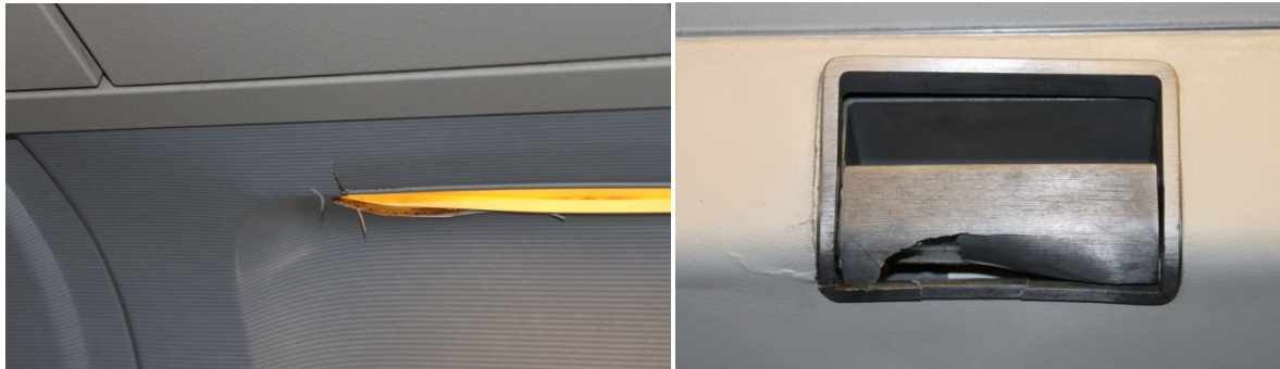
Damage to window reveal (L) and overhead locker (R) – Turbulence event, Boeing 767-300 (VH-OGR), near Perth Airport, Western Australia (AO-2011-064)
