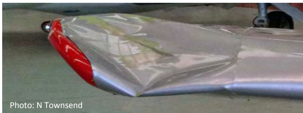
Figure 11: Frontal image of R-2160 right leading edge tip following a birdstrike with an ibis, 19 December 2009
