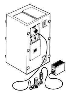
Frequency = F1  $\pm$ 0.1 GHz (See (S) TM-11-5865-202-30 (U) for values of F1, F2 and F3.) ►If the frequency is outside limits of tolerance. <del>-------</del> perform the following steps. TP Remove semi-rigid а. connector from jack J2 on rear of unit. Disconnect frequency meter from jack J4, and connect to RF OUT R12 connector on front panel of unit. TP2
