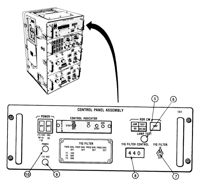
CONTROL PANEL ASSEMBLY CONTROLS AND INDICATORS
