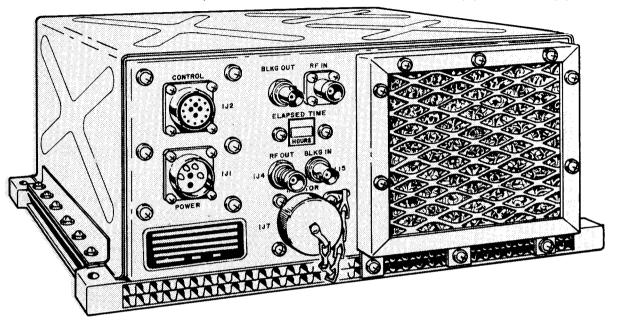
• Test Set, Countermeasures Set TS-3614/ALQ-136(V) (FLTS).
