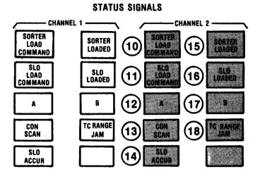
The LAMP TEST pushbutton (S13) lights all Status signal lamps on the Status Panel for test purposes.
