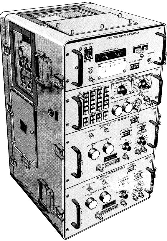
TEST SET, COUNTERMEASURES SET TS-3615/ALQ-136(V)
