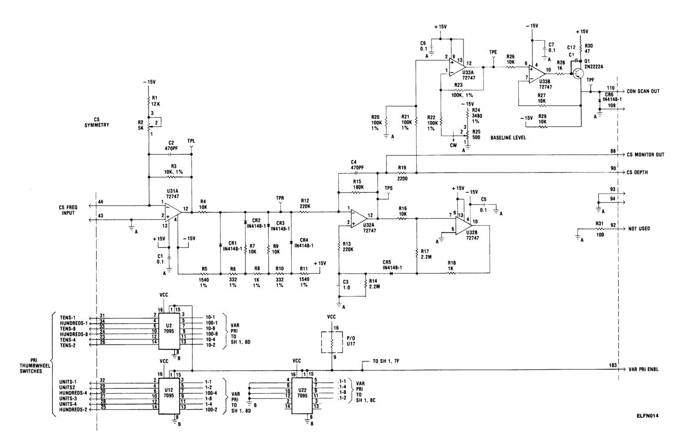
Figure FO-11 CCA, CS AND PULSE CONTROL 1A3A2/ 1A4A2 SCHEMATIC DIAGRAM (Sheet 2 of 2)
