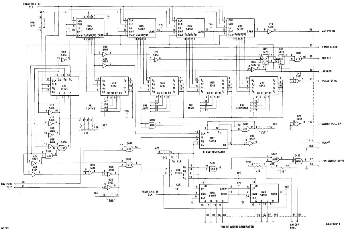
NOTES: UNLESS OTHER SPECIFIED: RESISTORS P/O RESISTOR NETWORK, U16, ARE 2200 OHMS. ALL CAPACITORS ARE IN MICROFARADS.
