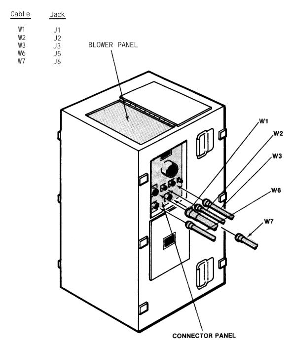
Make sure 115 VAC, 60 Hz switch on the control panel is set to OFF. Connect cable W6 to a 115 Vac power source.
