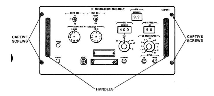
(5) **Firmly** grasp the two handles of the assembly to be removed and gently **pull** the assembly out. Continue pulling slowly until the assembly is almost out of its closure at which time-carefully and slowly pull-it free of the case and gently lower the assembly to the test bench.
