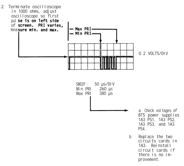
c. Replace RF Modulation Assembly 1A3.
