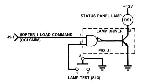
LAMP TEST Switch S13, when depressed, applies a ground level to one input of the nand gate on the lamp driver assembly. The high output from the nand gate turns on the output power drivers, illuminating the lamps on the status panel.
