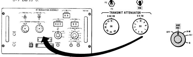
2. On Status Panel 1A2, set INPUT RF ATTENUATOR 0-60 DB and 0-9 DB to 0.
