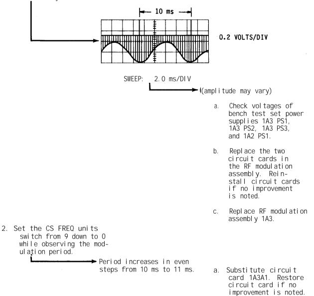
b. Check con scan frequency select switch 1A3S2.
