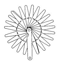
Figure 3-70. Thickness Gauge
