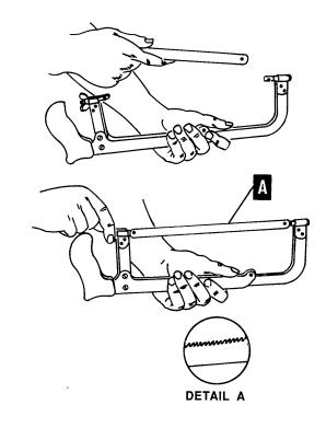
Figure 4-99. Installing a Hacksaw Blade
