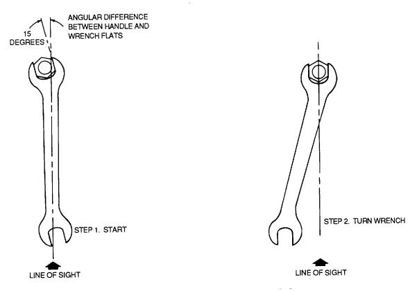
Figure 8-24. Tightening to 15-Degree Wrench Arc
