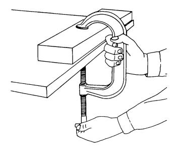
Figure 4-56. Using Carriage Clamp
