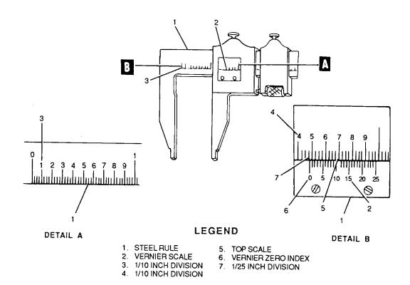
Figure 3-32. Reading a Measurement on a Vernier Caliper
