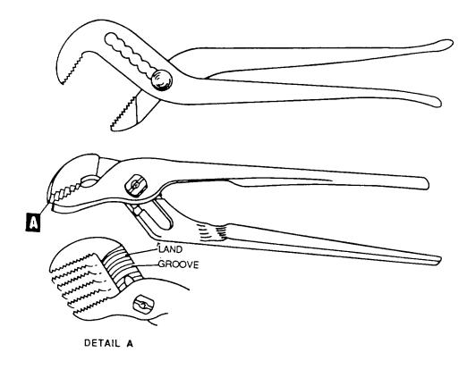
Figure 4-46. Water Pump Pliers
