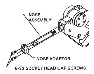
Figure 7-28. Removal of Safety Cable Tool Nose Assembly
