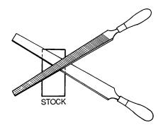
Figure 4-77. Filing for a Flat Surface
