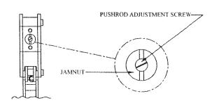
Figure 7-29. Adjustment of Safety Cable Indenter (Same for hand and pneumatic tool models)
