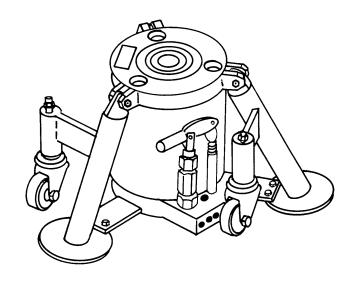
Figure 9-7. Tripod Jack, 12-Ton
