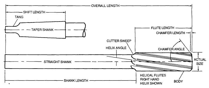
CHUCKING REAMER, STRAIGHT AND TAPER SHANK
