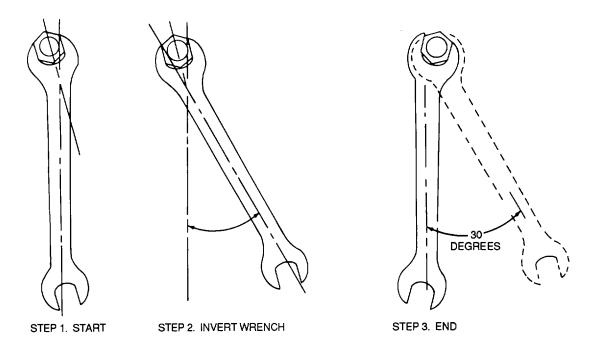
Figure 8-27. Tightening to 30-Degree Wrench Arc
