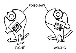
Figure 4-35. Proper Procedure for Pulling Adjustable wrenches
