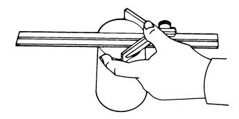
Figure 3-15. Locating Diameter of Cylinder
