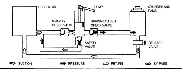
Figure 9-6. Jack Hydraulic Schematic Diagram
