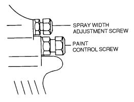
Figure 5-4. Adjustment of Spray Pattern
