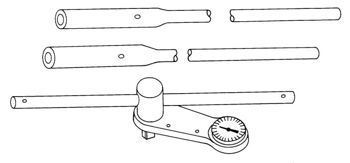
Figure 8-11. Type II, Style C Torque Wrench-Rigid Cases with Presetting Dial (Direct Reading with Flashlight Signal)
