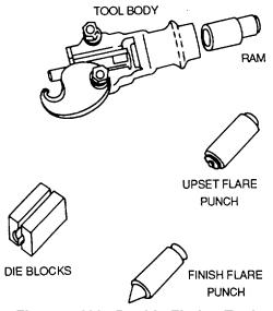
Figure 4-122. Double-Flaring Tool
