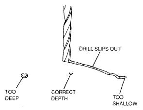
Figure 4-84. Center Punch for Drilling
