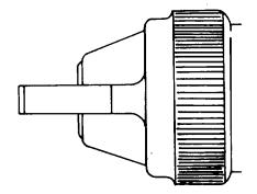
Figure 5-3. Nozzle Position to Produce Vertical Fan
