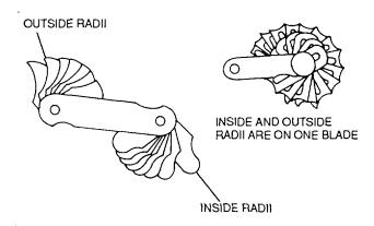
Figure 3-73. Fillet and Radius Gauges
