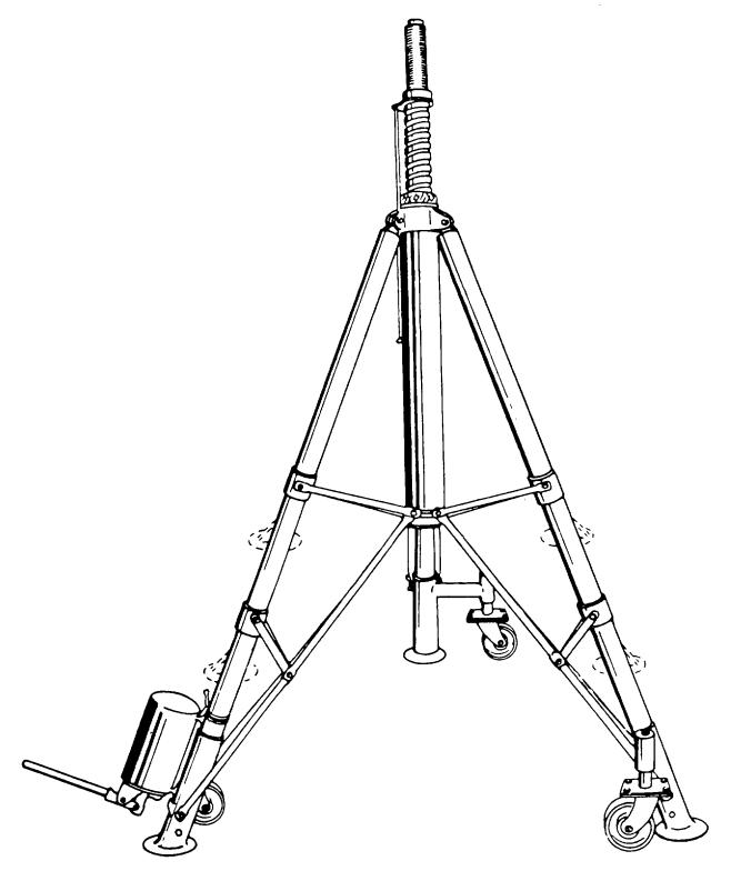
Figure 9-8. Tripod Jack, 5-Ton
