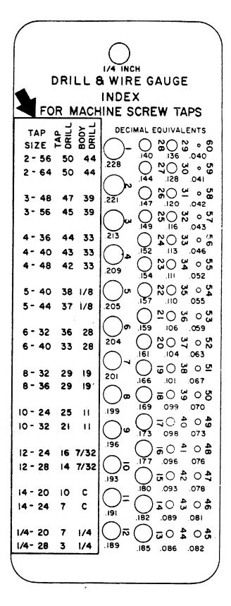
Figure 4-102. Correct Drill Sizes for Tapping
