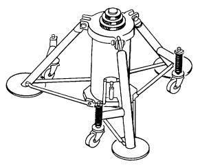
Figure 9-9. Tripod Jack, 3-Ton
