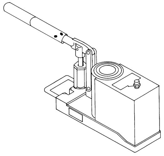
Figure 9-11. Self-Contained Jack, 10-Ton
