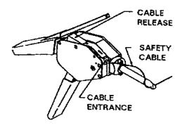
Figure 7-23. Pre-set Tension Safety Cable Application Tool
