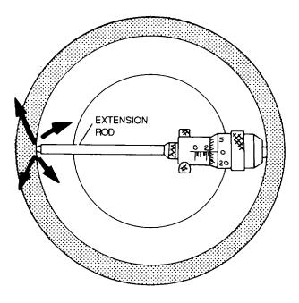
Figure 3-40. Using Inside Micrometer with Extension Rod
