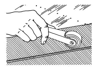
Figure 7-19. Using Diecer Boot Roller
