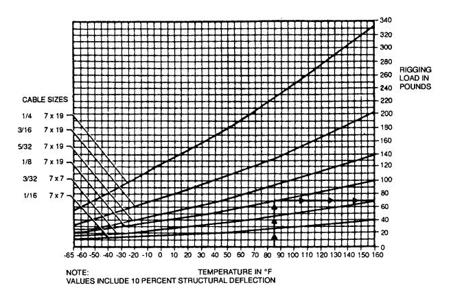
Figure 7-7. Typical Cable Rigging Tension Chart
