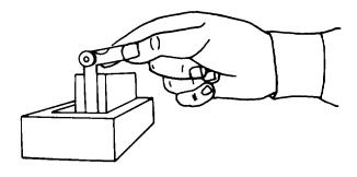
Figure 3-71. Using a Thickness Gauge
