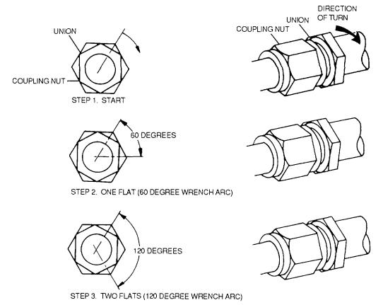
Figure 8-26. Tightening to 60- or 120-Degree Wrench Arc
