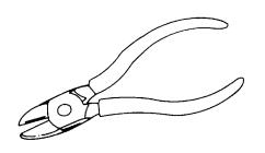
Figure 4-42. Diagonal Cutting Pliers
