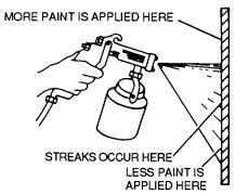
Figure 5-6. Effect of Applying Paint at an Angle
