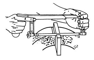
Figure 4-100. Proper Way to Hold a Hacksaw
