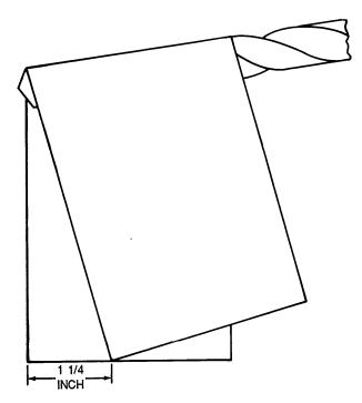
Figure 4-90. Measuring Heel Angle
