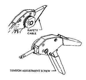
Figure 7-24. Adjustable Tension Safety Cable Tool
