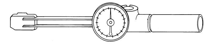
Figure 8-8. Type I, Class 2, Style B Torque Wrench - De.ecting Beam with indicating Dial (Direct Reading with Audible Signal)
