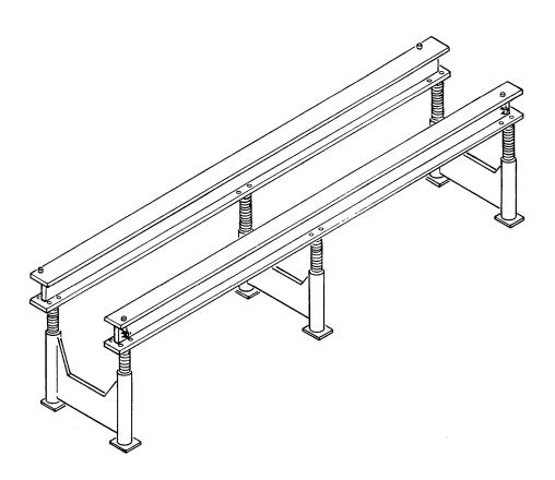
Figure 9-3. Engine Maintenance Stand
