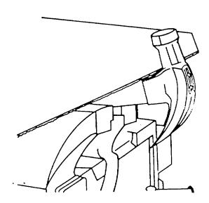
Figure 4-10. Removing Broken Handle
