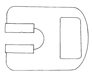
Figure 3-59. Snap Gauges
