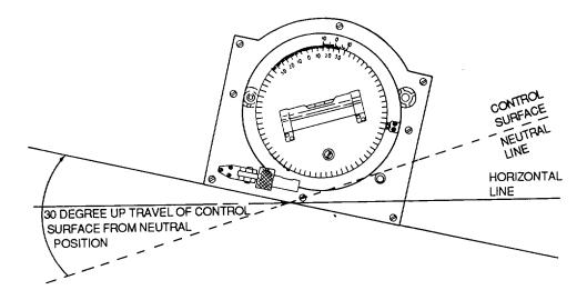
Figure 7-3. Measuring Control Surface Angle at Full Throw
