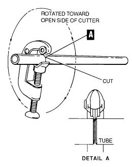
Figure 4-116. Cutting Tube with Tube Cutter
