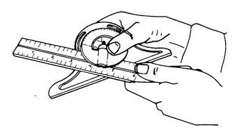
Figure 3-17. Installing Protractor Head on Rule
