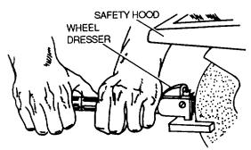
Figure 6-6. Dressing a Grinding Wheel
