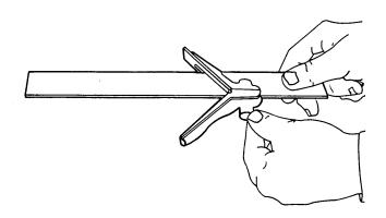
Figure 3-14. Setting the Center Head
