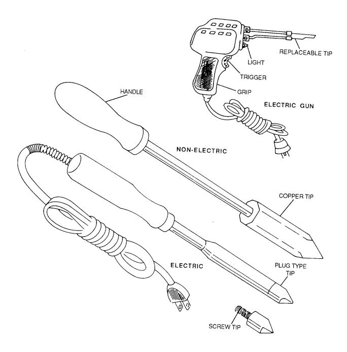
Figure 7-22. Soldering Tools
