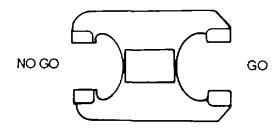
Figure 3-60. Solid Nonadjustable Snap Gauge
