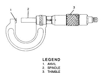
Figure 3-41. Parts of a Micrometer
