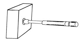
Figure 3-80. Measuring Hole with a Small Hole Gauge
