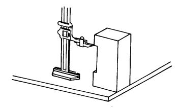
Figure 3-51. Typical Height Gauge
