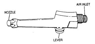
Figure 5-13. Air Blow Cleaning Gun
