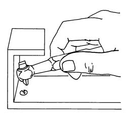
Figure 4-18. Using Offset Ratchet Screwdriver
