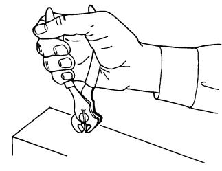
Figure 4-113. Flush Cutting
