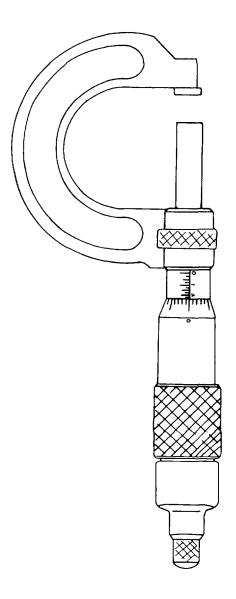
Figure 3-34. Outside Micrometer
