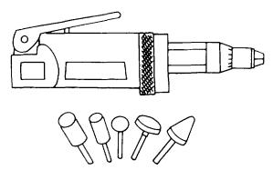
Figure 5-16. Pneumatic Grinder
