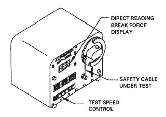
Figure 7-27. Electronic Safety Cable Pull Tester
