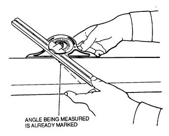
Figure 3-19. Checking Angle
