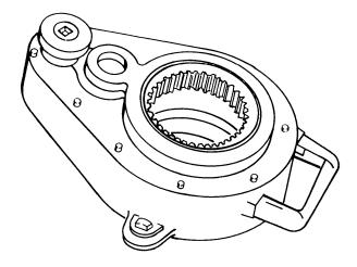
Figure 8-22. Hub Nut Torque Multiplier
