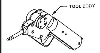
Figure 7-25. Pneumatic Safety Cable Application Tool
