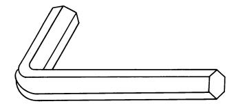
Figure 4-31. Hexagonal Setscrew Wrench (Allen Wrench)
