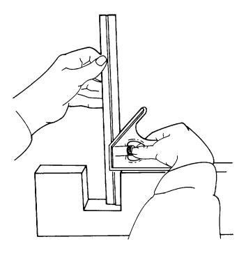
Figure 3-20. Determining Depth with the Square Head
