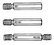
Figure 3-54. Plug Gauges
