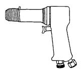
Figure 5-17. Pneumatic Hammer
