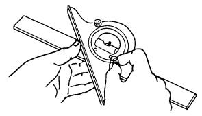
Figure 3-18. Loosening Protractor Adjustment Screws
