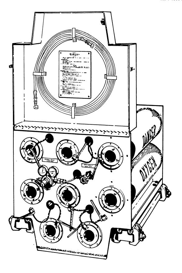
Figure 9-24. Oxygen Servicing Unit
