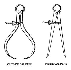
Figure 3-25. Spring-Joint Calipers
