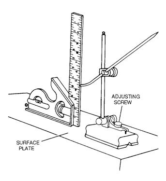
Figure 3-46. Setting Height on a Surface Gauge
