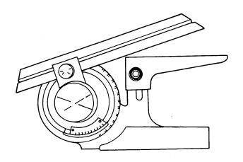
Figure 3-12. Bevel Protractor
