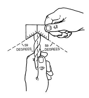
Figure 4-89. Using Drill Grinding Gauge
