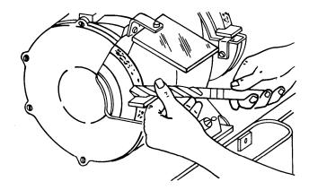
Figure 4-87. Hand Grinding of Cutting Edge
