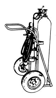
Figure 9-17. Nitrogen Servicing Unit
