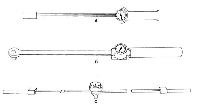
Figure 8-7. Type I, Class 2, Style A Torque Wrenches - De.ecting Beam with Indicating Dial (Direct Reading)
