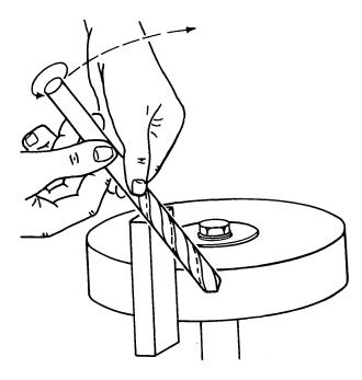
Figure 4-88. Hand Grinding of Heel to Cutting Edge
