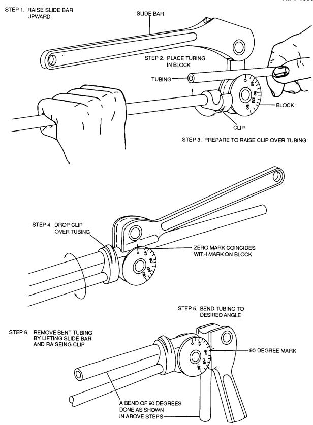
Figure 4-118. Bending Tube
