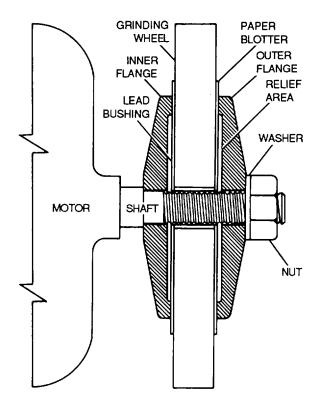
Figure 6-5. Grinding Wheel Installation
