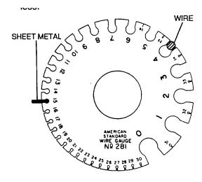
Figure 3-72. Measuring Sheet Metal and Wire
