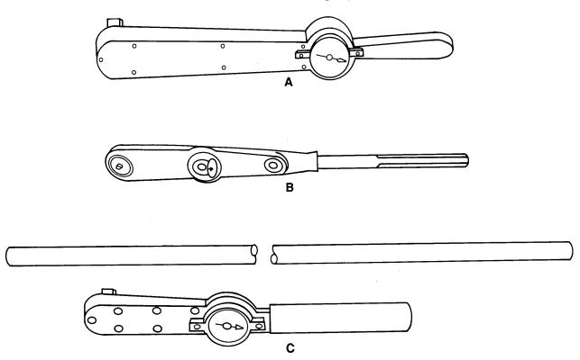
Figure 8-9. Type II, Style A Torque Wrench - Rigid Case with Indicator Dial (Direct Reading)
