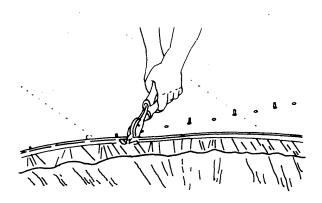
Figure 7-17. Using Deicer Boot Pliers
