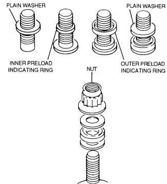
Figure 8-31. Installation of Preload Washers on a Stud mashers on a stud
