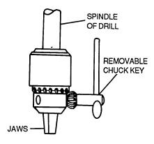
Figure 6-3. Three-Jaw Chuck and Chuck Key
