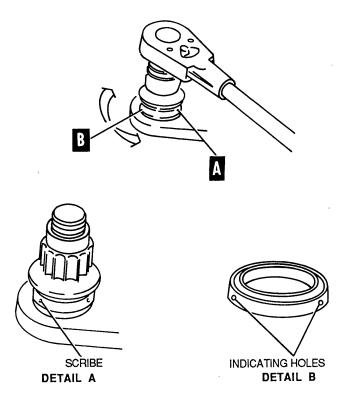
Figure 8-33. Tightening Preload Washers
