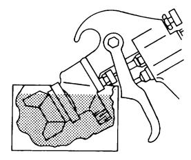
Figure 5-9. Soaking a Paint Gun
