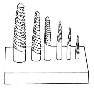
Figure 4-108. Spiral Screw Extractors
