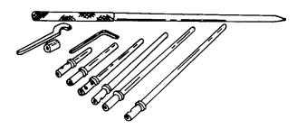
Figure 3-37. Extension Rods for Inside and Depth Micrometers
