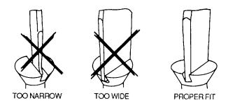
Figure 4-17. Proper Fit of Screwdrivers
