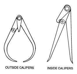
Figure 3-26. Transfer Calipers
