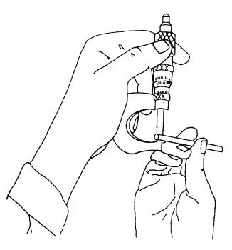
Figure 3-39. Using Outside Micrometer
