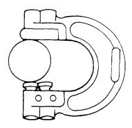
Figure 3-68. Correct GO Dimension for Cylindrical Part
