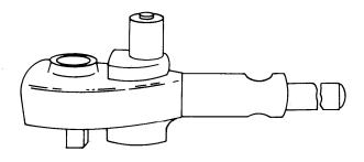
Figure 8-21. General Use Torque Multiplier
