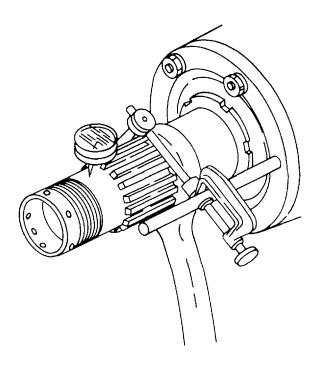
Figure 3-76. Checking Propeller Shaft Run Out
