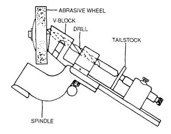
Figure 4-85. Machine Grinding a Drill Bit
