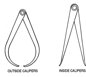
Figure 3-24. Simple Calipers
