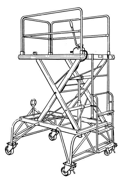
Figure 9-2. Type B-4A Maintenance Stand
