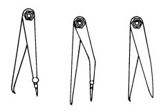
Figure 3-27. Hermaphrodite Calipers
