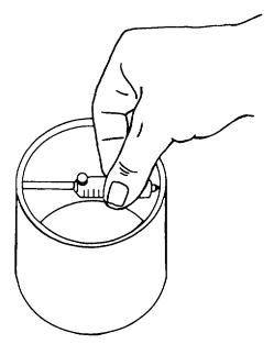
Figure 3-38. Using Inside Micrometer
