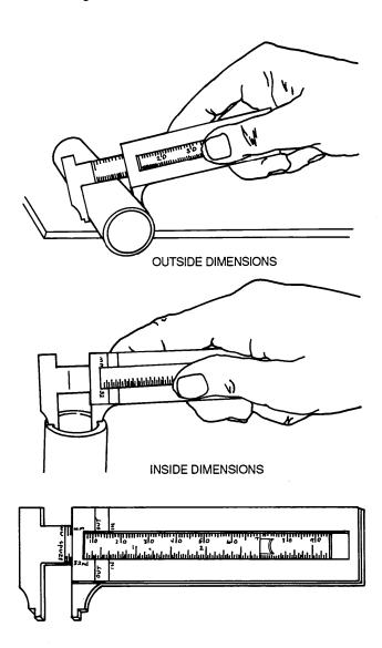
Figure 3-28. Slide Caliper
