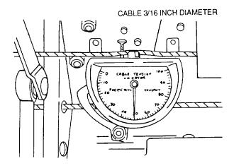
Figure 7-5. Using a Tensiometer
