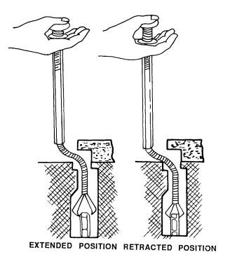
Figure 7-13. Flexible Mechanical Fingers
