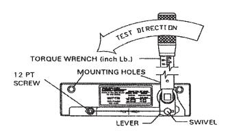
Figure 7-26. Torque Verification Fixture and Torque Wrench
