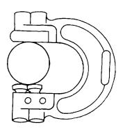
Figure 3-69. Correct NO-GO Dimension for Cylindrical Part
