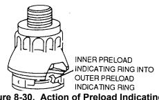
Figure 8-30. Action of Preload Indicating **Washers**
