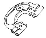
Figure 3-62. Snap Gauge for Checking Dimension Between Surfaces
