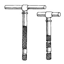
Figure 3-77. Telescoping Gauges
