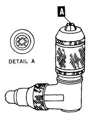
Figure 4-82. V-Grooves in Drill Jaws
