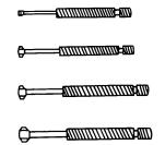
Figure 3-79. Small Hole Gauges
