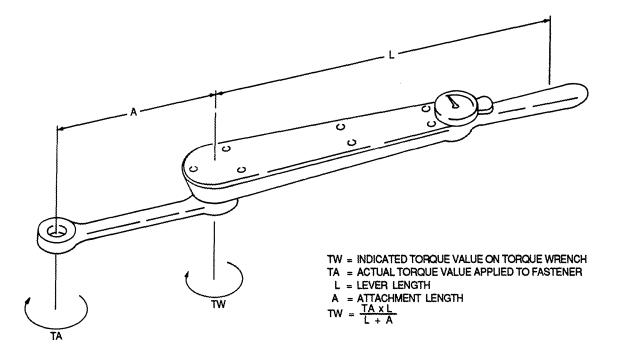
Figure 8-16. Nonconcentric Attachments to Torque Wrench
