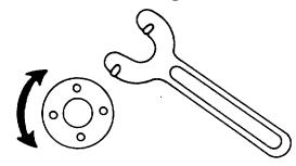
Figure 4-38. Face Pin Spanner Wrench
