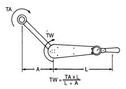
Figure 8-20. Angle Extension Torque Wrench Attachment
