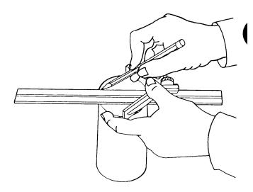
Figure 3-16. Marking Diameter of Cylinder
