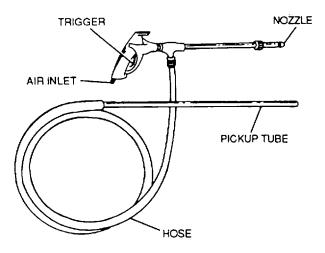
Figure 5-12. Cleaning Solvent Gun
