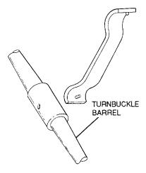
Figure 7-8. Turnbuckle Wrench
