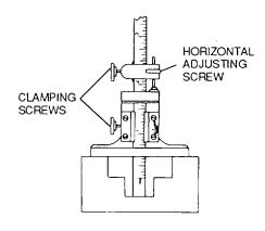
Figure 3-49. Vernier Depth Gauge
