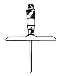
Figure 3-36. Depth Micrometer
