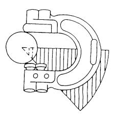
Figure 3-67. Placing Snap Gauge on Cylindrical Part
