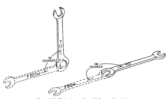
Figure 8-28. Tightening to 90- or 180-Degree Wrench Arc
