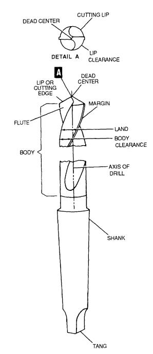
Figure 4-83. Typical Drill Bit
