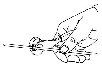
Figure 4-112. Cutting Wire
