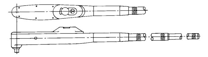
Figure 8-10. Type II, Style B Torque Wrench-Rigid Case with Indicator Dial, Presetting Torque Dial (Direct 8-4 Reading with Audible Signal)
