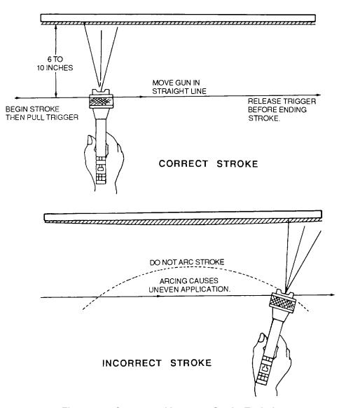
Figure 5-5. Correct and Incorrect Stroke Technique
