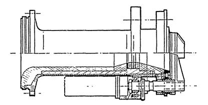
Figure 3-5. Flightweight Quickturn Test Nozzle
