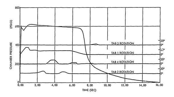
Figure 5-32. <u>Tab Actuation and Motor Chamber Pressure</u>, PFRT-05
