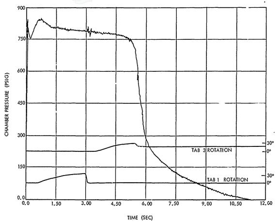
Figure 5-27. <u>Tab Actuation and Motor Chamber Pressure, PFRT-03</u>
