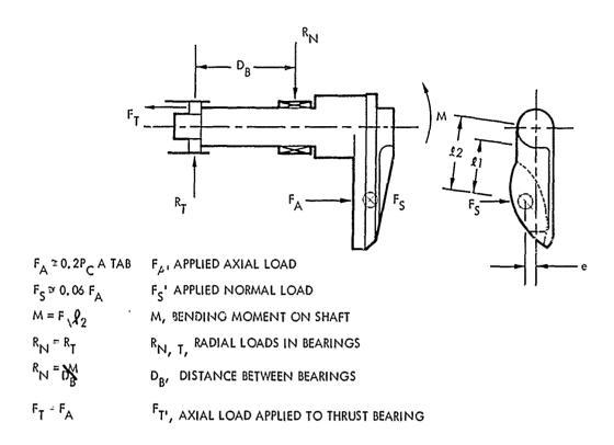
Figure 4-13. Free Body Force Diagram of the Tab Assembly
