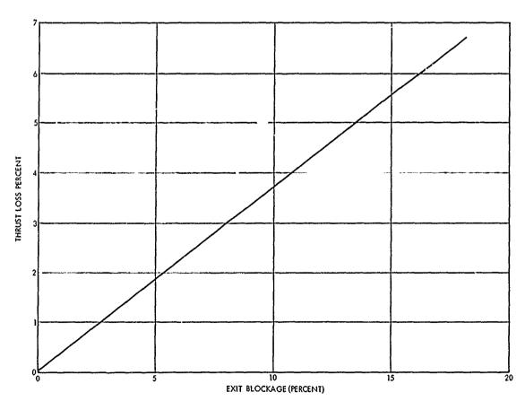
Figure 7-2. Thrust Loss as a Function of Nozzle Exit Area Blockage
