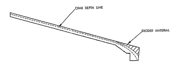
Figure 7-7. Nozzle Liner Char Depth
