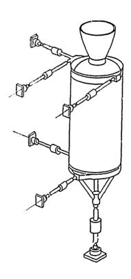
Figure 8-1. AFRPL Six-Component Char Motor Thrust Stand
