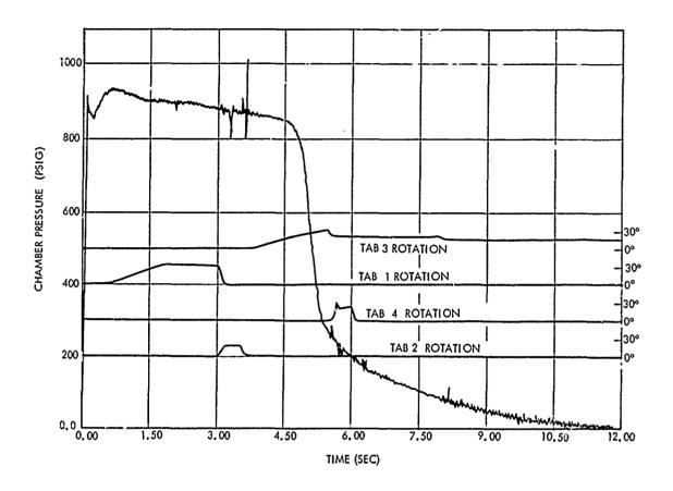
Figure 5-29 Tab Actuation and Motor Chamber Pressure PFRT-04
