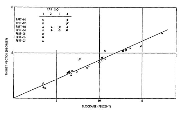
Figure 7-1. Thrust Vector Angle vs. Nozzle Exit Area Blockage
