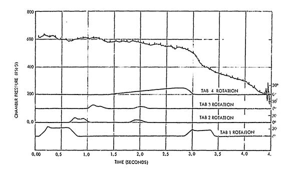
Figure 5-4. Motor Chamber Pressure and Tab Actuation, PI-1
