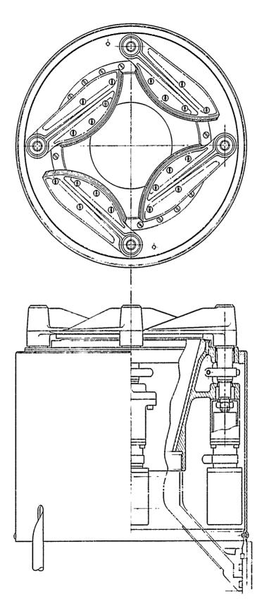
Figure 4-1. Jet Tab TVC System for BGM-34C
