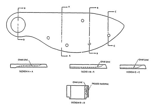
Figure 7-8. Tab Insulator Char Depth
