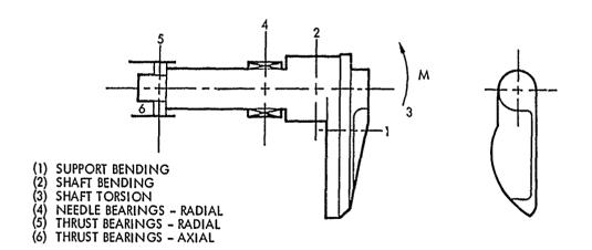
Figure 4-14. Critical Stress Areas for Jet Tab
