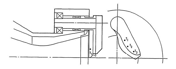
Figure 8-3. Thermocouple Location
