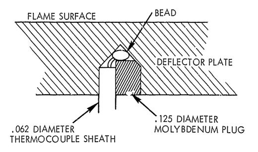
Figure 8-4. Buried Thermocouple
