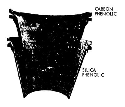
Figure 5-20. <u>Nozzle Exit Liner Erosion Comparison</u>
