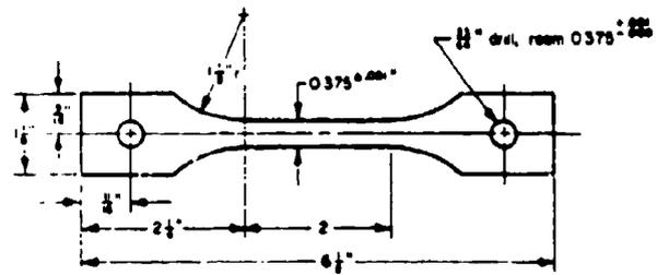
**FIGURE 64. SHEET CREEP - AND STRESS-RUPTURE SPECIMEN**
