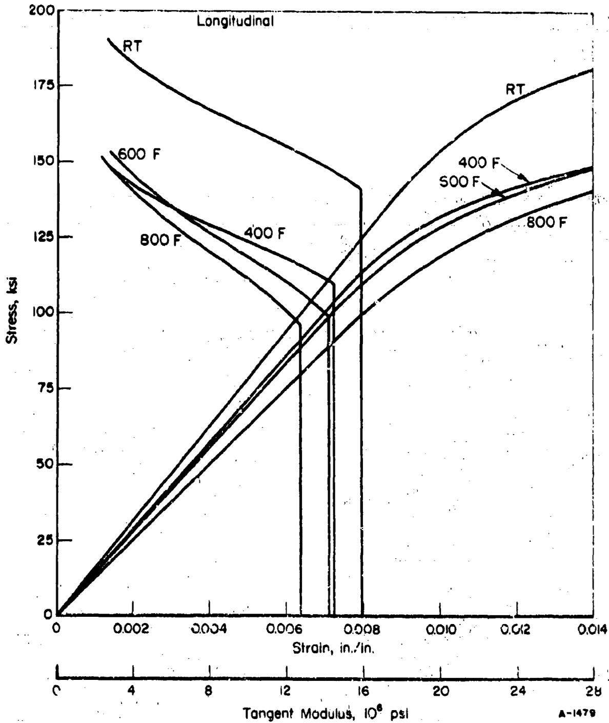
FIGURE 34. TYPICAL COMPRESSIVE STRESS-STRAIN AND TANGENT-MODULUS CURVES AT TEMPERATURE FOR SOLUTION-TREATED AND AGED T1-8Mo-8V-2Fe-3Al SHEET (LONGITUDINAL)
