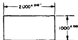
FIGURE 75. THERMAL-EXPANSION SPECIMEN
