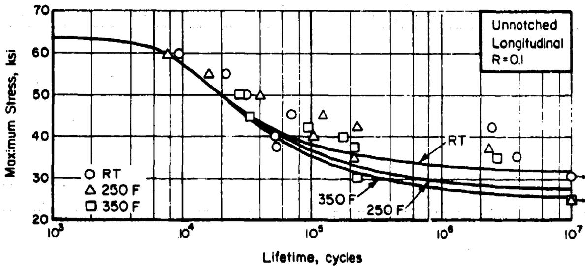
FIGURE 8. AXIAL LOAD FATIGUE BEHAVIOR OF UNNOTCHED X2048-T851 PLATE (LONGITUDINAL)
