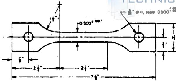
**FIGURE 60. SHEET AND THIN-PLATE TENSILE SPECIMEN**
