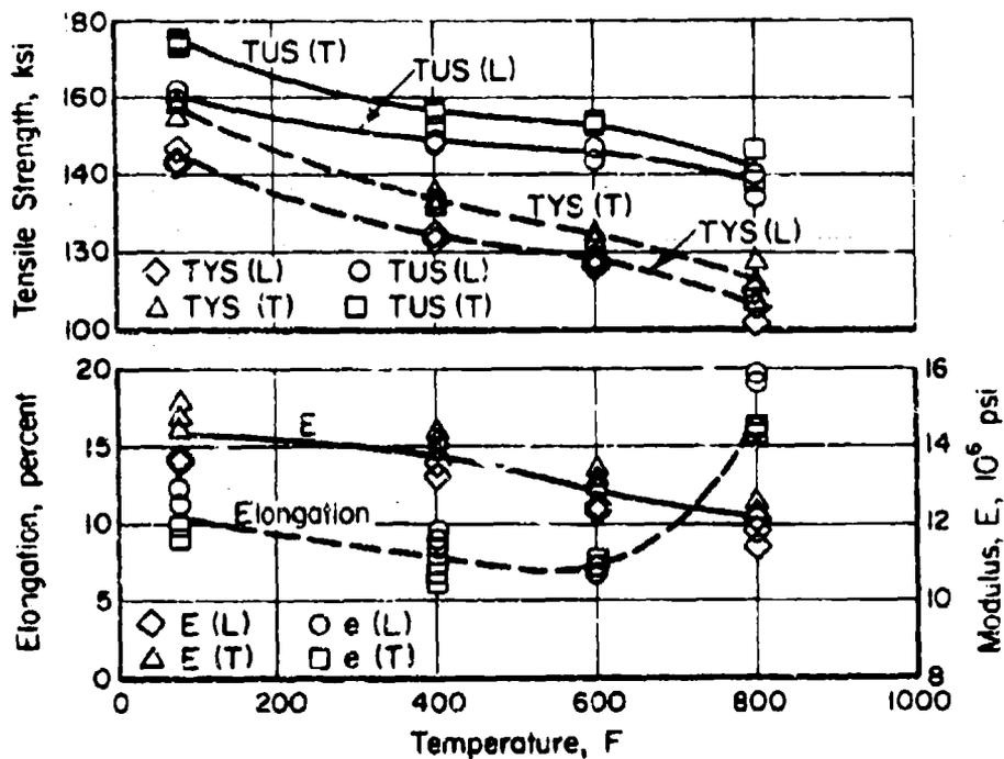
FIGURE 36. EFFECT OF TEMPERATURE ON THE TENSILE PROPERTIES OF SOLUTION-TREATED AND AGED Ti-8Mo-8V-2Fe-3Al SHEET
