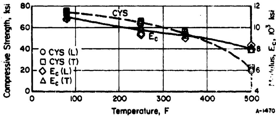
FIGURE 17. EFFECT OF TEMPERATURE ON THE COMPRESSIVE PROPERTIES OF 7050-T73651 PLATE
