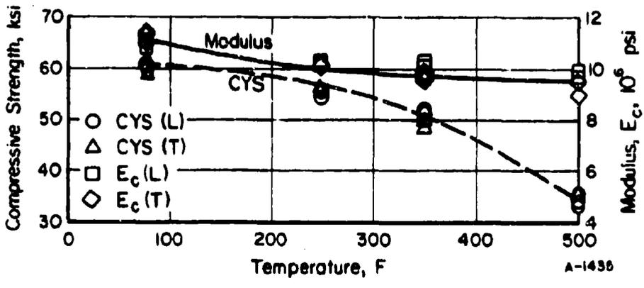
FIGURE 7. EFFECT OF TEMPERATURE ON THE COMPRESSIVE PROPERTIES OF X2048-T851 PLATE
