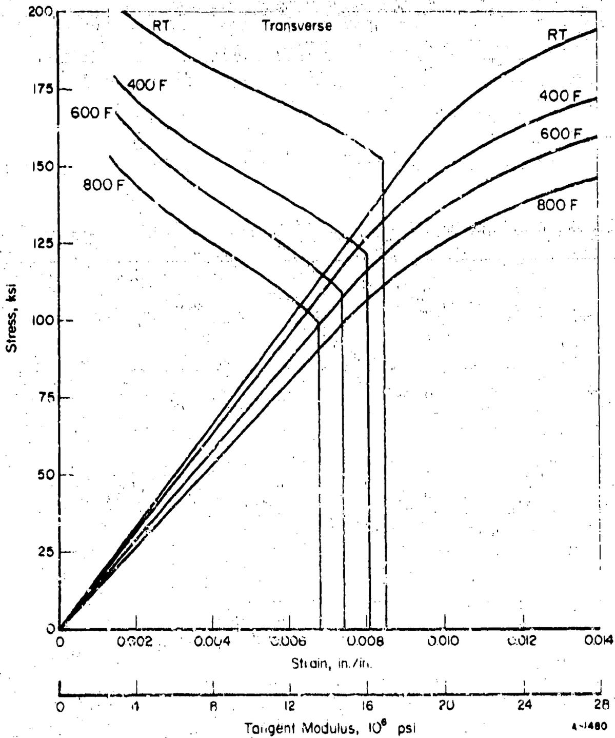
FIGURE 35. TYPICAL COMPRESSIVE STRESS-STRAIN AND TANGENT-MODULUS CURVES AT TEMPERATURE FOR SOLUTION-TREATED AND AGED TI-6AL-4V-2FE-2AL SHEET (TRANSVERSE)
