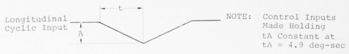
Figure 25. Effect of control input magnitude and rate on main rotor flapping.
