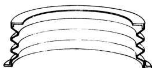
B-11 CORRUGATED DIAPHRAM SCISSORS WT - 9 LB COST - $1200
