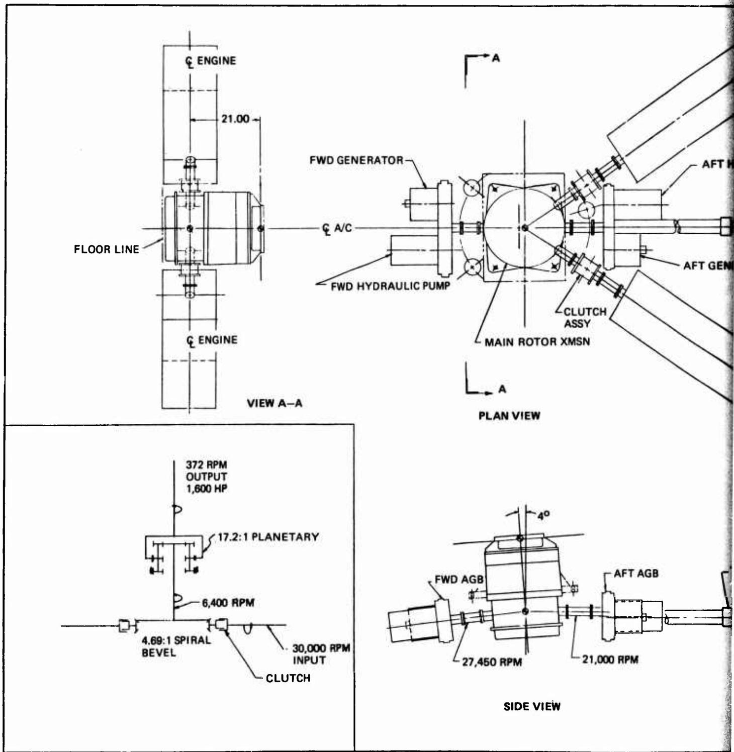
Figure 5. Free Planet Version for Direct Engine Input.
