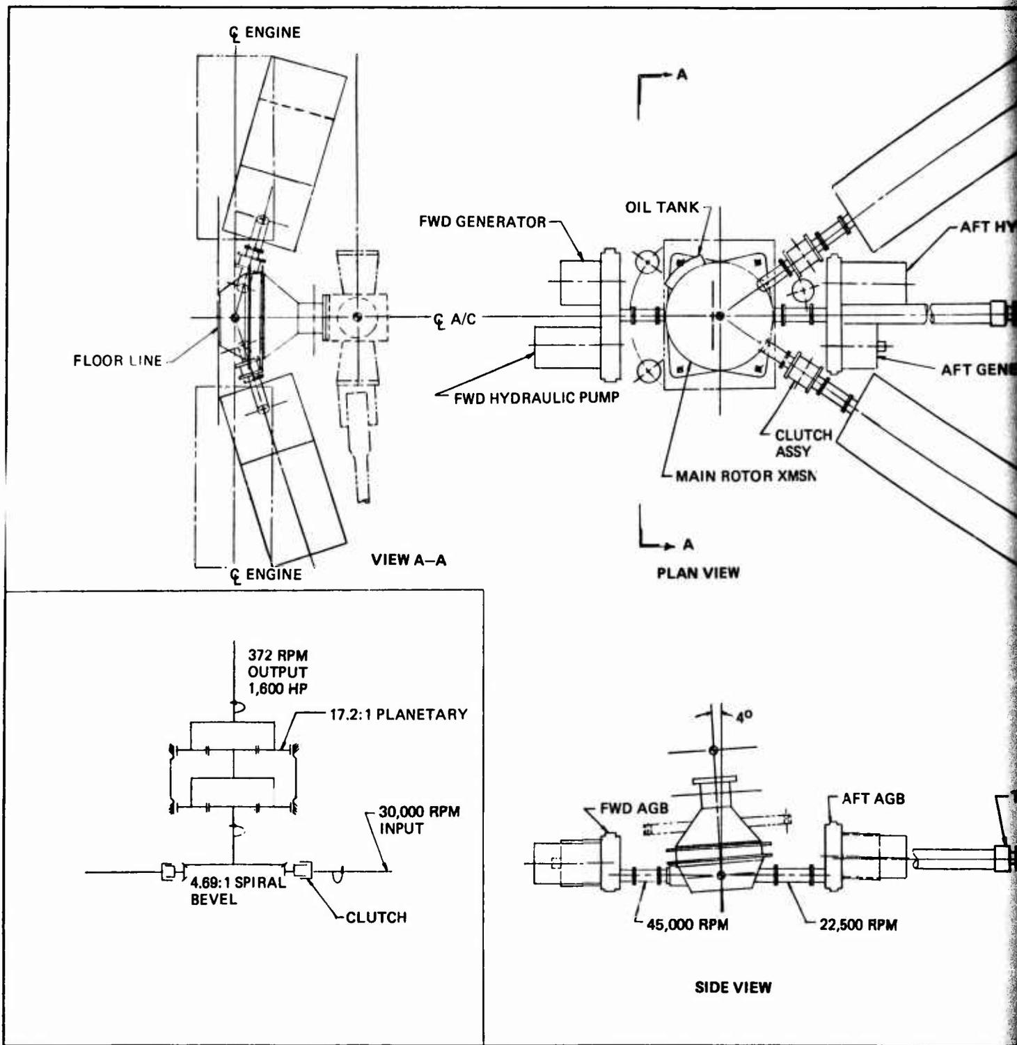
Figure 4. Conventional Version for Direct Engine Input.
