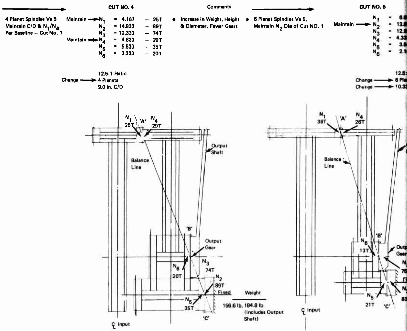
Figure 12. Free Planet Study Parametric Study (1,604 hp, 372 rpm).
