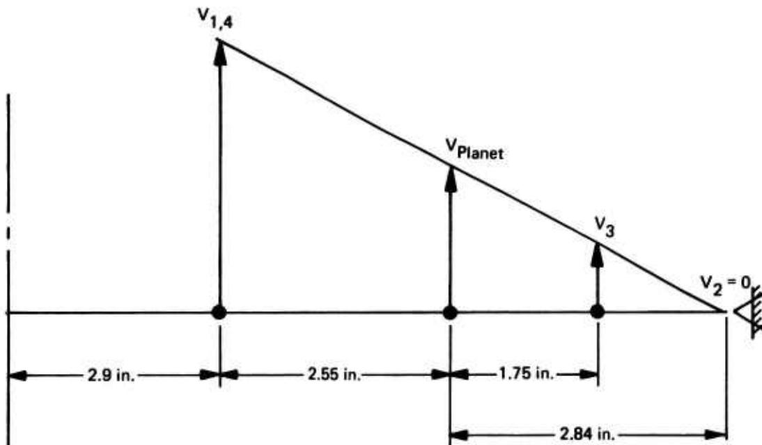
$$V_{1,4} = 4,620 \text{ rpm} \times 2.9$$
