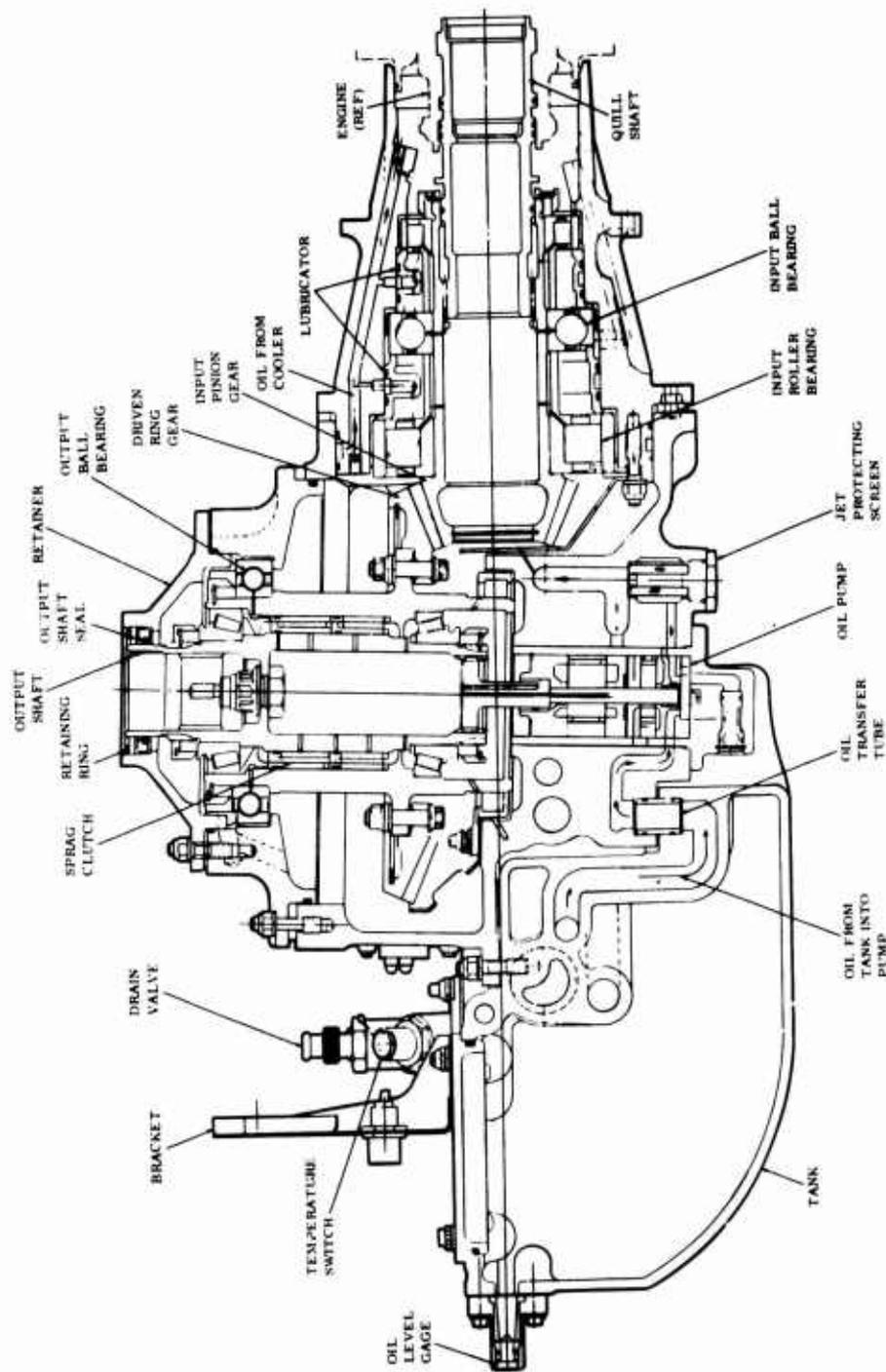
Figure 6. Engine Transmission with 2.7:1 Reduction.
