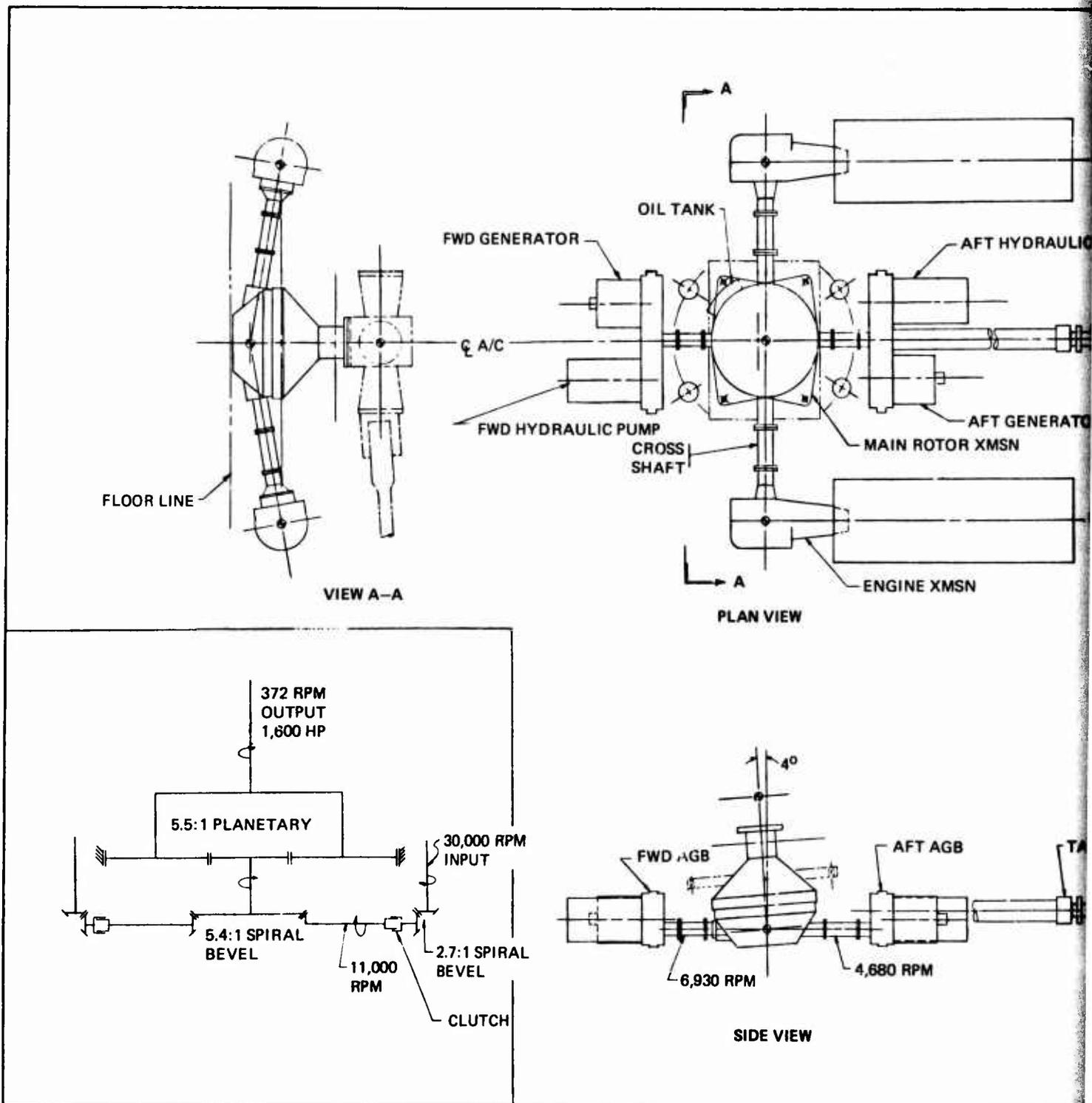
Figure 2. Conventional Transmission - Configuration No. 1.
