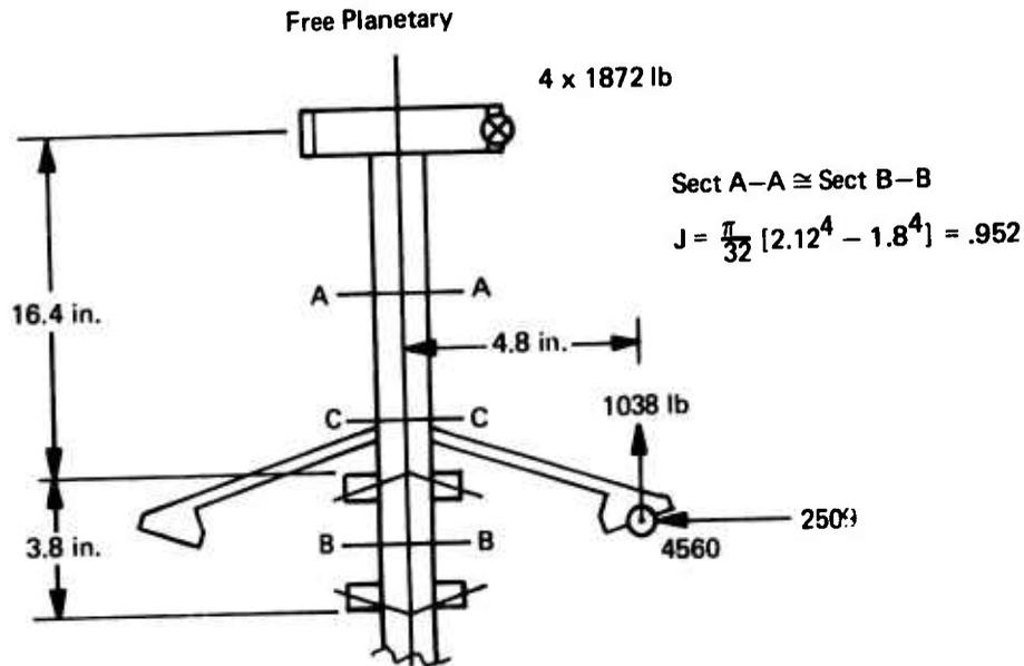
$$\text{Shaft Torsion } f_s = \frac{Tc}{J} = \frac{21,870 \times 1.06}{.952} = 24,350 \pm 2,922 \times K_t$$
