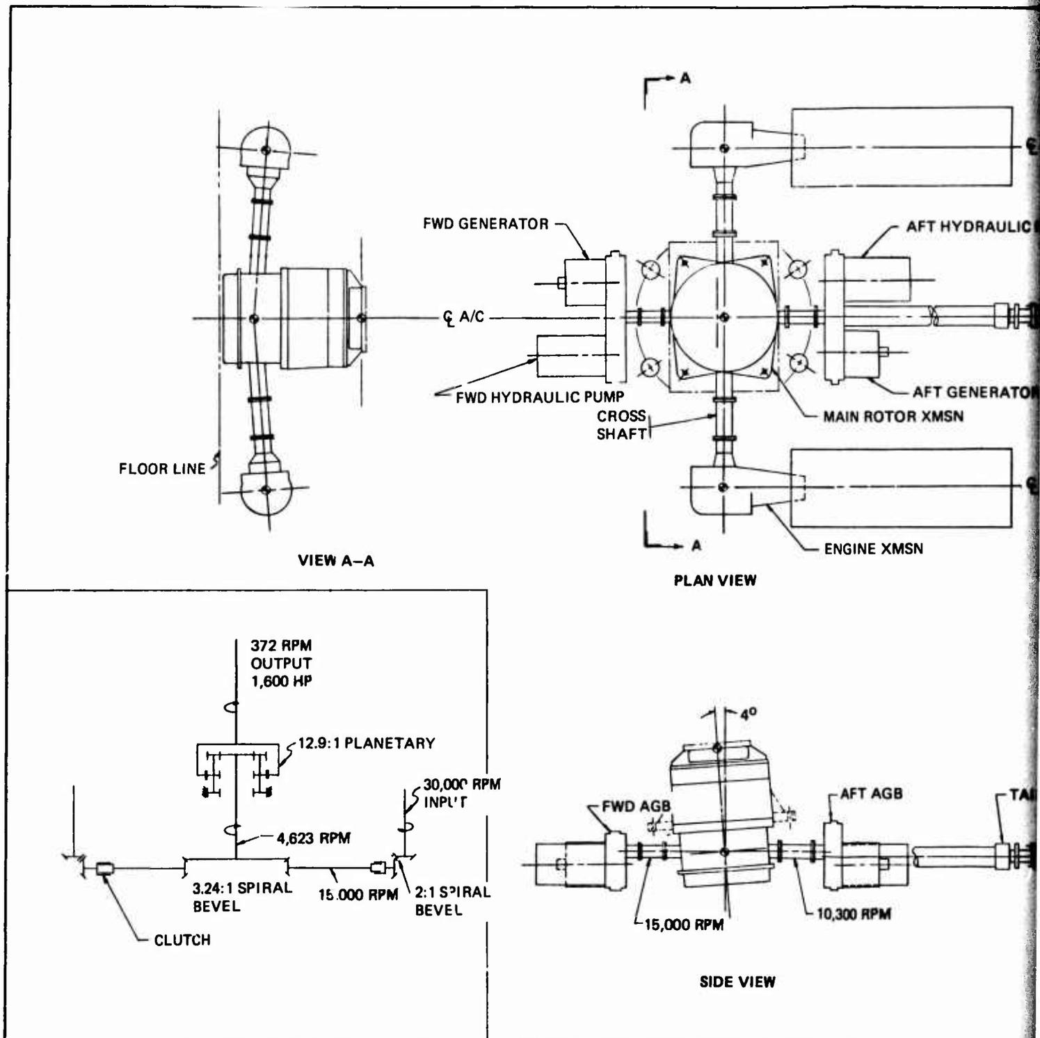
Figure 3 . Free Planet Version of Configuration No. 1.
