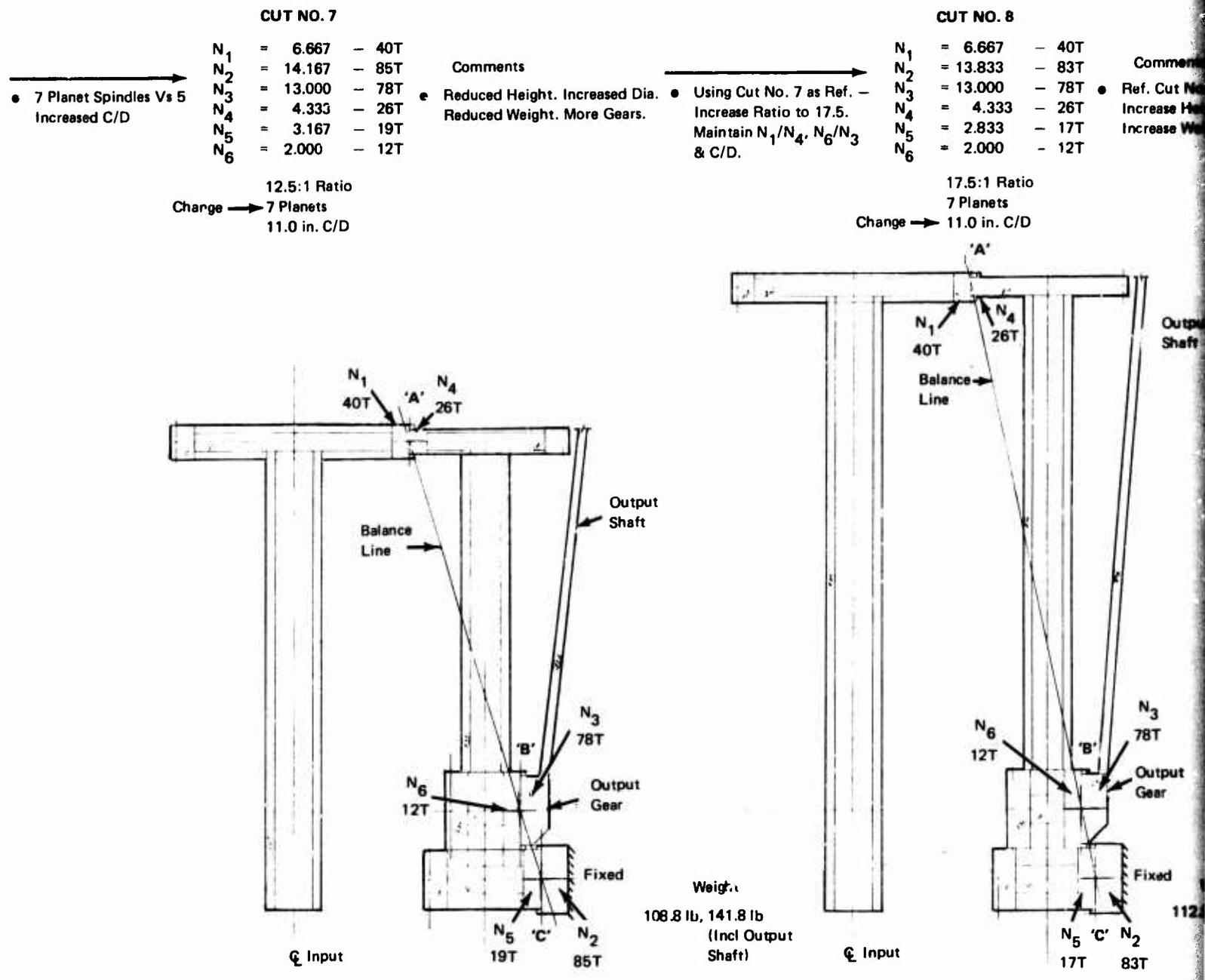
Figure 13. Free Planet Study Parametric Study (1,604 hp, 372 rpm).
