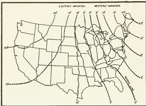
Figure 99—This diagram shows the agonic and isogonic lines of variation.
