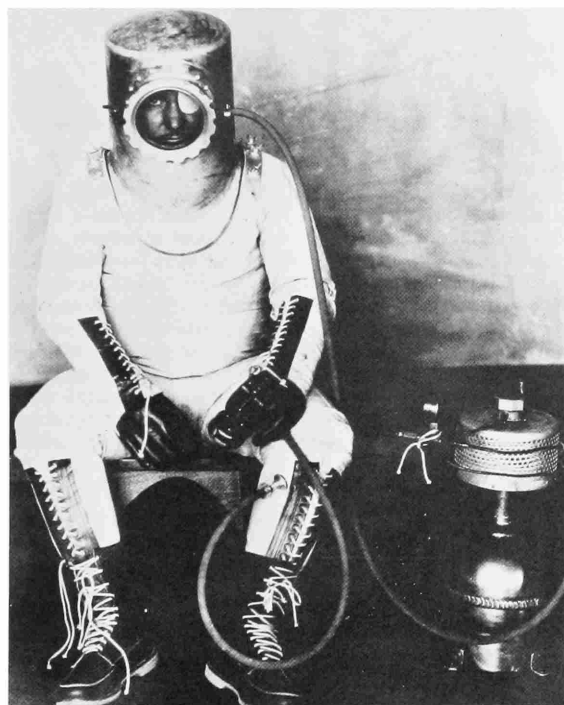
FIGURE 75. —The complete pressure-suit ensemble used by Wiley Post for inflight studies. Liquid oxygen is in the spherical tank. The liquid-to-gas conversion unit is attached to the top of the tank. The oxygen-inflow tube leads from the converter to the left side of the helmet. In Post's left hand is the outflow pressure-monitoring gauge. A second gauge on the oxygen converter gives inflow pressure information. Photograph made at Wright Field, August 27, 1934. (Courtesy U.S. Air Force.)
