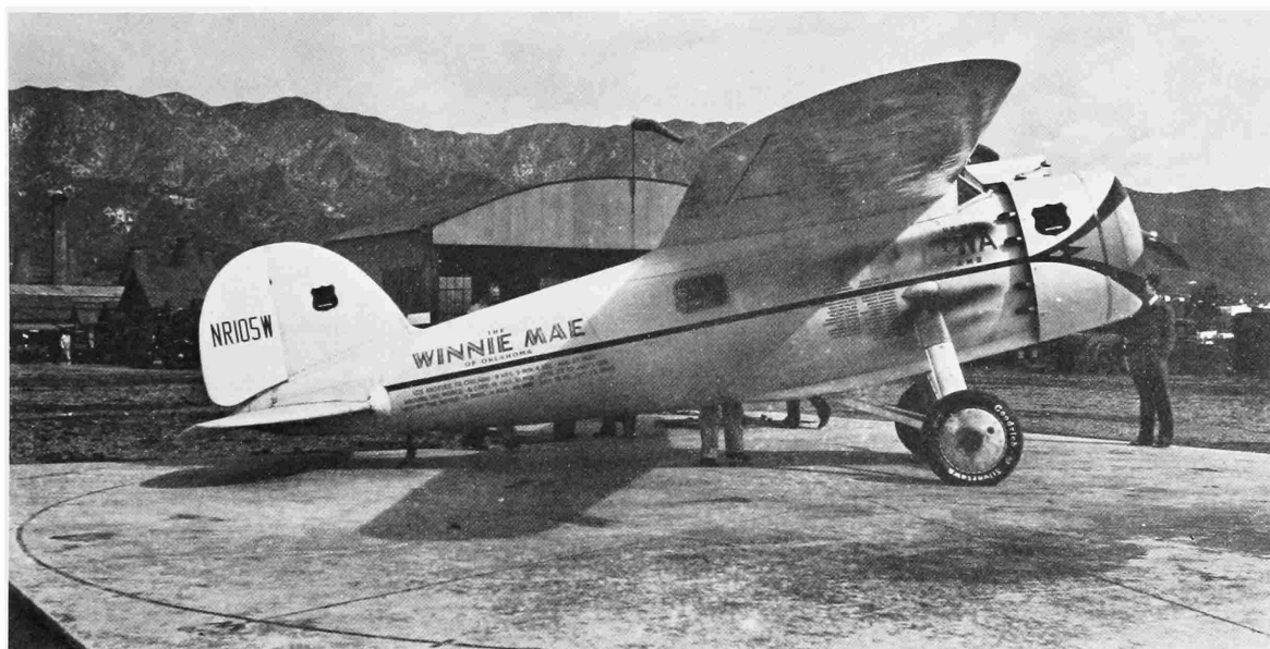
FIGURE 105.—The Winnie Mae without droppable gear (but with the belly skid in place) is shown at Burbank after a test flight. The dark exhaust marks on the fuselage were not unusual following a long flight. (Courtesy Phillips Petroleum.)
