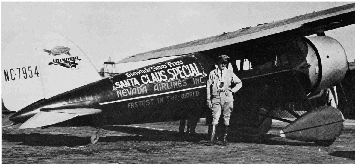
FIGURE 14.—In 1929 F. C. Hall sold the first Winnie Mae (NC 7954) back to Lockheed, who in turn sold the aircraft to Nevada Airlines. The Vega was equipped with a N.A.C.A. cowling and wheel pants, and was renamed “Sirius.” “Captain” Roscoe Turner (later “Colonel”) flew the aircraft in the 1929 air races, coming in third in the free-for-all speed contest, at an average speed of 163.44 miles-per-hour (mph), behind Doug Davis, first, (194.90 mph in a Travel Air) and R. G. Breen, second, (186.84 mph in a Curtiss P-3-A). (Courtesy Lockheed Aircraft Company.)
