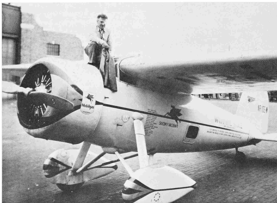
FIGURE 65.—This view shows the Winnie Mae at Floyd Bennett Field with a battered wing leading edge and dented wheel pants and cowling, illustrating the scars of the 1933 solo world flight. The two steps for mounting or climbing down from the cockpit are extended. The steps could be moved in or out from either inside the cockpit or outside the aircraft. An unusual feature is the tail wheel, which Post did not prefer. His traditional tail skid gave much more stability with respect to ground handling during landing roll-outs, especially in crosswinds at short fields. However, some "grass-strip" airport operators objected to tail skids, due to the "furrowing" that was produced. The top of each wheel pant is metal clad to withstand foot-pressure without damage to the finish. (Courtesy Mobil Oil Corporation.)
