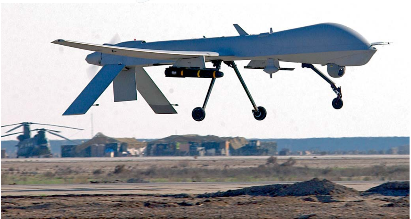
An MQ-1 Predator unmanned aerial vehicle lands at a base in Southwest Asia. USAF/ Staff Sgt Suzanne M Jenkins.
