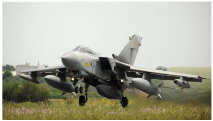
An RAF Tornado takes off for a sortie with a RAPTOR imaging pod. RAPTOR's imaging capabilities meant that such missions were a key part of NATO's intelligence gathering operations. Crown copyright/Sgt Pete Mobbs photo.
