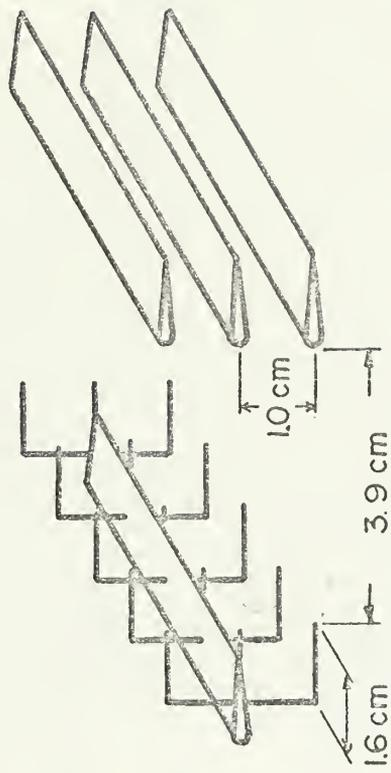
FIGURE 4. DETAIL OF ELECTRODES
