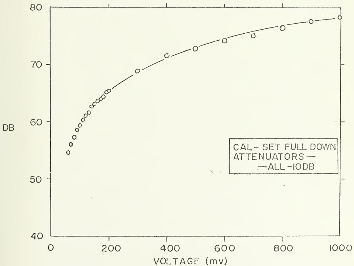
FIGURE 12. CALIBRATION OF RMS DETECTOR
