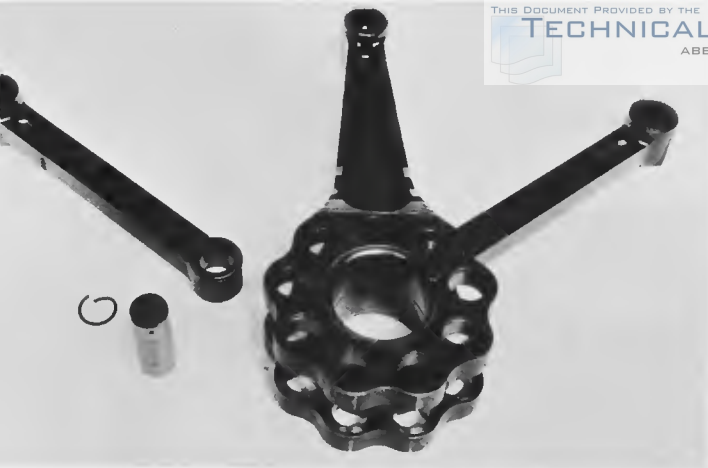
Figure 25.—Master and link connecting rods. U.S. Navy test, 1931. (Smithsonian photo A48323A.)
