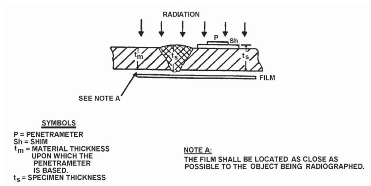
Figure 3-8. Examples of  $T_m$ ,  $T_s$ , and Penetrator Placement: Single Wall, Weld Reinforcement, No Back-Up Strip.
