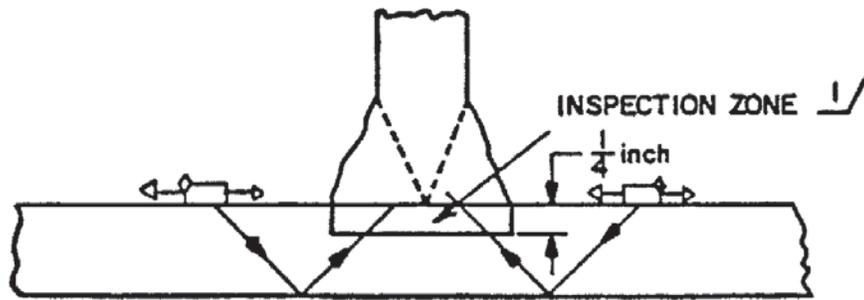
1/ THE INSPECTION ZONE MAY BE EXPANDED AS NECESSARY WITHIN THE PLATE OR WELD. THE SAME SCANNING PROCEDURES MAY BE APPLIED TO PARTIAL PENETRATION TEE WELDS.
