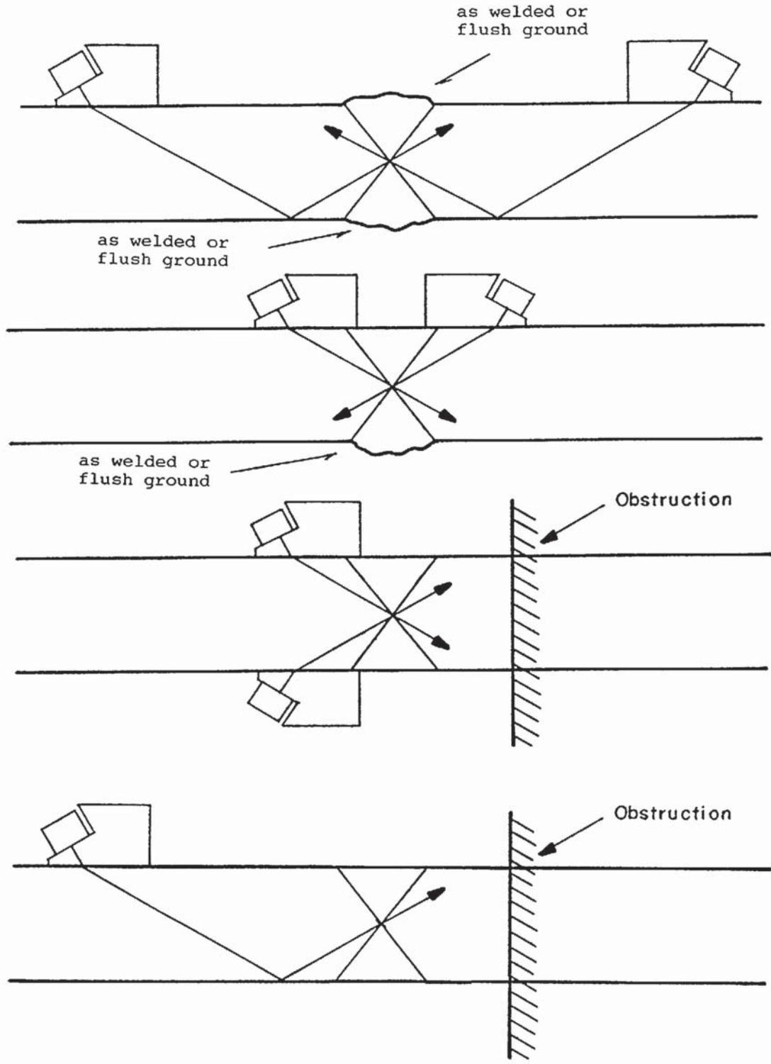
Figure 6-3. Example Full Coverage Scanning Techniques for Butt Welds.
