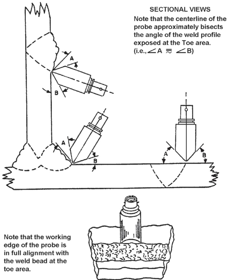
Figure 7-1. Recommended Probe-To-Weld Attitude for Eddy Current Standardization and Scanning Operations.
