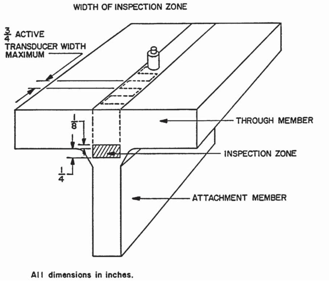
Figure 6-9. Scanning Procedure for Detection of Lack of Penetration in Tee Welds.
