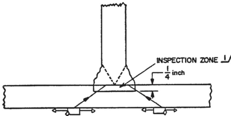
1/ THE INSPECTION ZONE MAY BE EXPANDED AS NECESSARY WITHIN THE PLATE OR WELD. THE SAME SCANNING PROCEDURES MAY BE APPLIED TO PARTIAL PENETRATION TEE WELDS.
