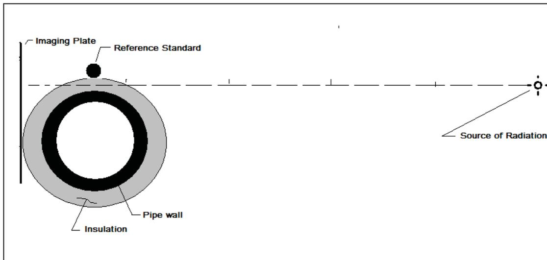
**Figure A-1. Alignment of Radiation Source and Imaging Plate.**
