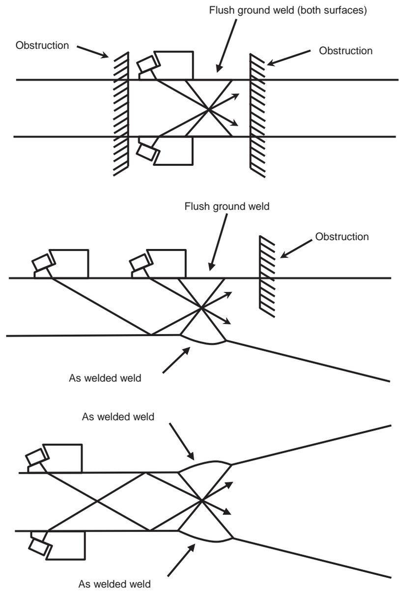
Figure 6-4. Example One-Directional Coverage Techniques for Butt Welds.
