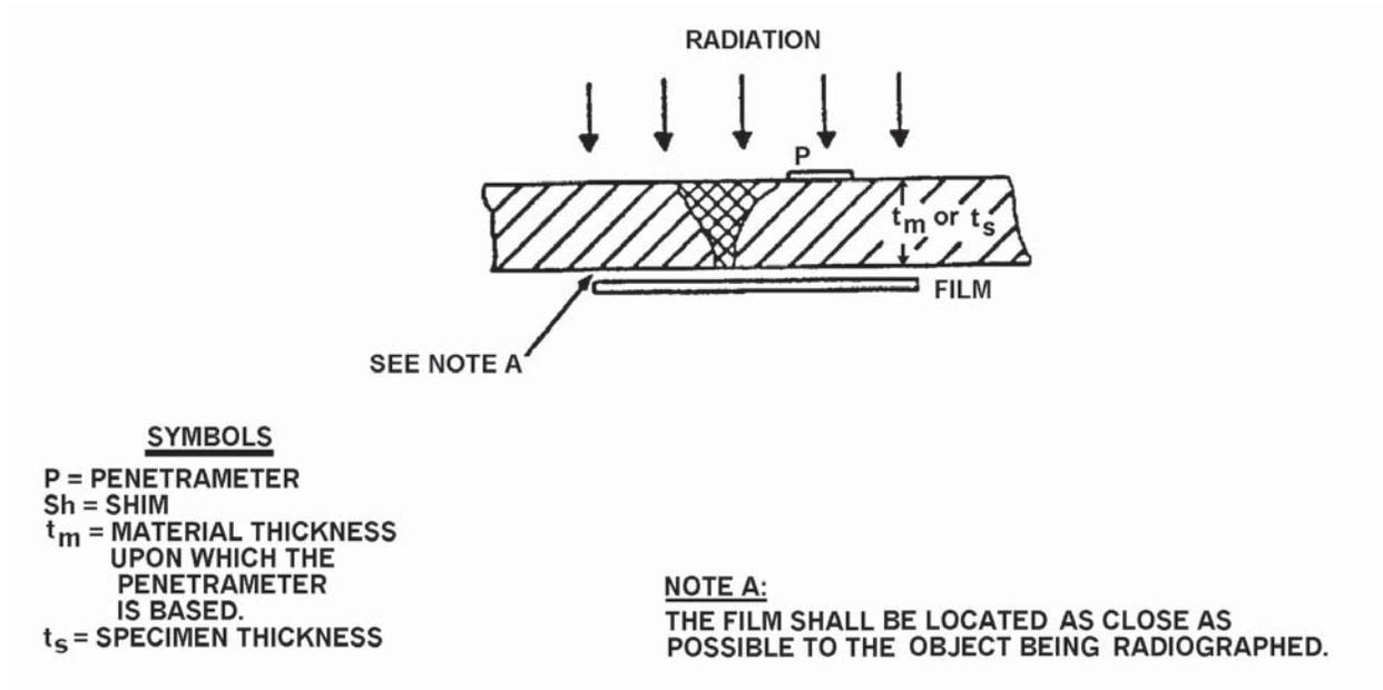
Figure 3-7. Examples of  $T_m$ ,  $T_s$ , and Penetrator Placement: Single Wall, No Reinforcement, No Back-Up Strip.
