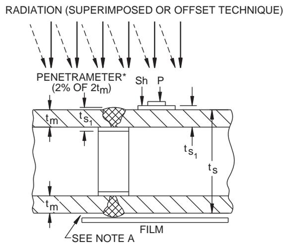
\* 2% OF  $2t_m$  FOR 2-LEVEL, 1% OF  $2t_m$  FOR 1-LEVEL, AND 4% OF  $2t_m$  FOR 4-LEVEL RADIOGRAPHY.
