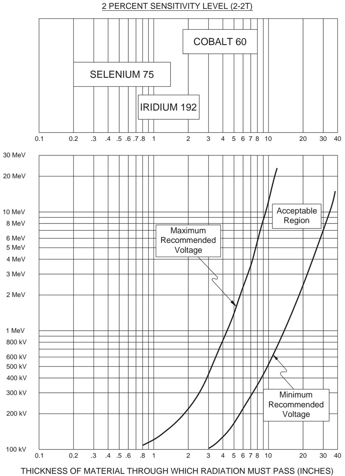
**Figure 3-3. Recommended X-ray Voltage Settings and Radioisotope Sources to Be Used with Various Aluminum, Magnesium and Similar Alloys.**
