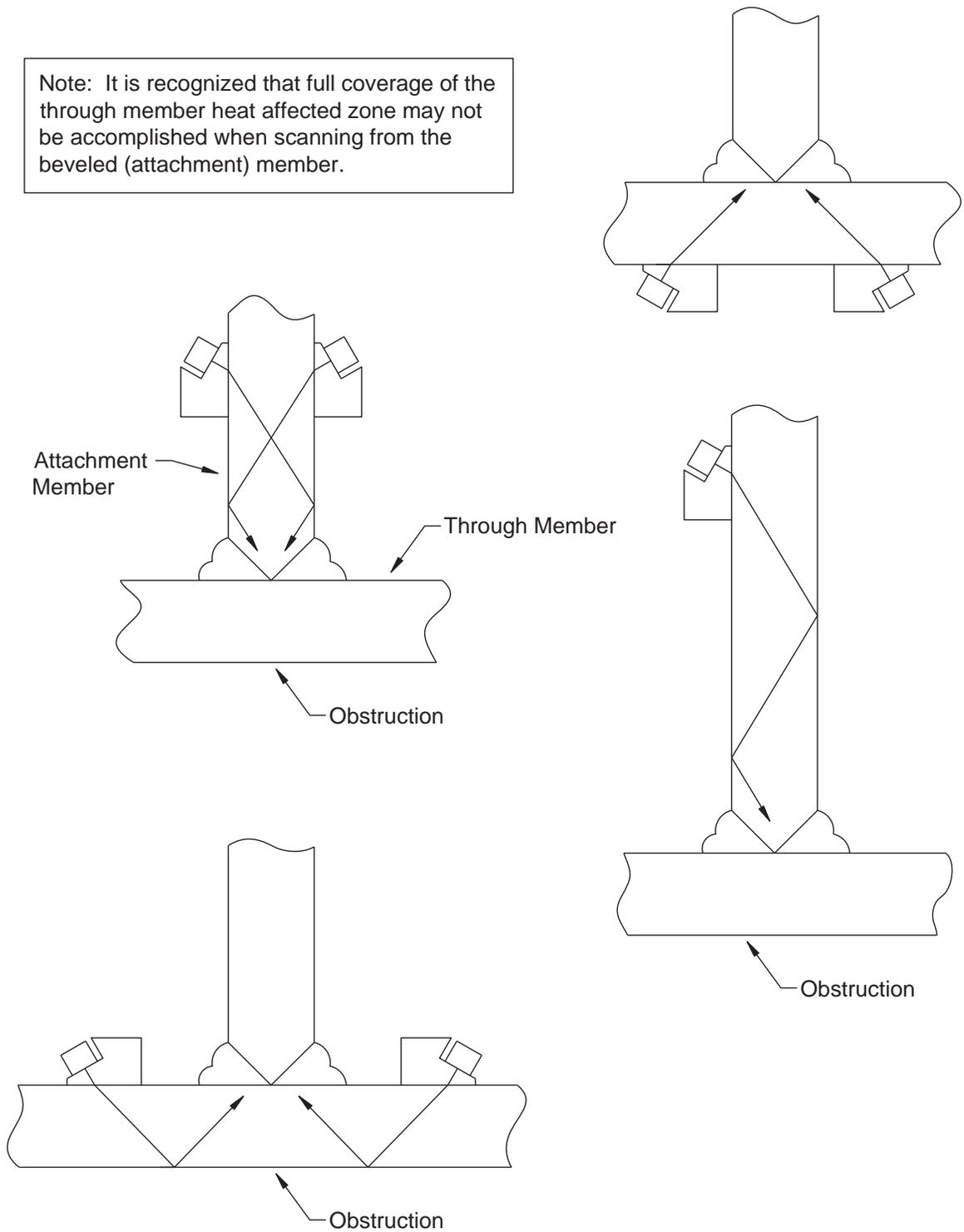
Figure 6-6. Example Scanning Techniques for Tee Welds.
