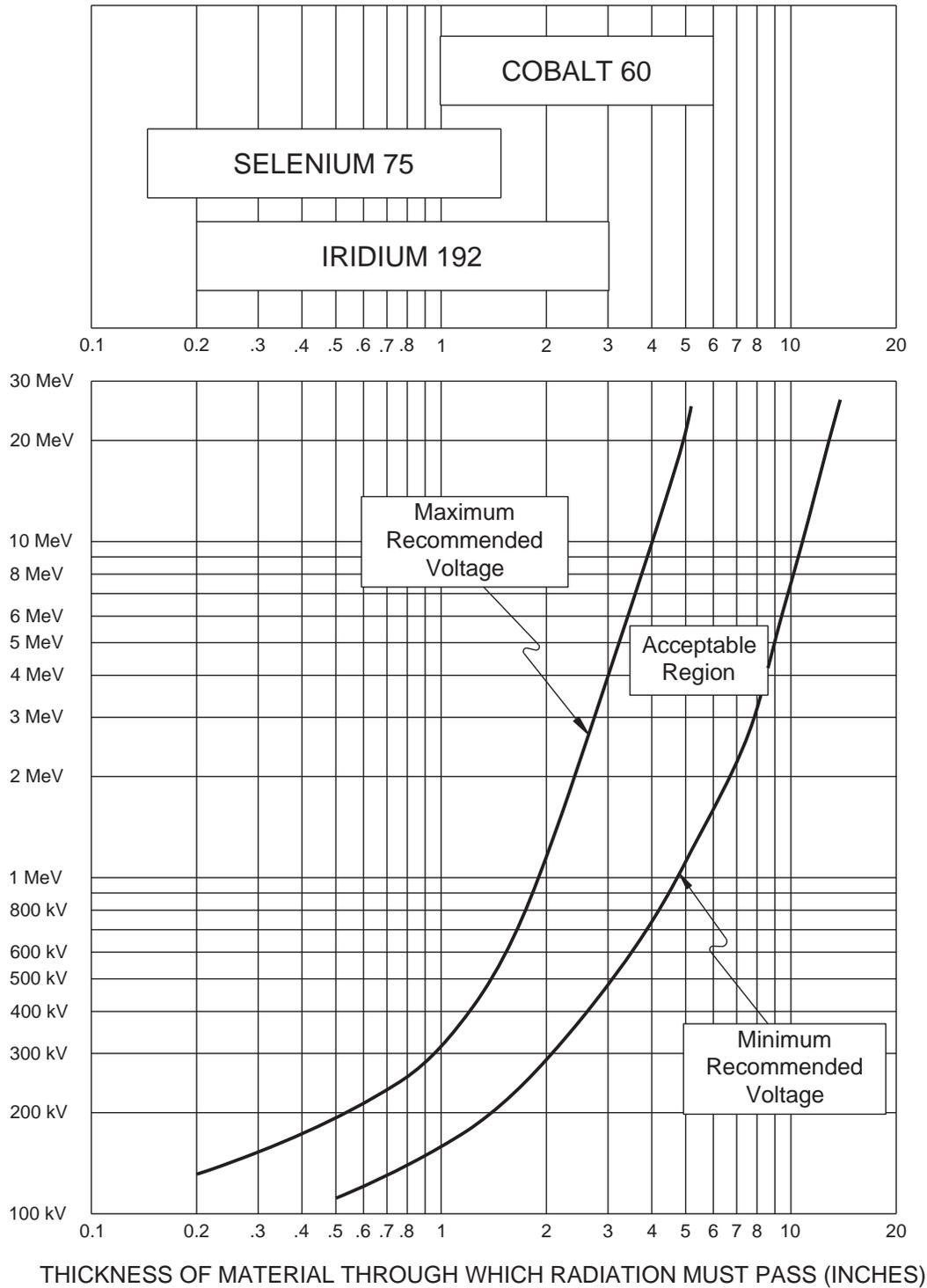
Figure 3-2. Recommended X-ray Voltage Settings and Radioisotope Sources to Be Used with Various Copper-Base and Similar Alloys.
