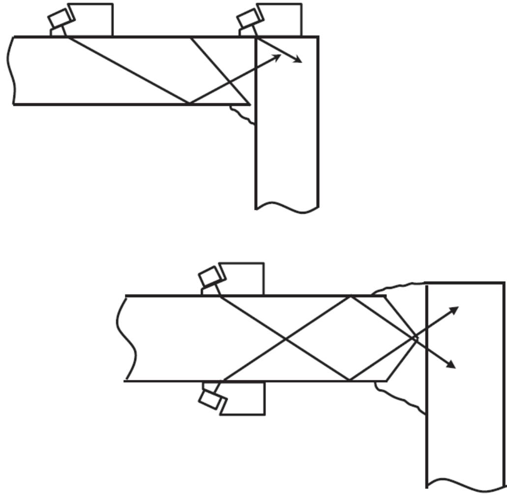
Figure 6-5. Example Scanning Techniques for Corner Welds.
