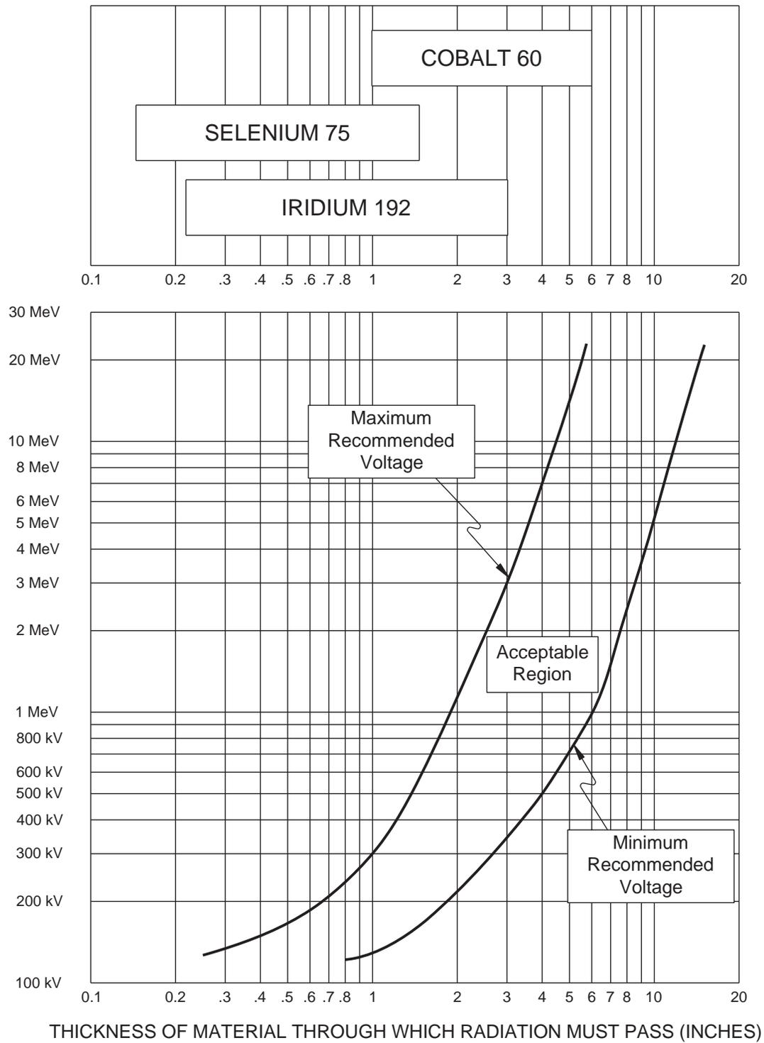
**Figure 3-1. Recommended X-ray Voltage Settings and Radioisotope Sources to Be Used with Various Steel and Similar Alloys.**
