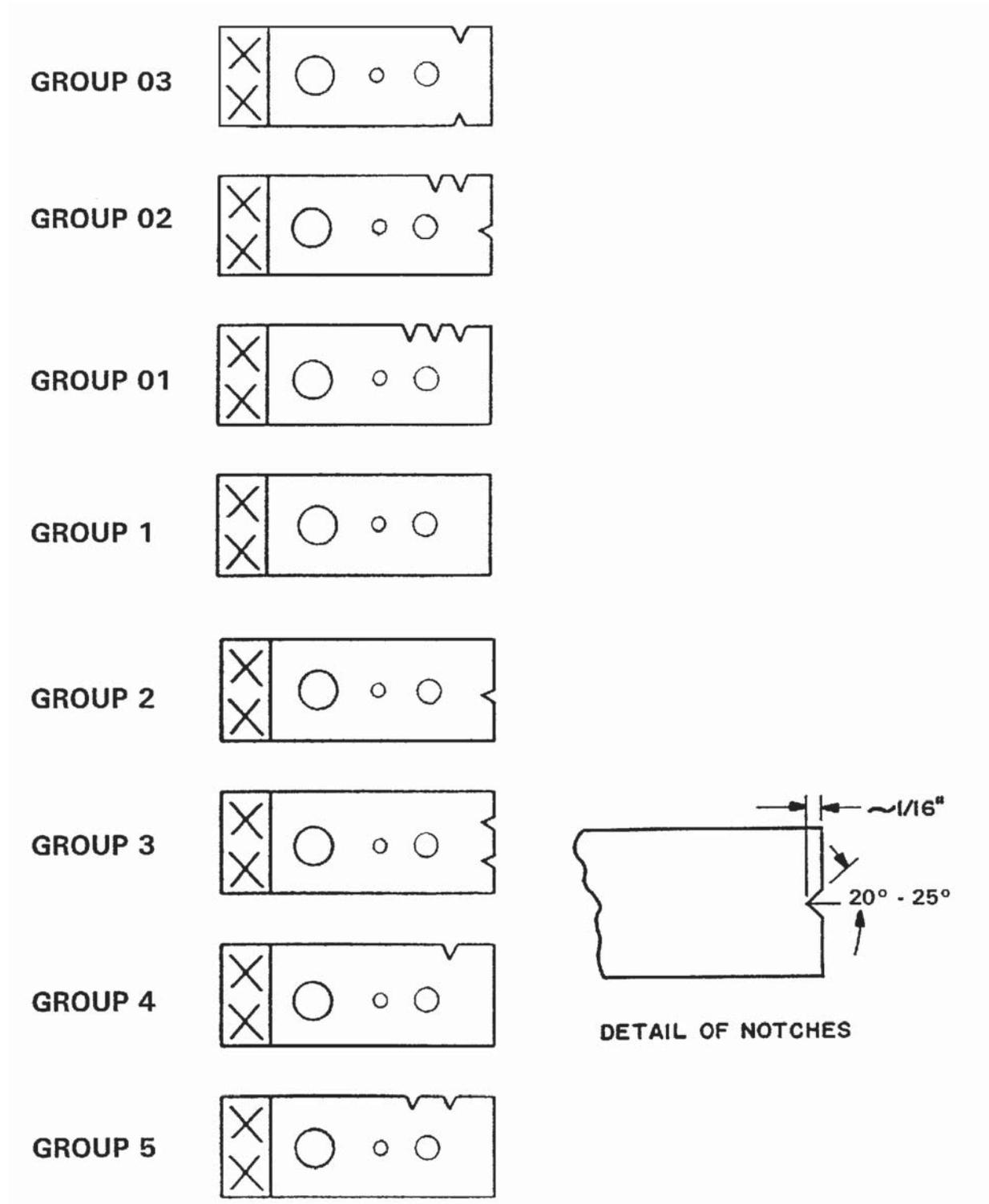
Figure 3-6. Penetrameter Identification Notching.
