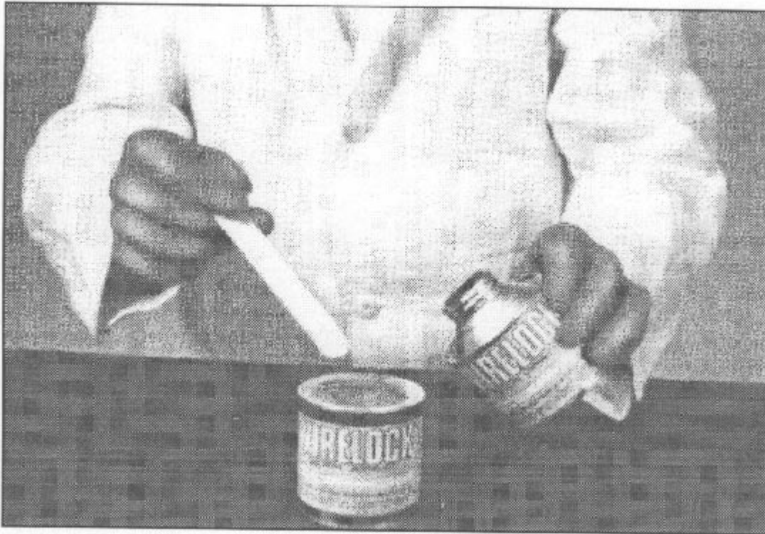
Figure 613-1-27A. Proper Vessel and Wooden Paddle Used in Mixing.
