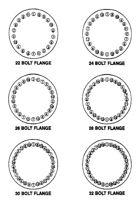
Figure 075-4-4. Multi-Jackbolt Tensioner Jackbolt Tightening Sequences, 22 or More Jackbolts
