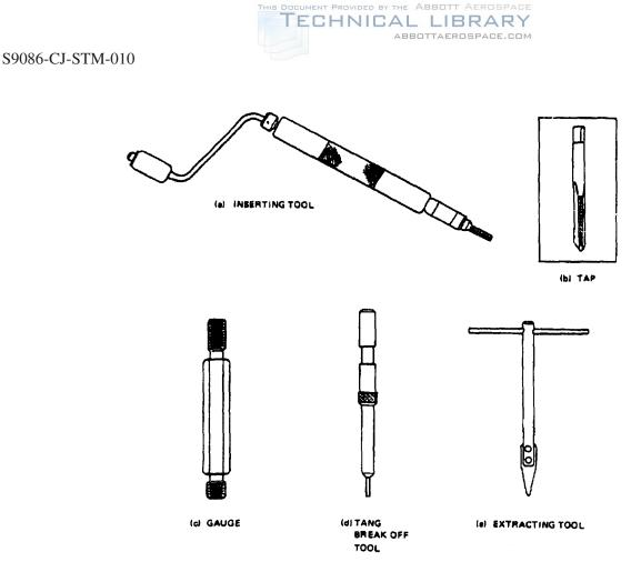
Figure 075-2-3. Typical Helical Coil Insert Repair Tools
