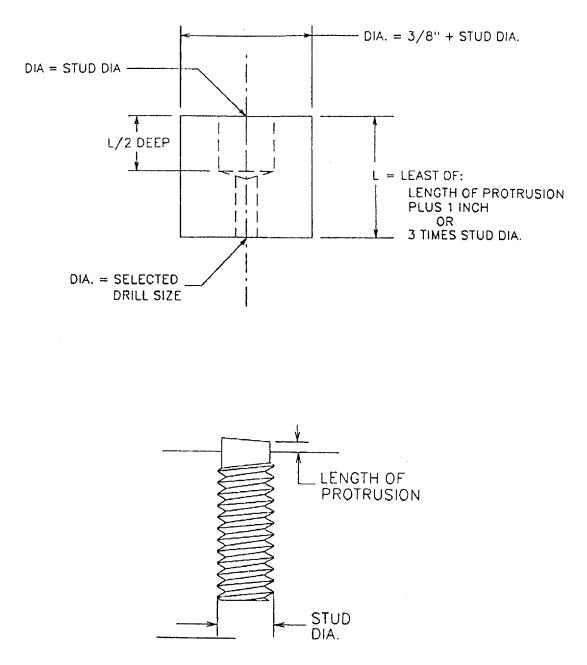
Figure 075-9-1. Broken Stud Drill Guide Removal Device
