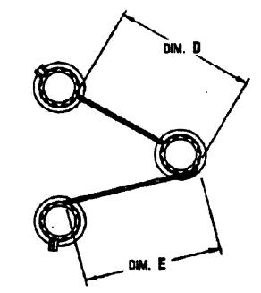
FOR THREE BOLT PATTERNS DIM. A - DIM. D + DIM. E
