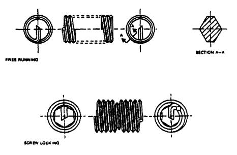
Figure 075-2-2. Typical Thin Wall Inserts
