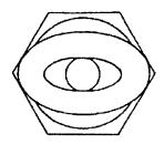
Figure 075-5-4. Distorted Collar Nuts.
