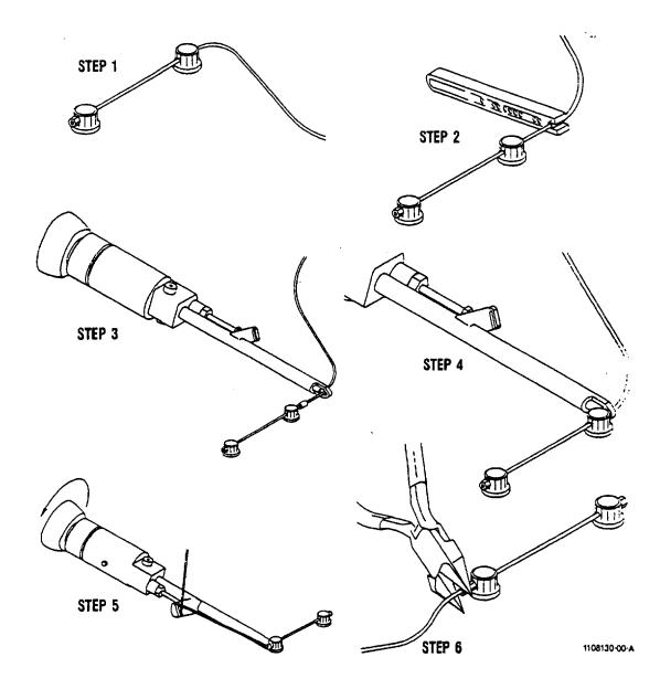
Figure 075-5-13. Safety Cable Procedure (Sheet 2 of 2) CAUTION
