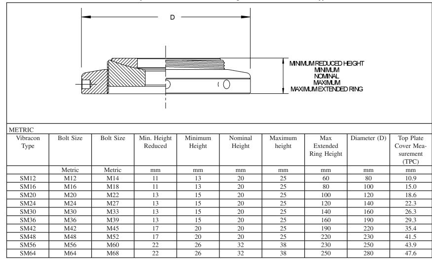
Table 075-2-28 Vibracon Adjustable Chock – Low Profile Configurations, Grade A/B Shock Applications, METRIC
