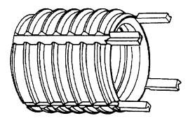
Figure 075-2-14 Key Locked Insert (Typical)
