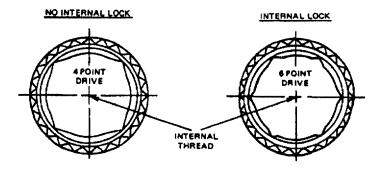
Figure 075-2-1. Helical Coil Inserts
