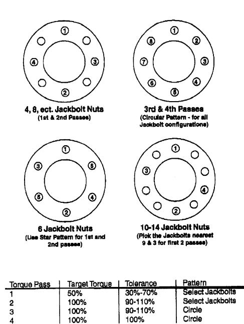
Figure 075-4-3. Multi-Jackbolt Tensioner Jackbolt Tightening Sequences, 14 or Fewer Jackbolts
