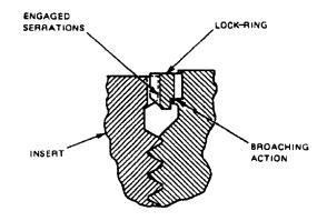
Figure 075-2-13 Ring Locking Principle
