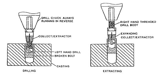
Figure 075-9-2. Broken Bolt Extractor.
