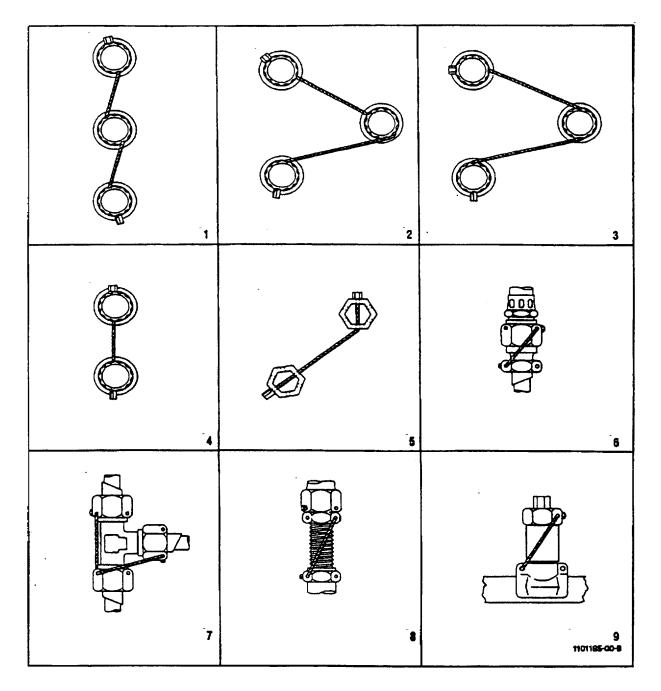
Figure 075-5-14. Safely Cable Patterns (Sheet 1 of 2)
