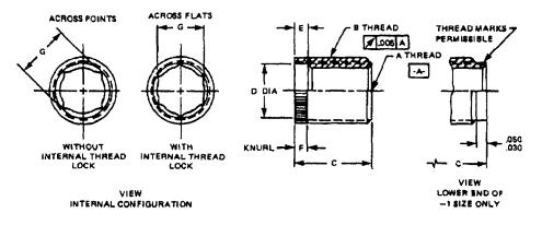
Figure 075-2-15 Thin Wall Insert
