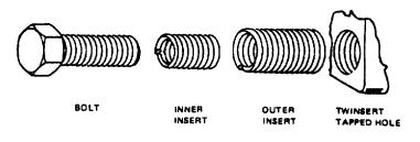
Figure 075-2-4. Heli-Coil Twinsert Assembly
