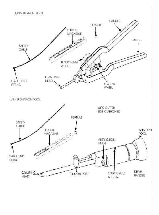
Figure 075-5-11. Safety Cable System Components
