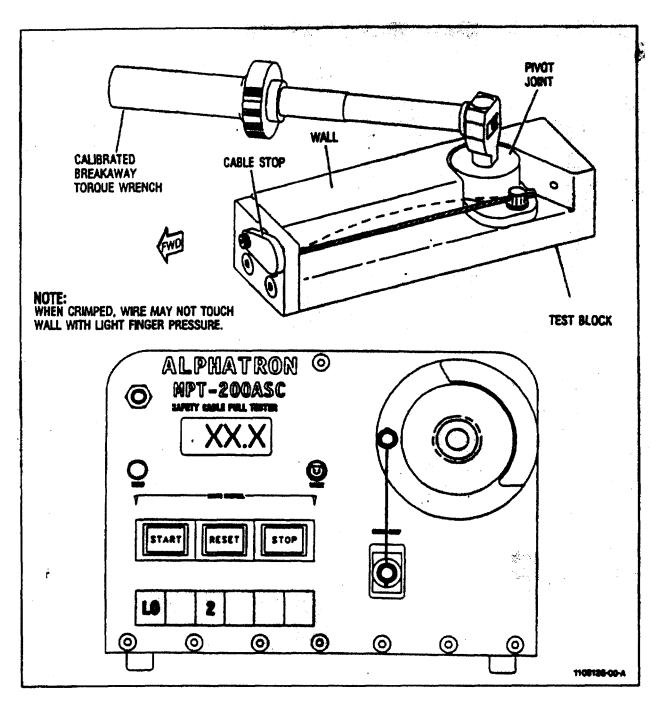
Figure 075-5-12. Crimping Tool Verification Equipment
