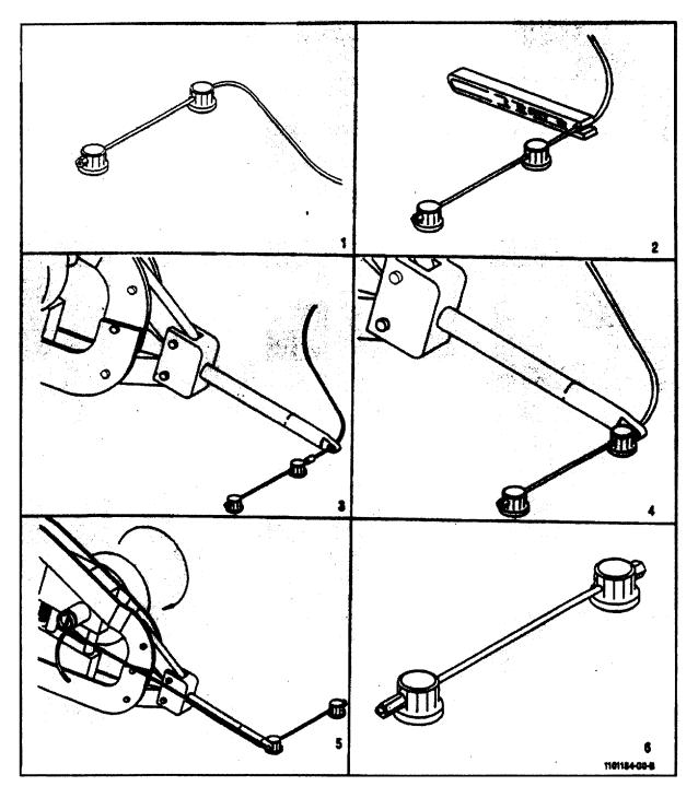
Figure 075-5-13. Safety Cable Procedure (Sheet 1 of 2)
