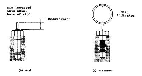
Figure 075-4-2. Measuring the Stretch.
