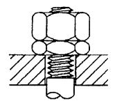
Figure 075-5-5. Jam Nut Assembly.
