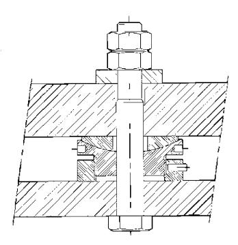
Figure 075-2-18 Vibracon Adjustable Chock Installed.
