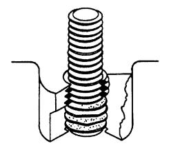
ASSEMBLED STUD-LOCK INSERT AND STUD
