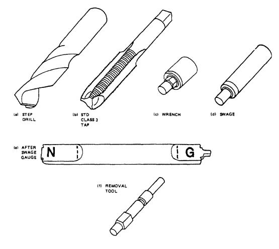
Figure 075-2-7. Typical Thin Wall Insert Repair Kit Tools
