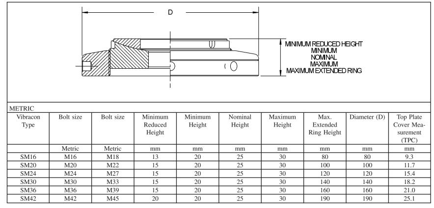
Table 075-2-32 Vibracon Adjustable Chock – Low Profile Configurations, Non-Shock Applications, METRIC
