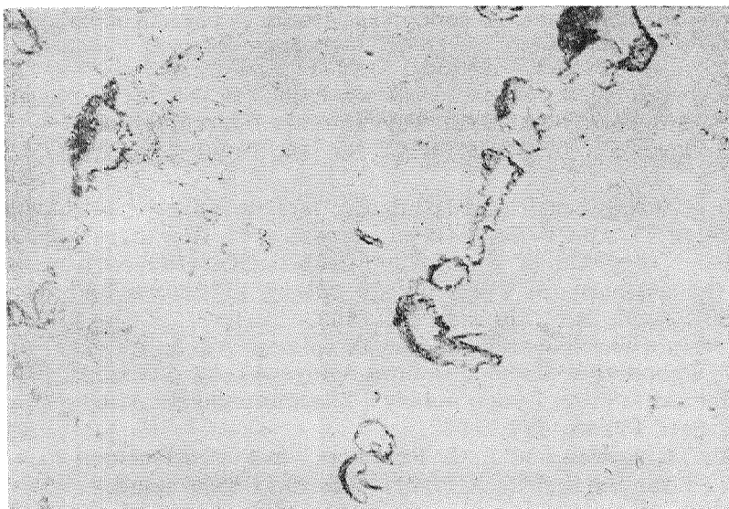
Figure 6. Microstructure of the Alloy AT-3 Following Creep Tests at T = 500^{\circ}\text{C} , \sigma = 15 \text{ kg/mm}^2 , \tau = 1500 \text{ hr} . Magnified 10,000 Times.
