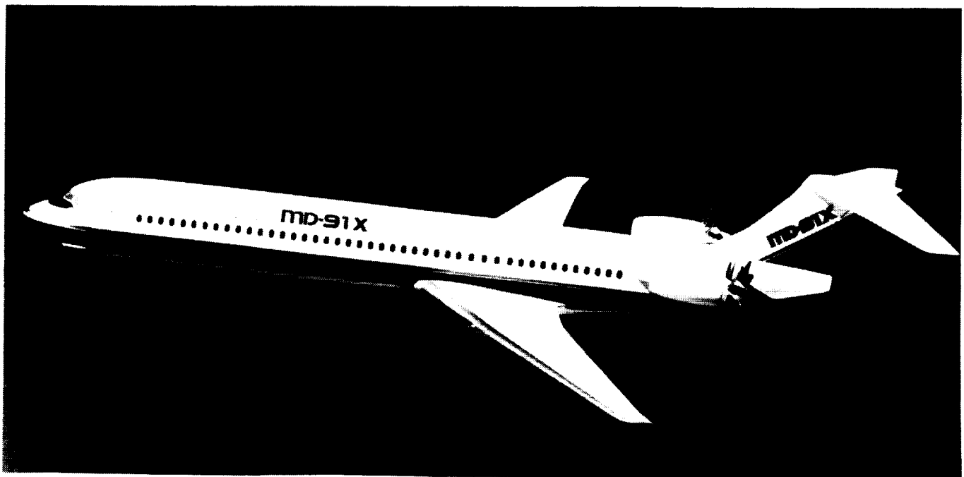
Figure 2. An aft-mounted, pusher, counter-rotating propeller configuration of an advanced turboprop aircraft.
