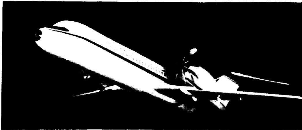
Figure 1. A wing-mounted, tractor, single-rotating propeller configuration of an advanced turboprop aircraft.
