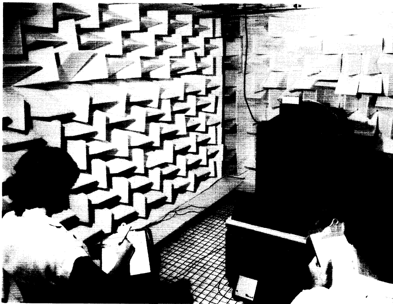
Figure 7. Subjects in the Anechoic Listening Room in the Langley Acoustics Research Laboratory.
