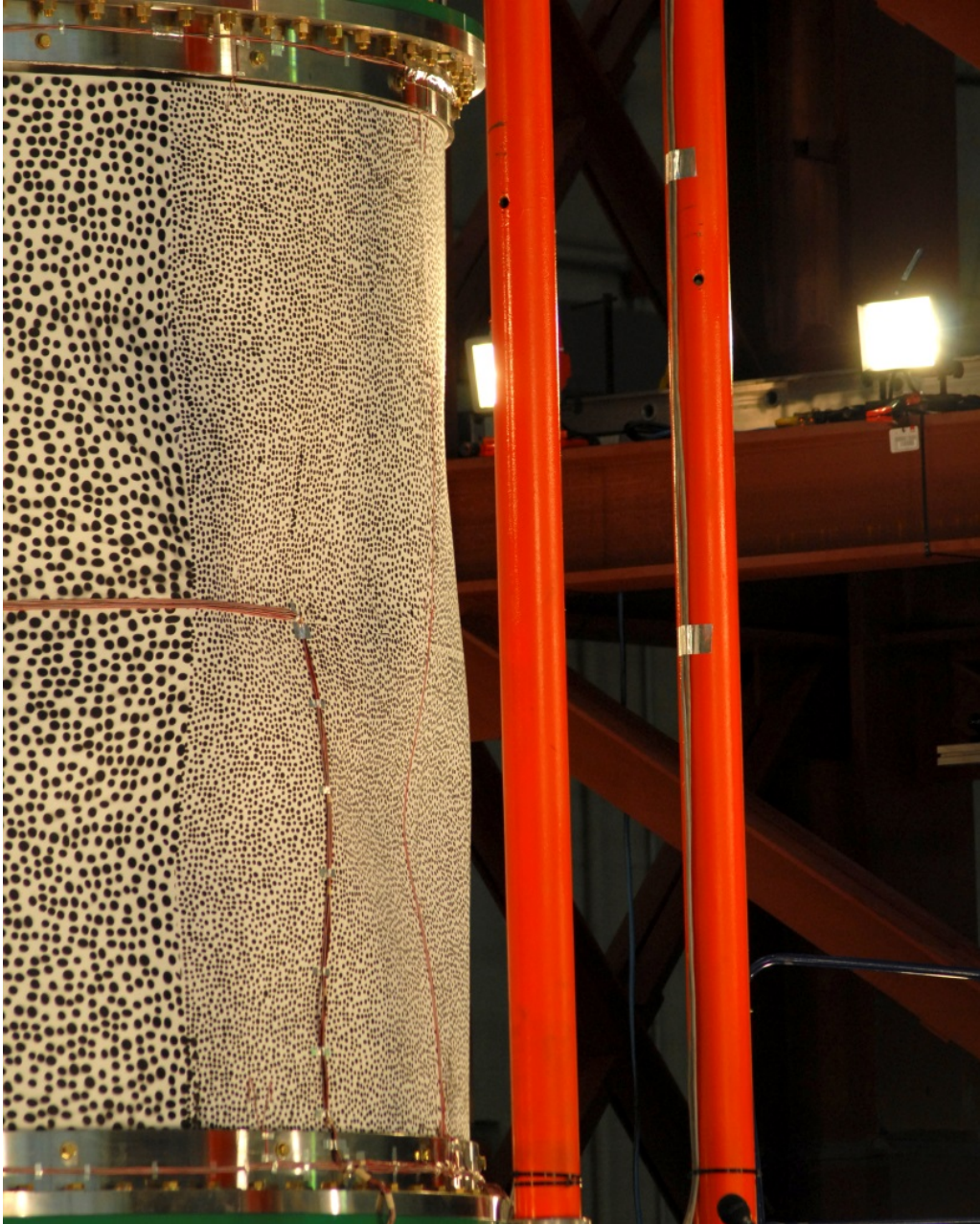
Figure 4.6. TA01 after global buckling.
