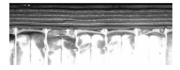
Figure 13. 2 ft-lb, 0.5-in-diameter impactor.
