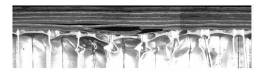
Figure 21. 8 ft-lb, 0.5 in-diameter impactor.
