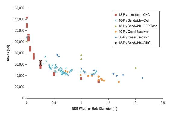
Figure 10. Comparison of all defect types.
