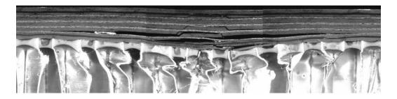
Figure 23. 10 ft-lb, 0.5 in-diameter impactor.
