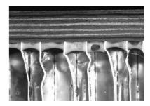
Figure 12. 1 ft-lb, 0.5-in-diameter impactor (no delamination).
