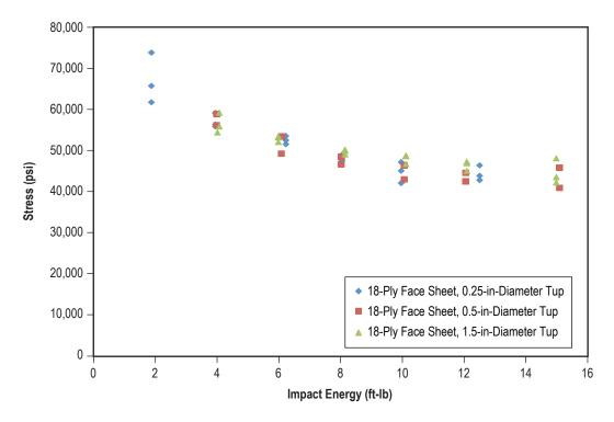
Figure 4. Residual compression strength versus impact energy.
