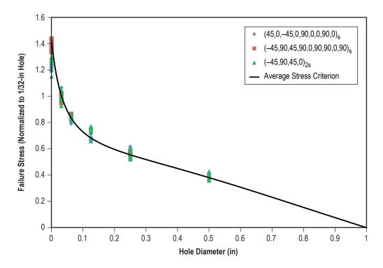
Figure 9. OHC normalized to 1/32-in-diameter hole.
