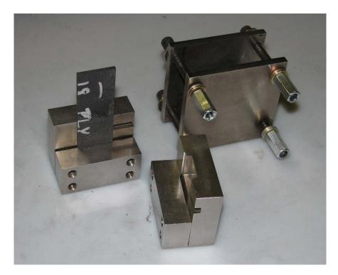
Figure 6. Northrop OHC fixture. 16
