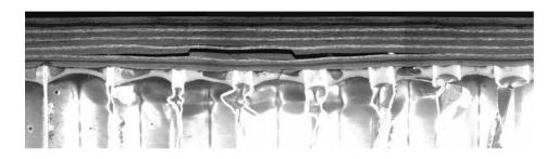
Figure 16. 3 ft-lb, 1.5-in-diameter impactor.
