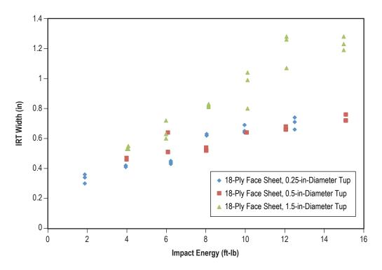
Figure 2. NDE indication width versus impact energy.
