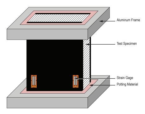
Figure 3. Sandwich edgewise compression.
