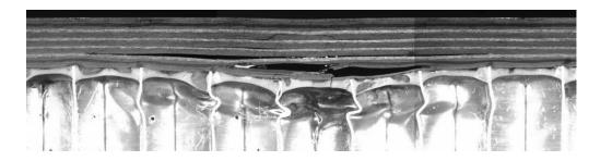
Figure 19. 6 ft-lb, 0.5-in-diameter impactor.
