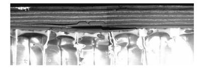
Figure 17. 4 ft-lb, 0.5-in-diameter impactor.
