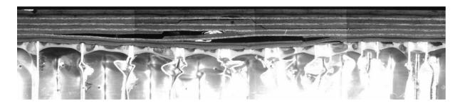
Figure 22. 8 ft-lb, 1.5 in-diameter impactor.
