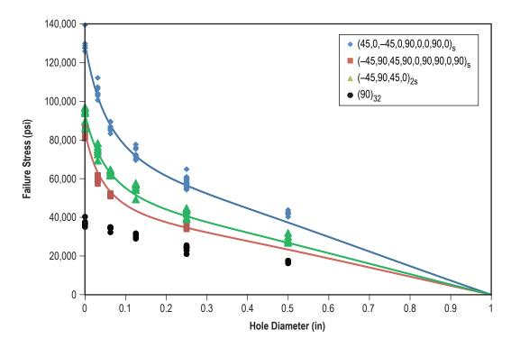
Figure 8. Laminate OHC results.
