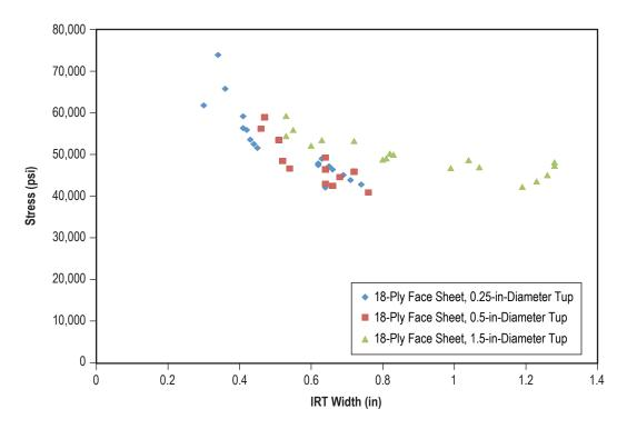
Figure 5. Residual compression strength versus NDE indication size.
