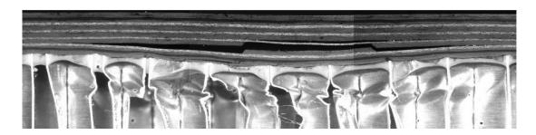
Figure 20. 6 ft-lb, 1.5-in-diameter impactor.
