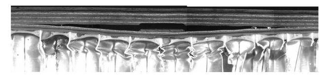
Figure 24. 10 ft-lb, 1.5-in-diameter impactor.
