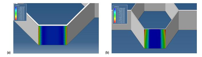
Figure 11. Finite element analysis model of residual thermally induced stresses in (a) 12 lb/ft<sup>3</sup> core and (b) 6.1 lb/ft<sup>3</sup> core.
