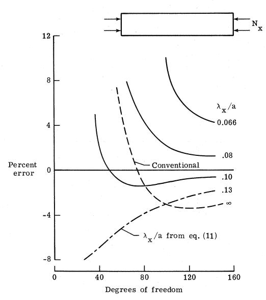
(d) Convergence for the compressive buckling of isotropic clamped  $5 \times 1$  panels.  $\lambda_y/\lambda_x = \beta = 1.5$ . From reference 16,  $\overline{N}_x \approx 7.0$ .
