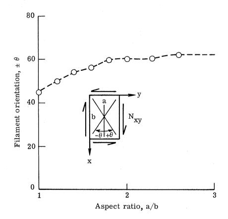
Figure 10.- Optimum filament orientation for the shear buckling of a simply supported panel.
