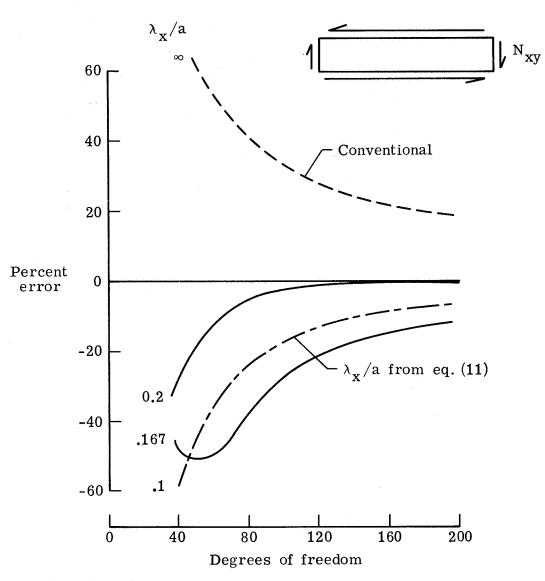
(f) Convergence for the shear buckling of isotropic clamped  $5 \times 1$  panels.  $\lambda_y/\lambda_x = \beta = 1.2$ . From reference 1,  $\overline{N}_{xy} \approx 9.3$ .
