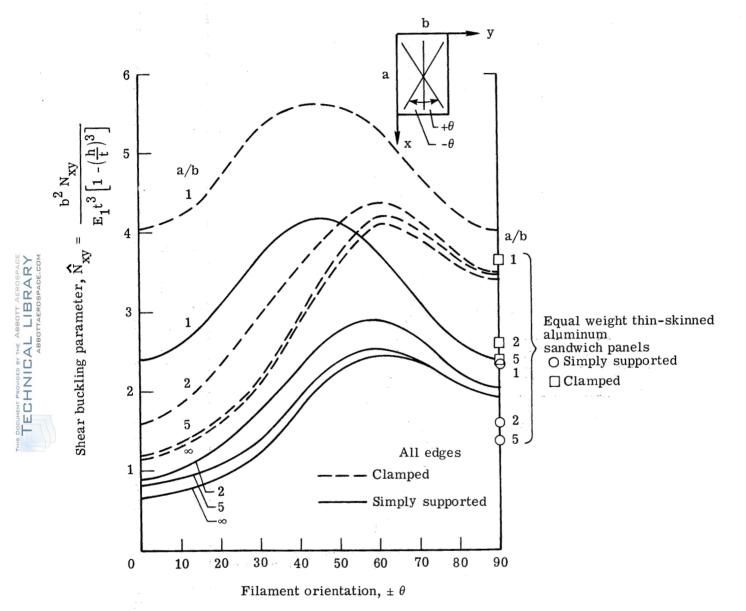
Figure 7.- Variation of shear buckling load with filament orientation for panels of various aspect ratios.
