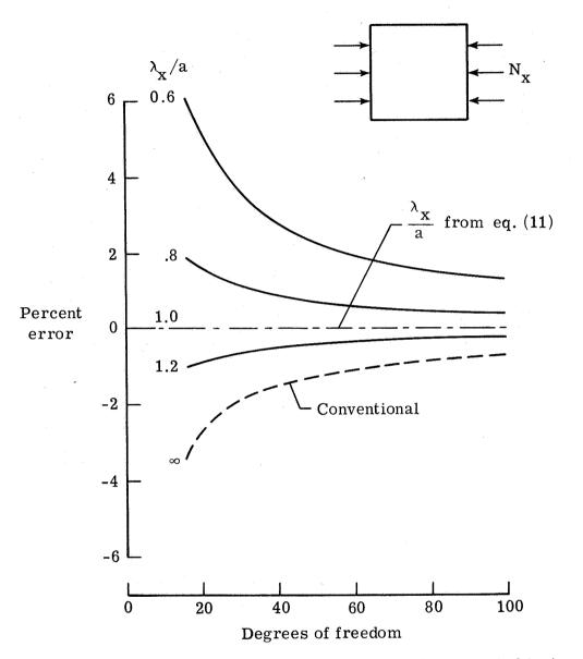
(a) Convergence for the compressive buckling of simply supported isotropic square panels.  $\lambda_y/\lambda_x = \beta = 1$ . From reference 6,  $\overline{N}_x = 4.0$ . Figure 17.- Convergence characteristics of trigonometric finite differences.
