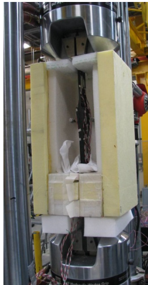
Figure 4. Test specimen encased in thermal insulation box.
