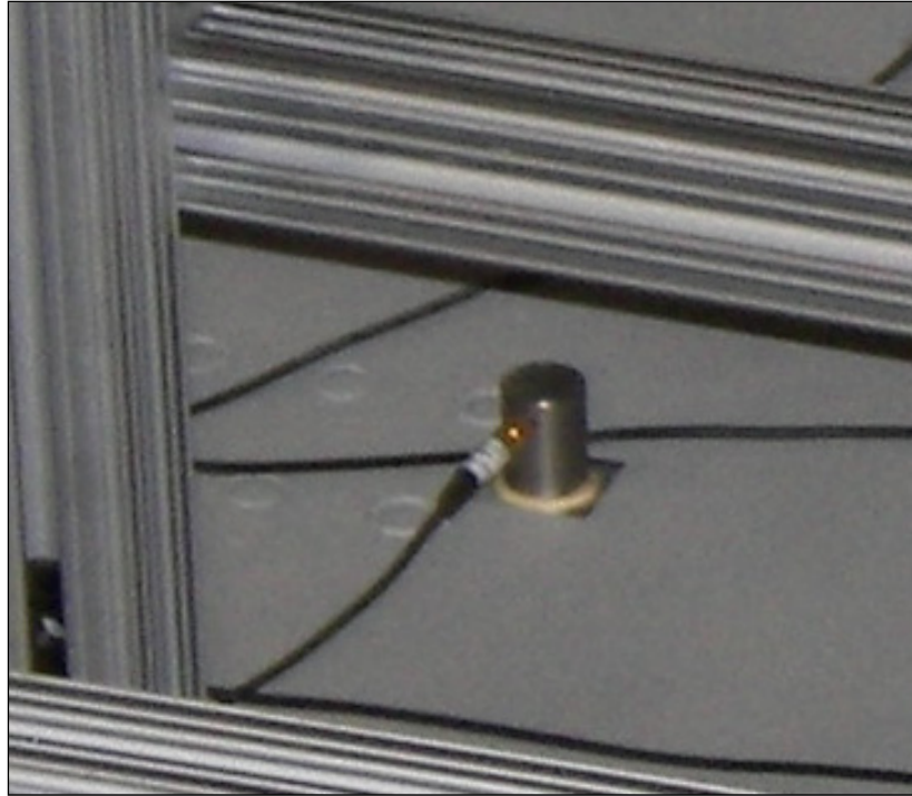
Figure 4. Installation of one AE sensor on the crown panel
