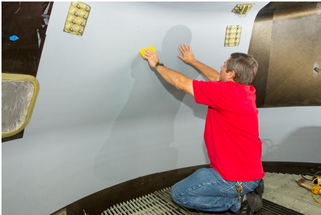
Figure 7.3-15. Technician Finalizes 3M ™ 5004 Film Application
