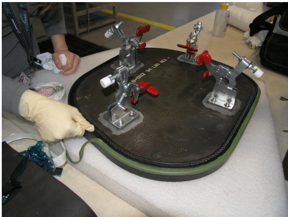
Figure 7.3-2. Vacuum Sealant Tape (i.e., vacuum putty) Installed on a CCM Hatch Cover on the Outside Flange Next to the O-ring
