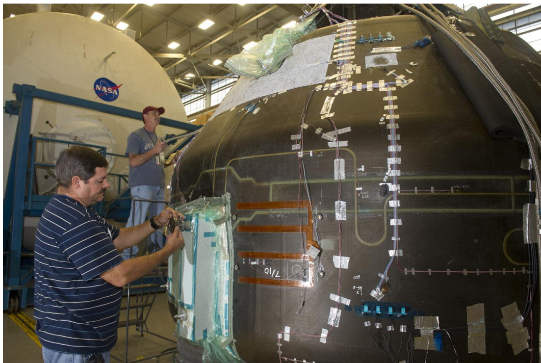
Figure 7.3-8. Vacuum Bag Installation around an SM/ALAS Fitting
