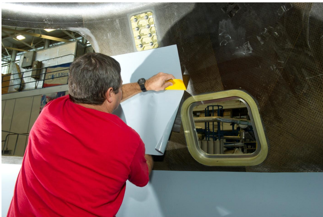
Figure 7.3-14. Technician Uses a Plastic Tool to Help Avoid Wrinkles and Bubbles
