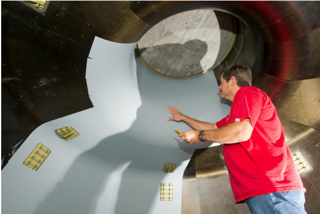
Figure 7.3-17. 3M™ 5004 Film Inspection in Docking Tunnel
