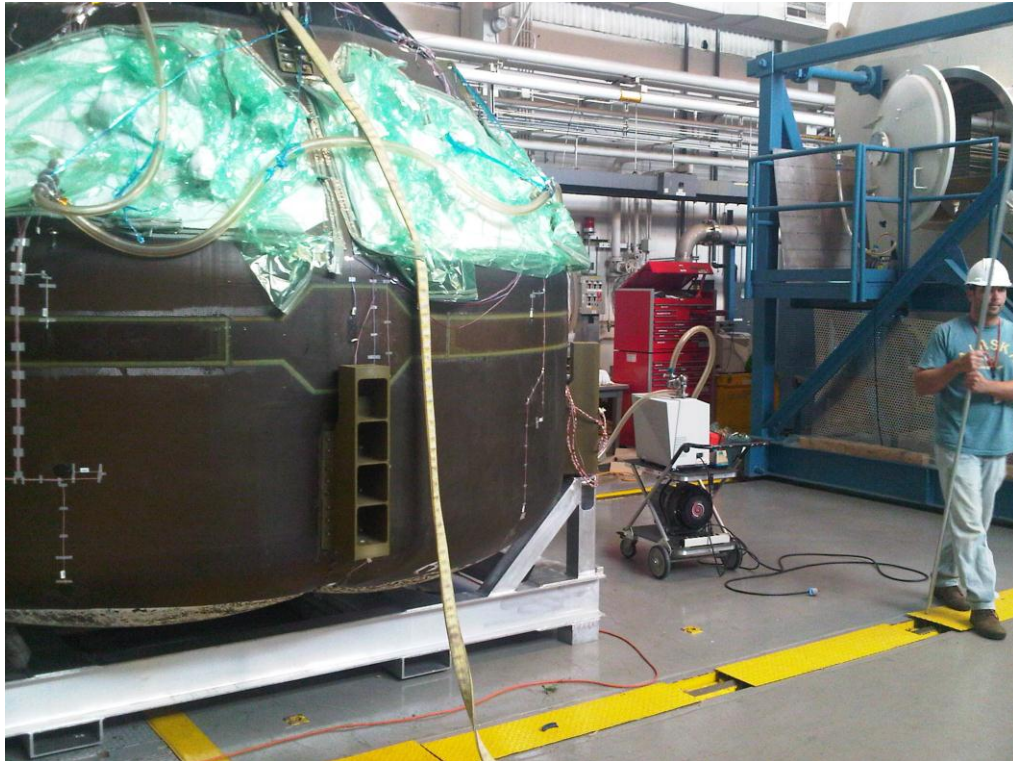
Figure 7.3-9. Installed Hatch Vacuum Bags Attached to a Mass Spectrometer
