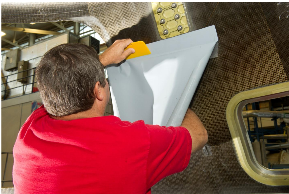
Figure 7.3-13. Technician Starts to Apply the 3M™ 5004 Film around CCM IML Features
