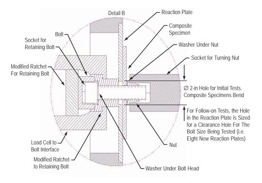
Figure 6. Details of specific test components.
