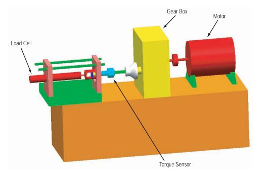
Figure 2. Torque versus tension machine configuration.
