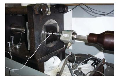
Figure 1. Torque versus tension test.
