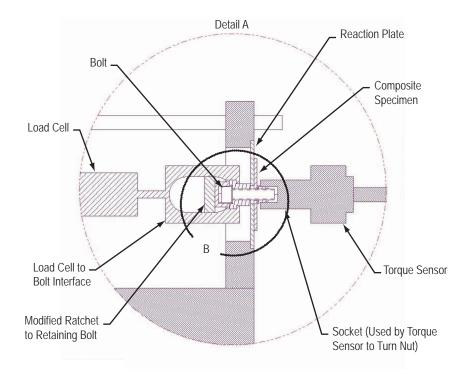
Figure 5. Detailed view of test setup.
