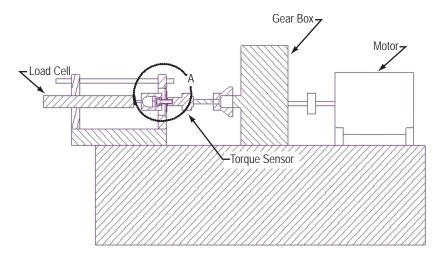
Figure 4. Torque versus tension cross section.
