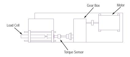
Figure 3. Top view of torque versus tension machine.
