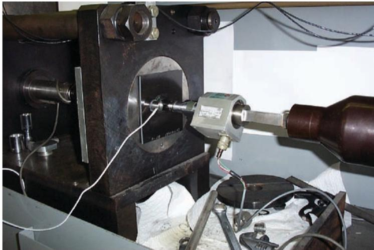
Figure 1. Torque versus tension test.
