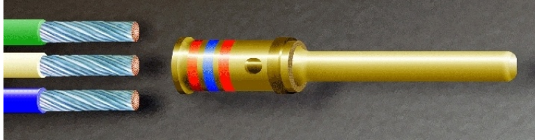
Figure 19-20. Stripped Wires Prior to Insertion
