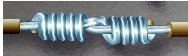
Figure 19-16. Completed Wrap for Western Union/Lineman Splice
