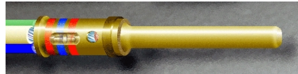
Figure 19-22. Wires Crimped Within Contact
