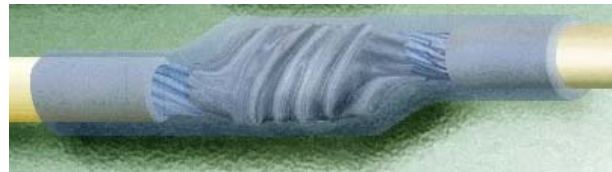
Figure 19-11. Sleeved Lash Splice
